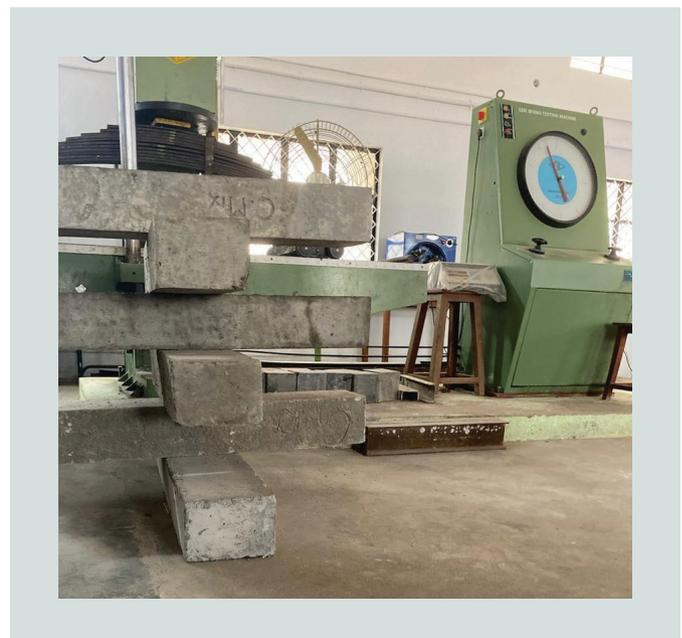
**Figure 3.** Reinforced concrete beam samples.
