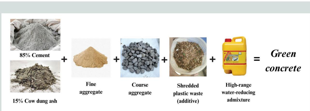
**Figure 2.** Components of optimized sustainable concrete mixture proportions.
