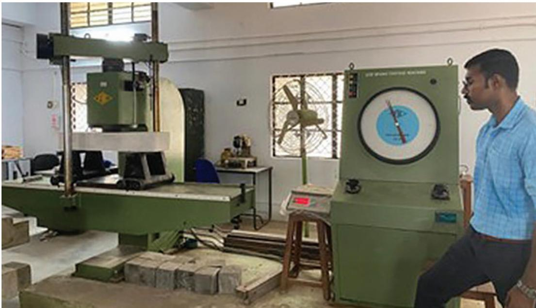
Figure 4. Load setup for testing of concrete beam specimen.
