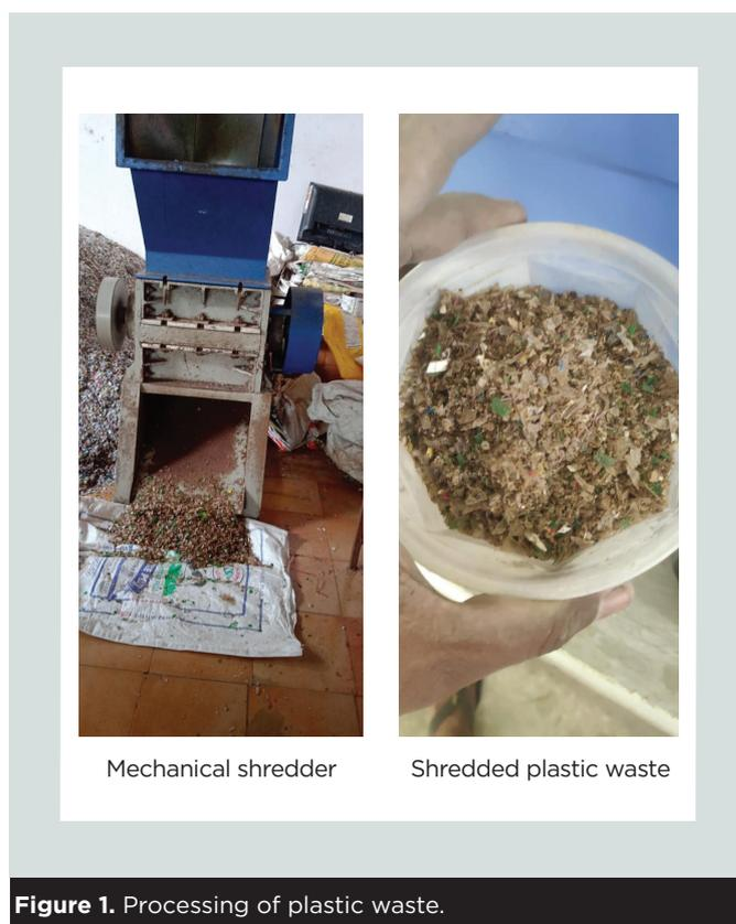
**Figure 1.** Processing of plastic waste.
