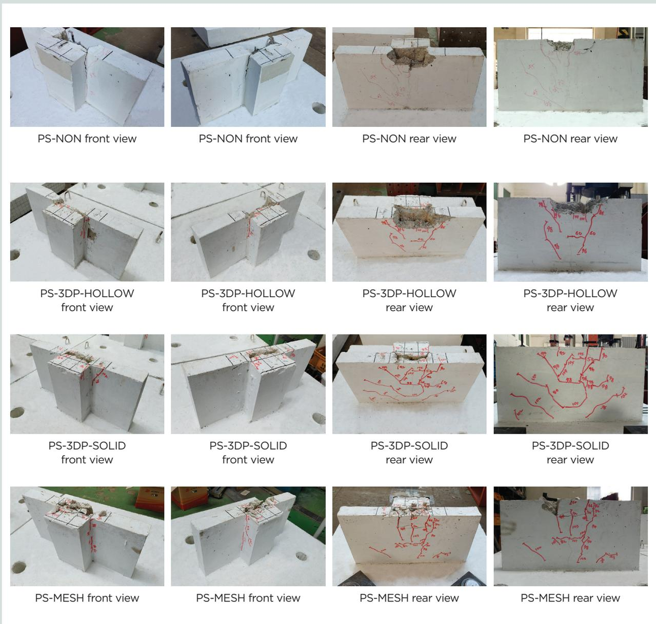
**Figure 9.** Crack patterns of each strand pullout experiment specimen. Note: PS-MESH = specimen with reentrant corners reinforced using metal lath; PS-NON = specimen with no reentrant corner crack reinforcing elements; PS-3DP-HOLLOW = specimen with hollow reinforcing elements manufactured by three-dimensional printing; PS-3DP-SOLID = specimen with solid reinforcing elements manufactured by three-dimensional printing.
