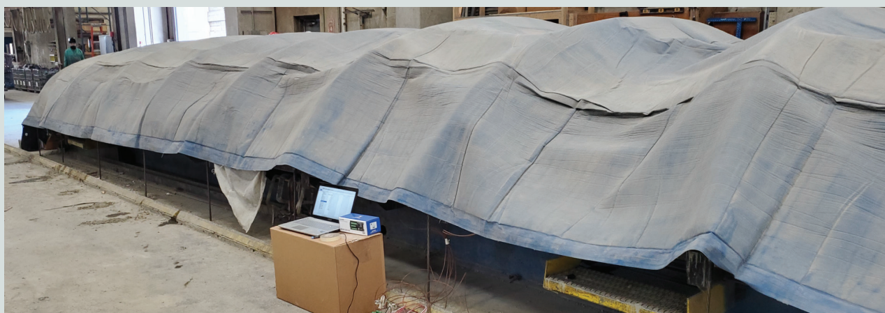
Figure 2. Beam curing setup with a heated bed and insulated blanket covering the specimens.
