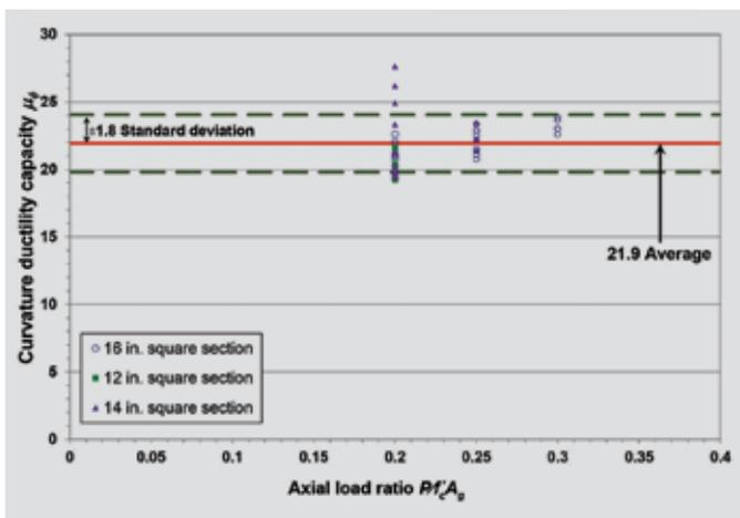
**Figure 8.** Curvature ductility capacities of different square pile sections with confinement based on Eq. (12). Note:  $A_g$  = gross section area of the concrete pile section;  $f'_c$  = compressive strength of unconfined concrete;  $P$  = design axial force (derived from overstrength consideration). 1 in. =25.4 mm.
