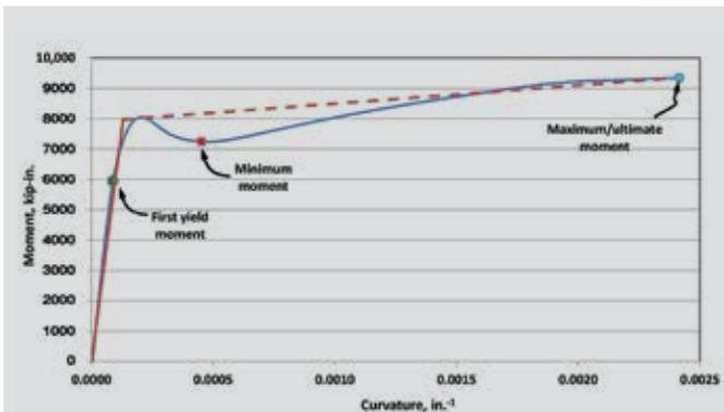
**Figure 4.** Moment-curvature idealization of a 24 in. octagonal prestressed concrete pile section. Note: 1 in. = 25.4 mm; 1 kip = 4.448 kN.
