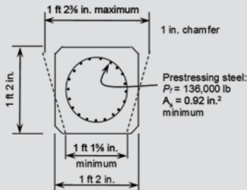
14 in. precast, prestressed concrete square cross section
