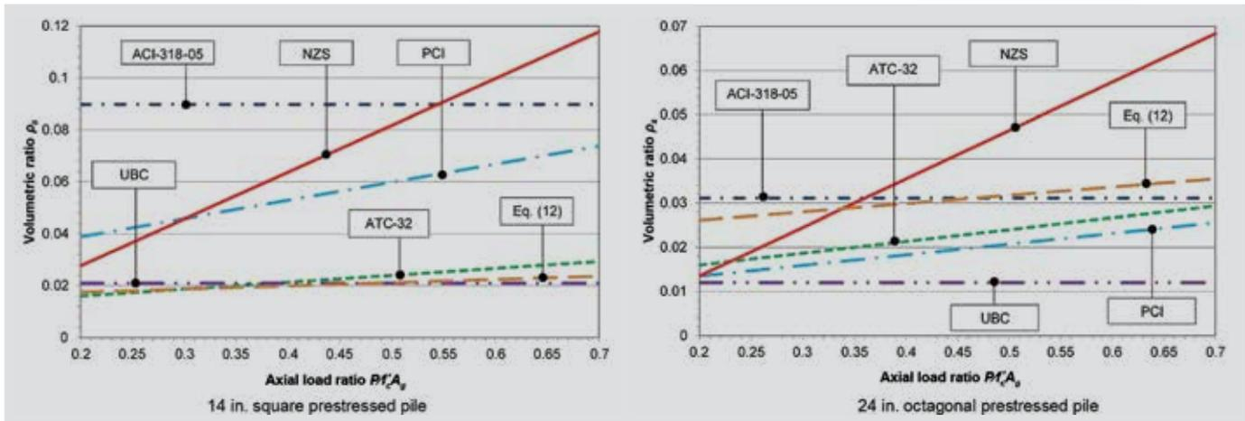
**Figure 6.** Comparison of required volumetric ratios of spiral reinforcement. Note:  $A_g$  = gross section area of the concrete pile section;  $f'_c$  = compressive strength of unconfined concrete;  $P$  = design axial force (derived from overstrength consideration). 1 in. =25.4 mm.
