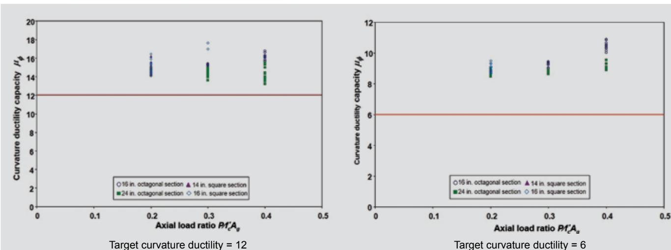
**Figure 9.** Curvature ductility capacities of octagonal piles designed with small target ductility. Note:  $A_g$  = gross section area of the concrete pile section;  $f'_c$  = compressive strength of unconfined concrete;  $P$  = design axial force (derived from overstrength consideration). 1 in. =25.4 mm.
