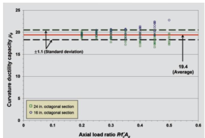
**Figure 7.** Curvature ductility capacities of 16 and 24 in. prestressed pile sections with confinement reinforcement based on Eq. (12). Note:  $A_g$  = gross section area of the concrete pile section;  $f'_c$  = compressive strength of unconfined concrete;  $P$  = design axial force (derived from overstrength consideration). 1 in. =25.4 mm.
