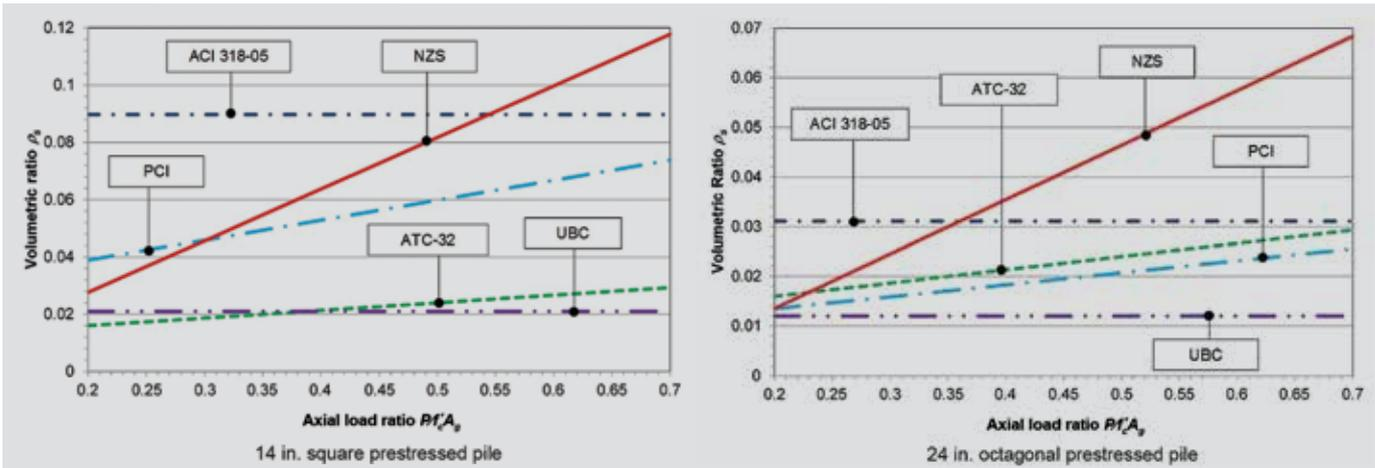
**Figure 2.** Confinement reinforcement per different design requirements as a function of axial load ratio. Note:  $A_g$  = gross section area of the concrete pile section;  $f'_c$  = compressive strength of unconfined concrete;  $P$  = design axial force (derived from overstrength consideration). 1 in. = 25.4 mm.
