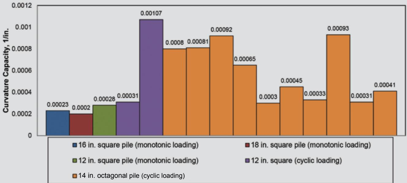
Curvature capacities reported for precast, prestressed concrete piles
