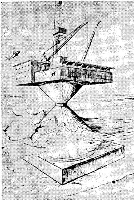
Fig. 5. Proposed deep-water drilling structure of prestressed concrete for Arctic Ocean
