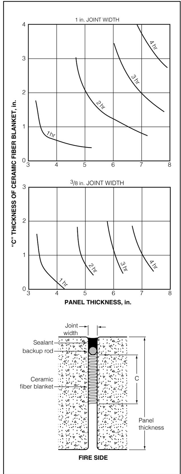
Figure 2. Fire resistance of precast concrete wall joints.
