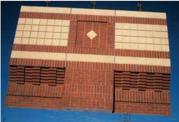
**Figure 1** Bonding patterns incorporated into the finished panel.
