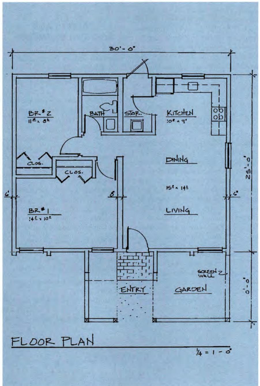
Fig. 10D. Floor plan of small residence designed with a single panel comprising each of the four basic exterior walls.
