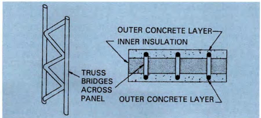
Fig. 10C. Cross section of laminated panel.
