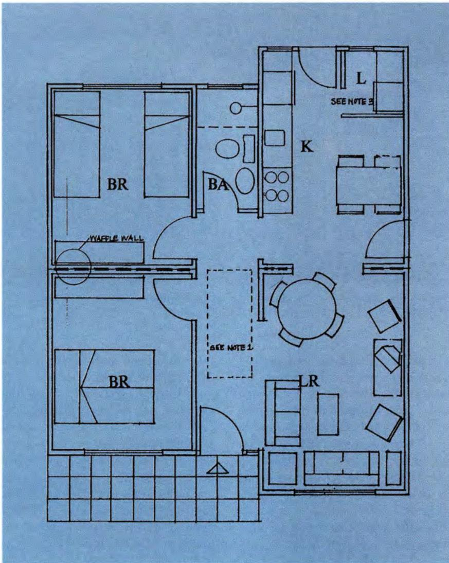
Fig. 8A. Floor plan of 512 sq ft (48 m<sup>2</sup>) house made with two sizes of room modules. Door-size window in the kitchen permits future expansion.
