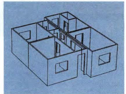
Fig. 8B. Cutaway view of assembled modules shows how extensions cast with the boxes permit enclosing a portion of the central corridor to create a bathroom.
