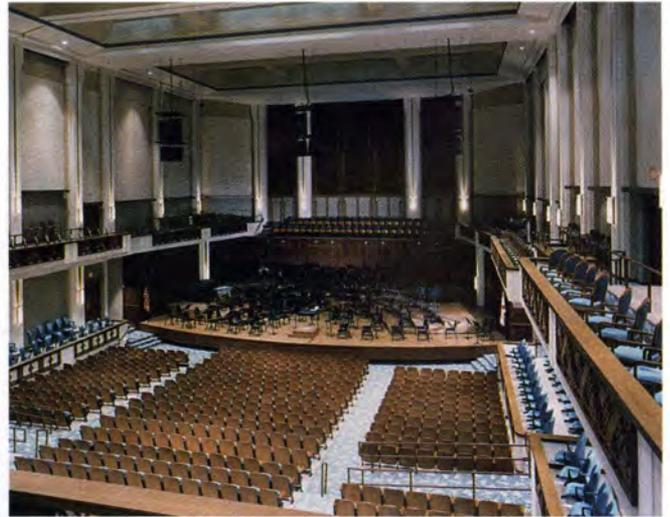
Fig. 4. Designing the precast wall panels that provide the loadbearing and acoustical needs for the Jacoby Hall was complicated by the step-down format that places the stage at the lowest point. The wide panels featured a similar step-down style that had zero tolerance for erection.
