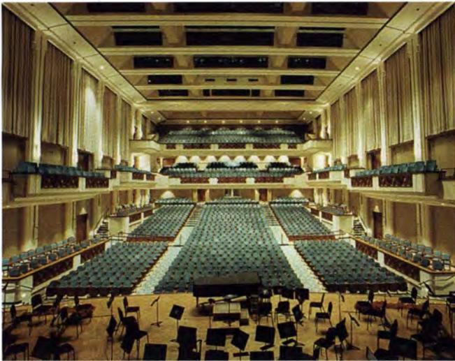
Fig. 3. The new Jacoby Symphony Hall features precast concrete walls that provide a curved and completely smooth interior surface that offers excellent acoustics. Only a low-powered public address system is used for lectures, with no enhancements needed for performances.
