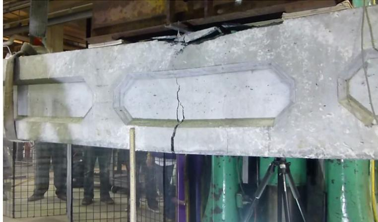
***Figure 9. Beam at Failure***
