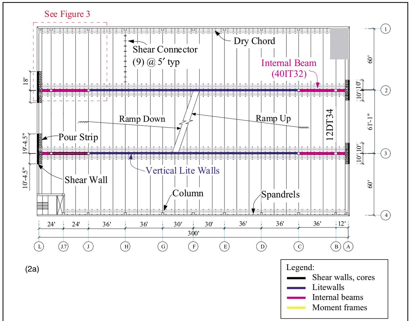
Fig. 2. Prototype structures (2a): Plan of PS#1: Side-by-side parking structure, four stories. Note: 1 ft = 0.308 m; 1 in. = 25.4 mm.
