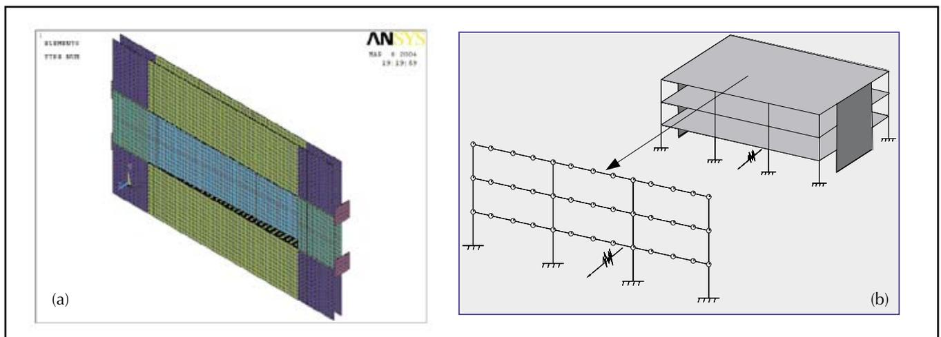
Fig. 11. Structure models: (a) Three-dimensional FE model; (b) UCSD MDOF model.
