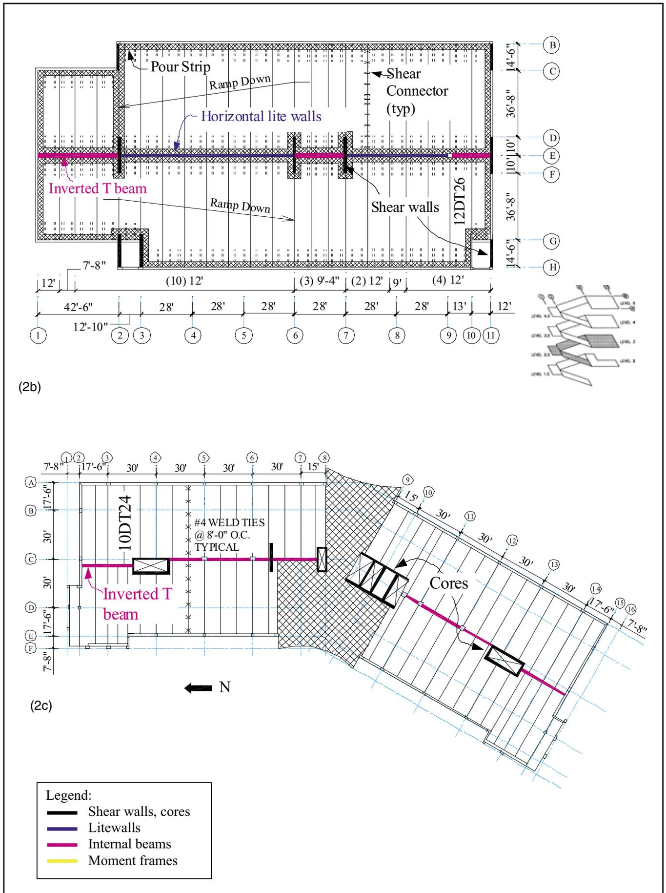
Fig. 2 (cont.). Prototype structures (2b): Plan of PS#2: Helical parking structure, four stories; (2c): Plan of PS#3: Distributed core L-wing office building, five stories. Note: 1 ft = 0.308 m; 1 in. = 25.4 mm.
