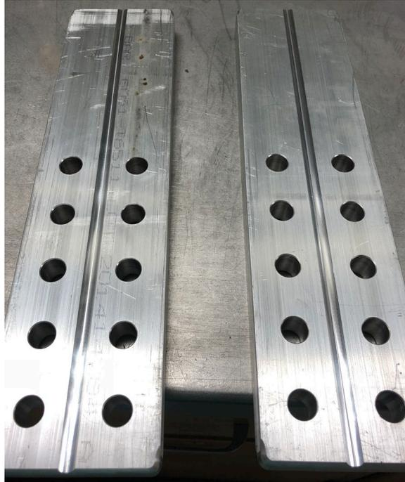
Figure 3 – Example of smooth cylindrical grips
