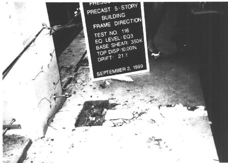
Figure. A.15 – Floor damage (EQ-III level)
