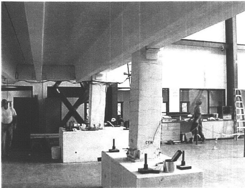
Figure A.18 – Gravity column and first floor slab (End of Test)
