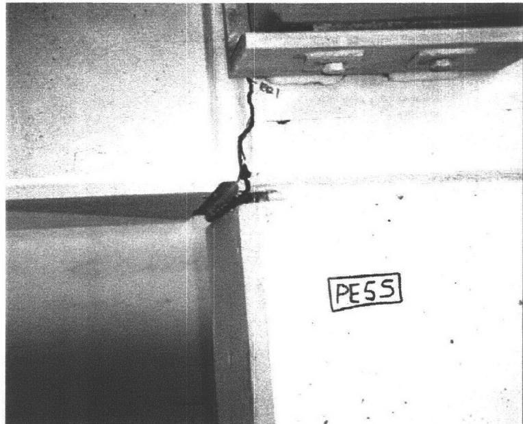
Figure. A.4 – Pretensioned connections EQ2 Excitation (average drift 1.7 % )
