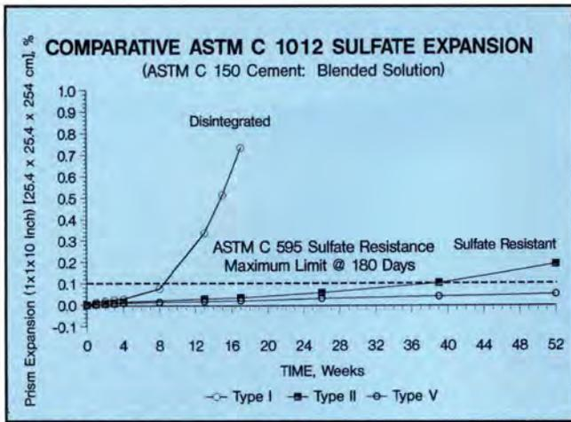
Fig. K. Comparative ASTM C 1012 sulfate expansion (ASTM C 150 cement: blended solution).
