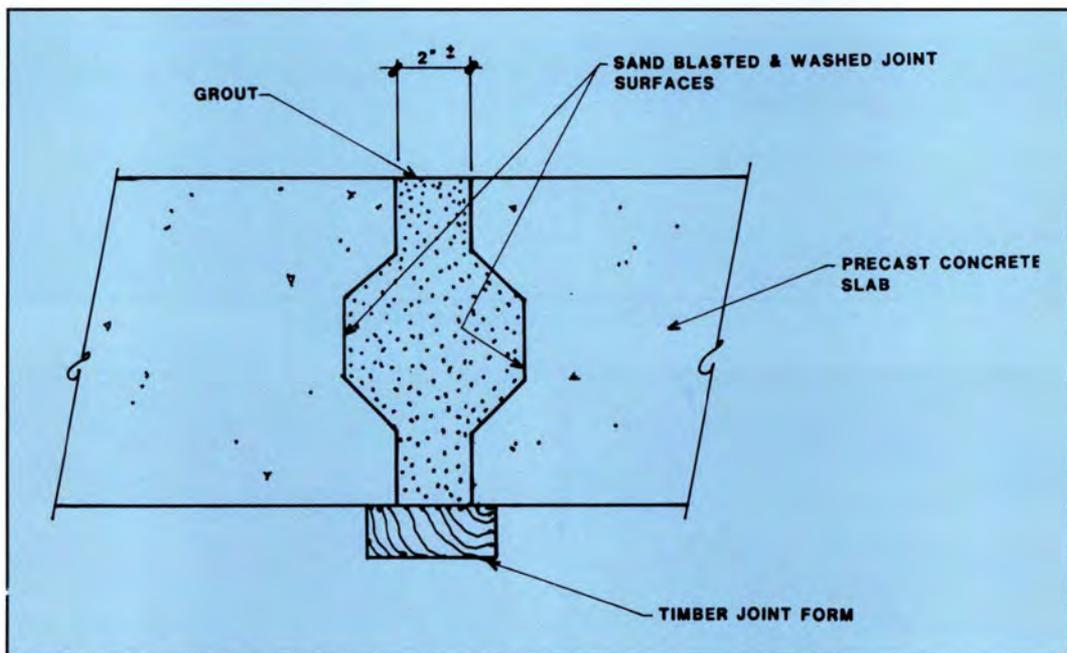
Fig. C. Typical Peratrovich, Nottingham & Drage, Inc. grouted panel shear key.
