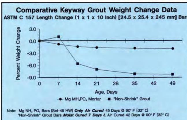
Fig. I. Comparative keyway grout weight change data [ASTM C 157 length change 1 x 1 x 10 in. (24.5 x 24.5 x 254 mm) bars].
