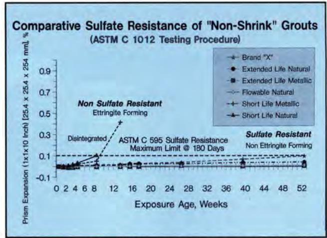
Fig. L. Comparative sulfate resistance of non-shrink grouts (ASTM C 1012 testing procedure).
