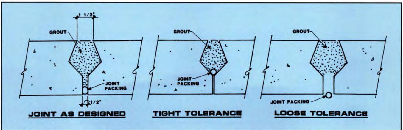
Fig. B. Typical examples of grouted shear keys.
