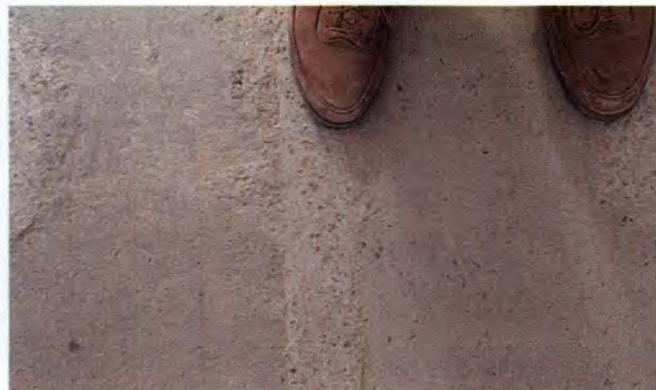
Fig. F. Set 45 extended magnesium ammonium phosphate grout joint.
