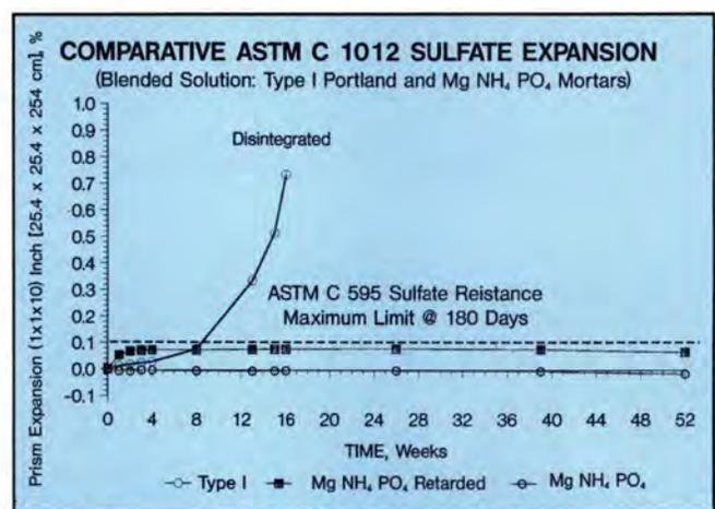
Fig. M. Comparative ASTM C 1012 sulfate expansion (blended solution: Type I portland and  $MgNH_4PO_4$  mortars).
