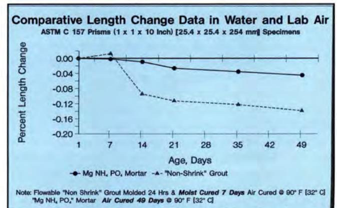
Fig. J. Comparative length change data in water and laboratory air [ASTM C 157 prisms 1 x 1 x 10 in. (25.4 x 25.4 x 254 mm) specimens].
