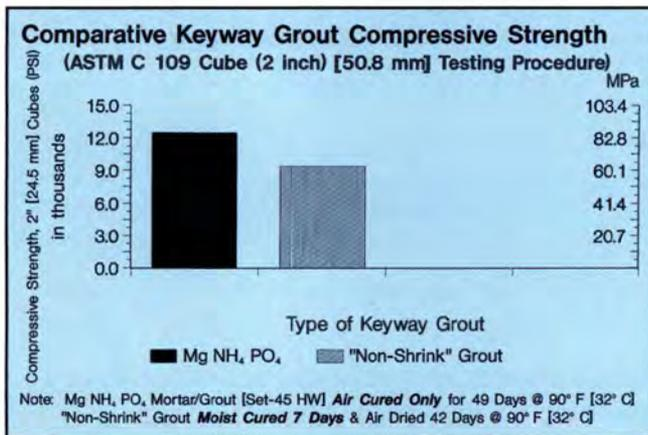
Fig. G. Comparative keyway grout compressive strength [ASTM C 109 cube 2 in. (50.8 mm) testing procedure].
