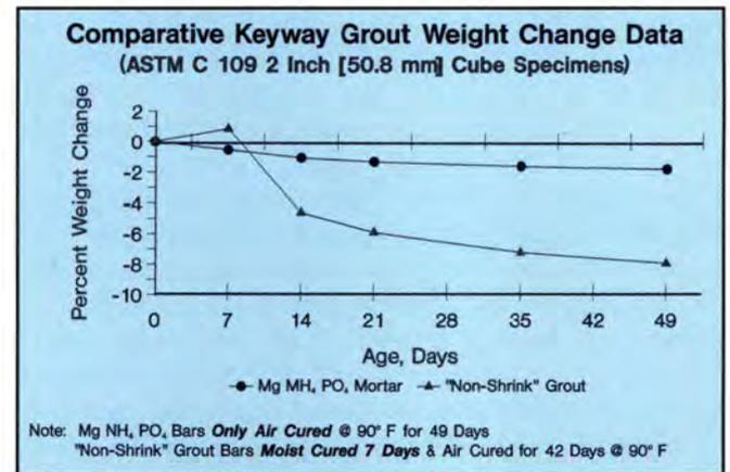
Fig. H. Comparative keyway grout weight change data [ASTM C 109 2 in. (50.8 mm) cube specimens].
