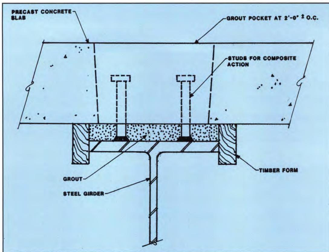
Fig. D. Typical Peratrovich, Nottingham & Drage, Inc. grouted girder haunch.
