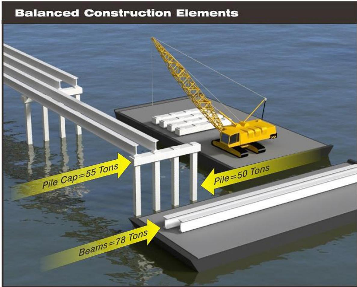
**Figure 7 – Precast Element Weights**
