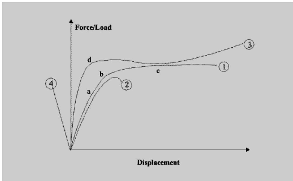
**Figure 4 - Different Types of Load Displacement Response**
