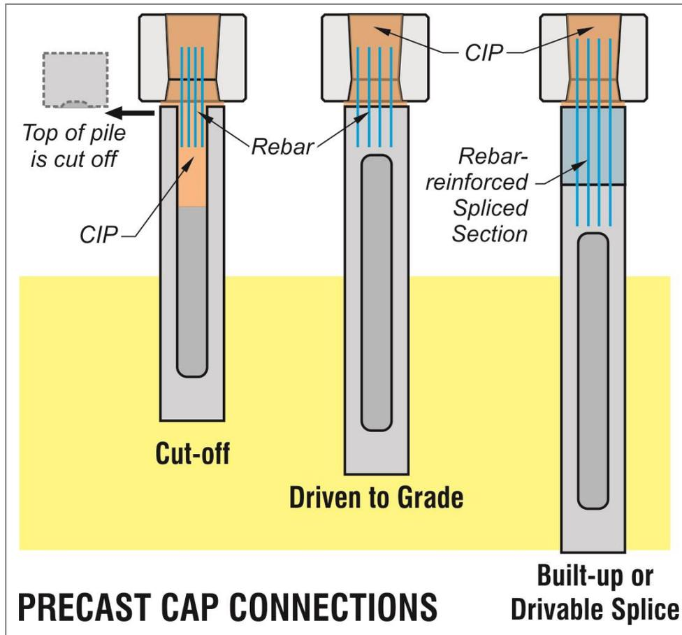
**Figure 8 – Bent Cap Connection Options**
