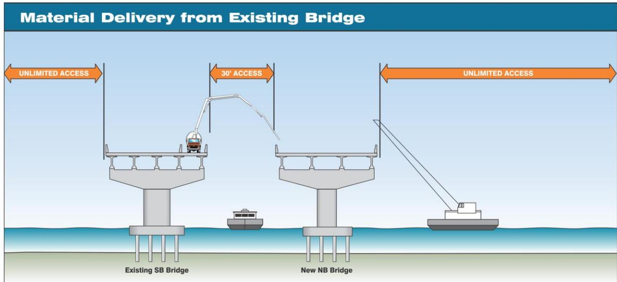
**Figure 2 – Material Delivery from Existing Bridge**
