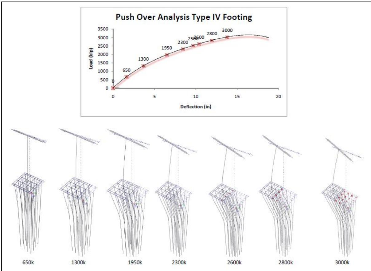
**Figure 5 - Load Displacement Response for Pier Type IV**
