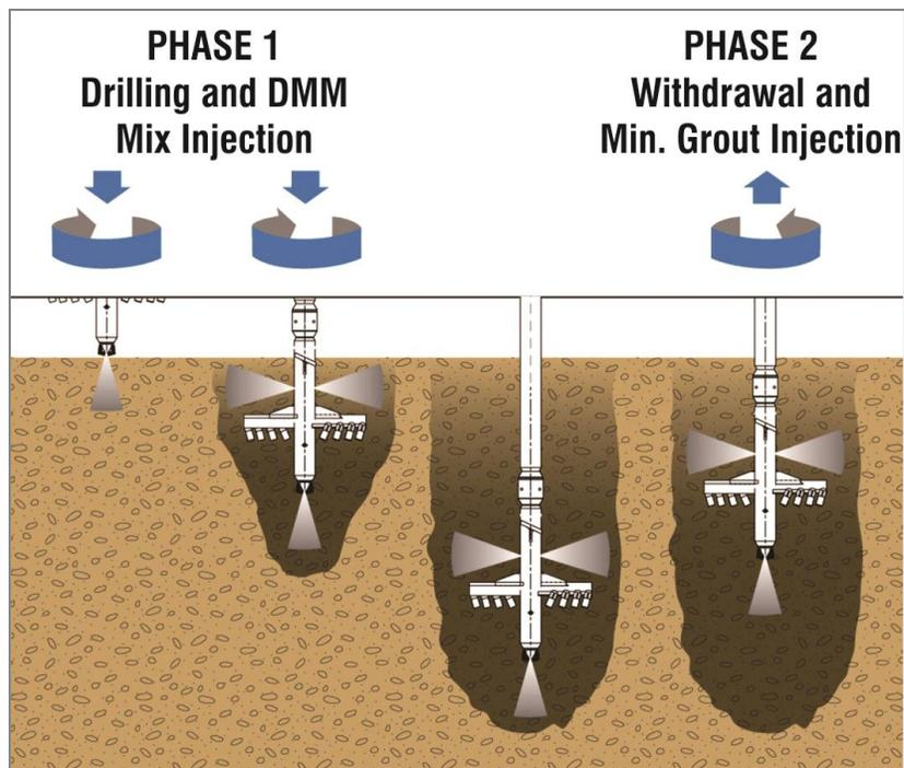
**Figure 15 – TTM Soil Mixing Method**
