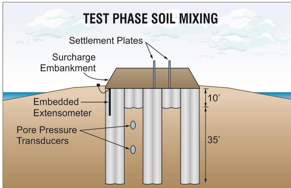
**Figure 16 – Embankment Test Instrumentation**
