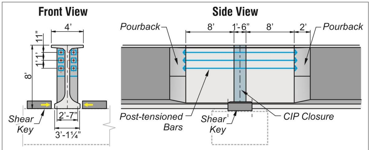
**Figure 6 – Post-Tensioned Connection Detail**
