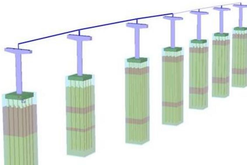
**Figure 3 – Seven Pier FEM Model from FB Multi-Pier**
