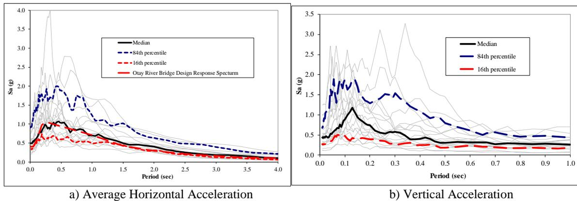
**Figure 11. Earthquake Response Spectra**
