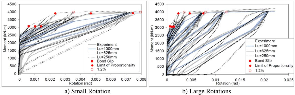
**Figure 4. Sensitivity of joint model response to the unbonded length,  $L_u$ , of PT tendons.<sup>3</sup>**
