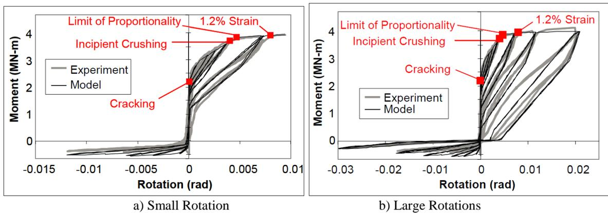
Figure 3. Comparison of 2D joint model with large scale experimental results.<sup>3</sup>
