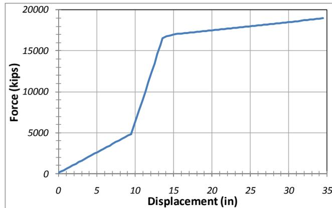
**Figure 14. Longitudinal Push-Over Response of the 3D Model**
