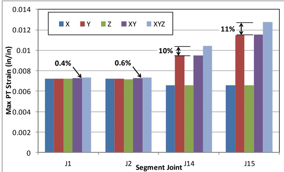
**Figure 16. Median Value of the Maximum PT Strain**
