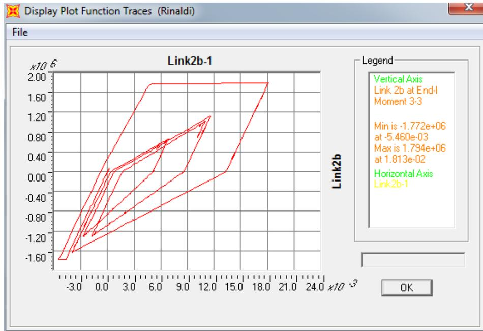
**Figure 13. Moment-Rotation Response of the NLINK element at the Base of Pier 2**
