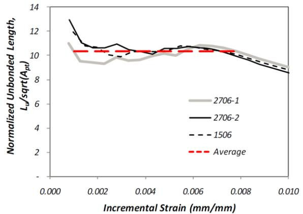
b) Normalized Unbonded Length vs Incremental Strain
