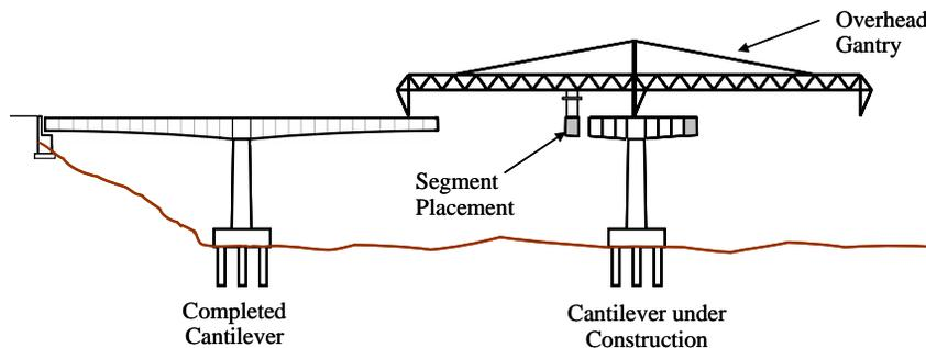
**Figure 1. Schematic of Balanced Cantilever Construction with Precast Segments and an Overhead Gantry**
