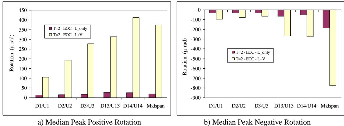
**Figure 6. The bar graphs show the influence of vertical ground motion on the segment joint rotations.<sup>5</sup>**
