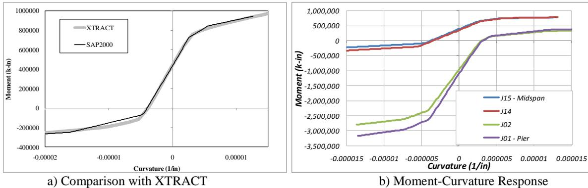
Figure 8. SAP2000 Segment Joint Model
