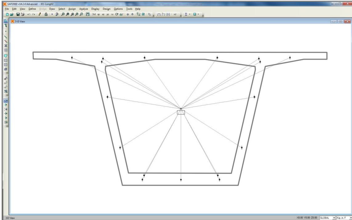
Figure 7. Screen shot of a 3D segment joint model with the cross section outlined
