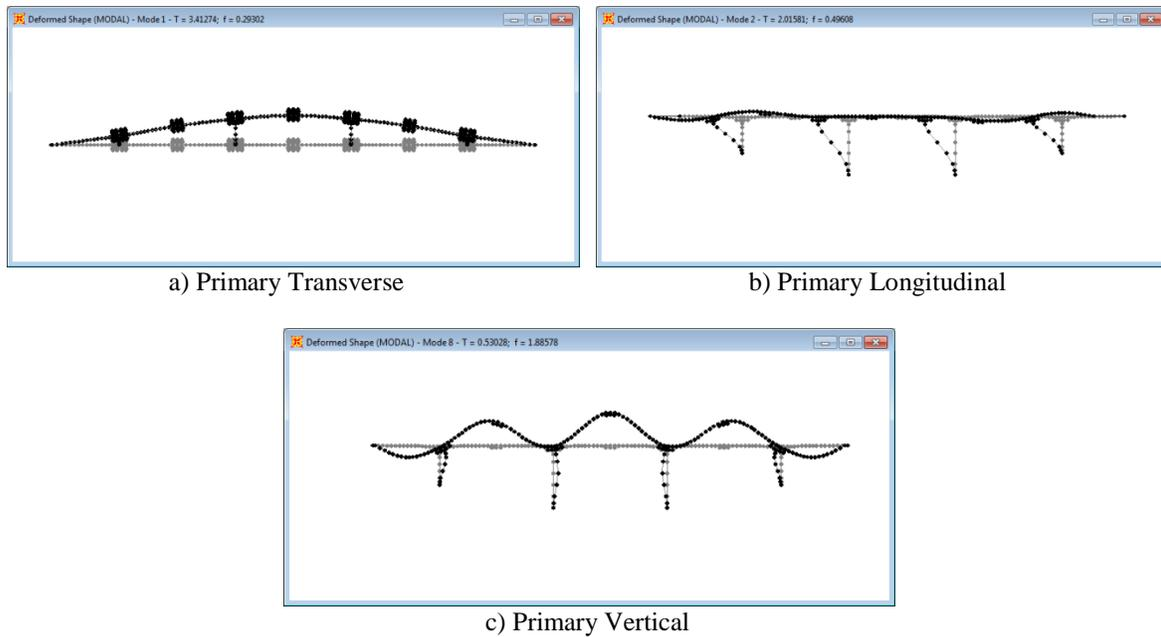
**Figure 12. Primary Mode Shapes from the 3D Model**
