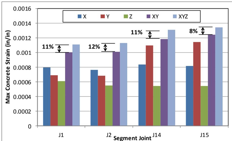
**Figure 17. Median Value of the Maximum Concrete Strain**
