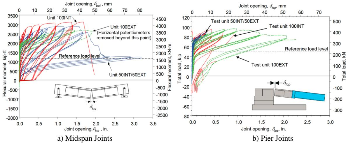
Figure 2. Segment Joint Response from Large Scale Experiments<sup>2</sup>
