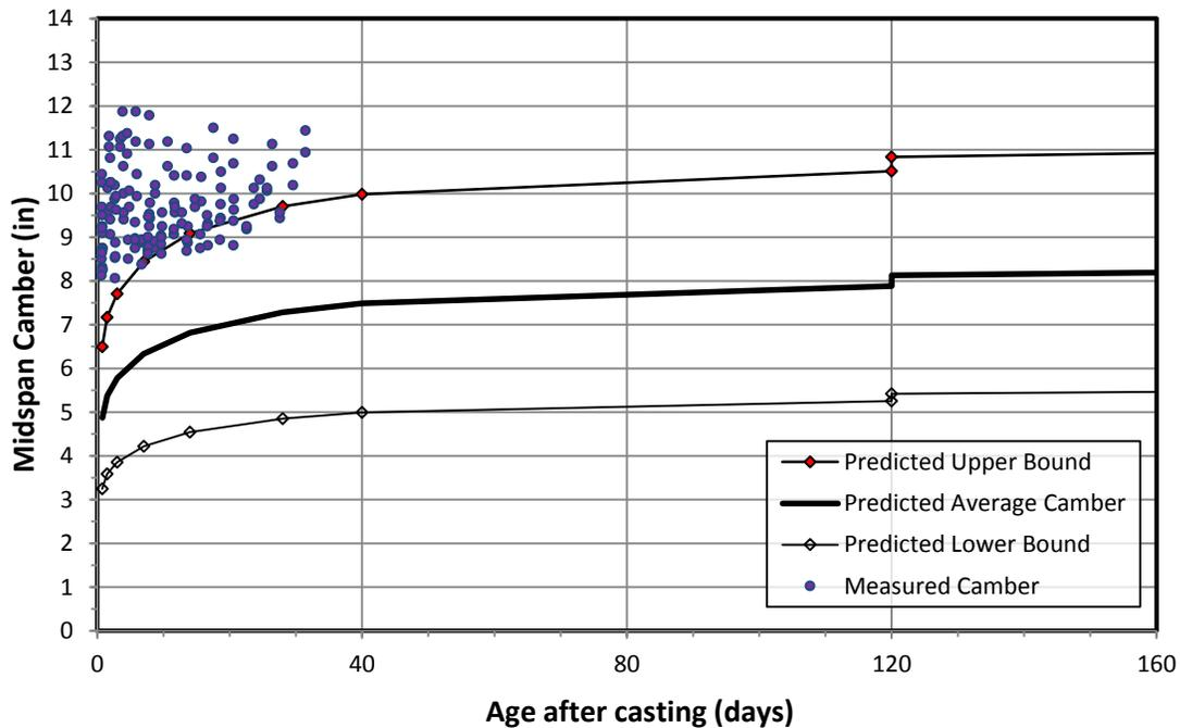
Fig. 16 Measured camber versus age after casting, Skagit River Bridge DBTs
