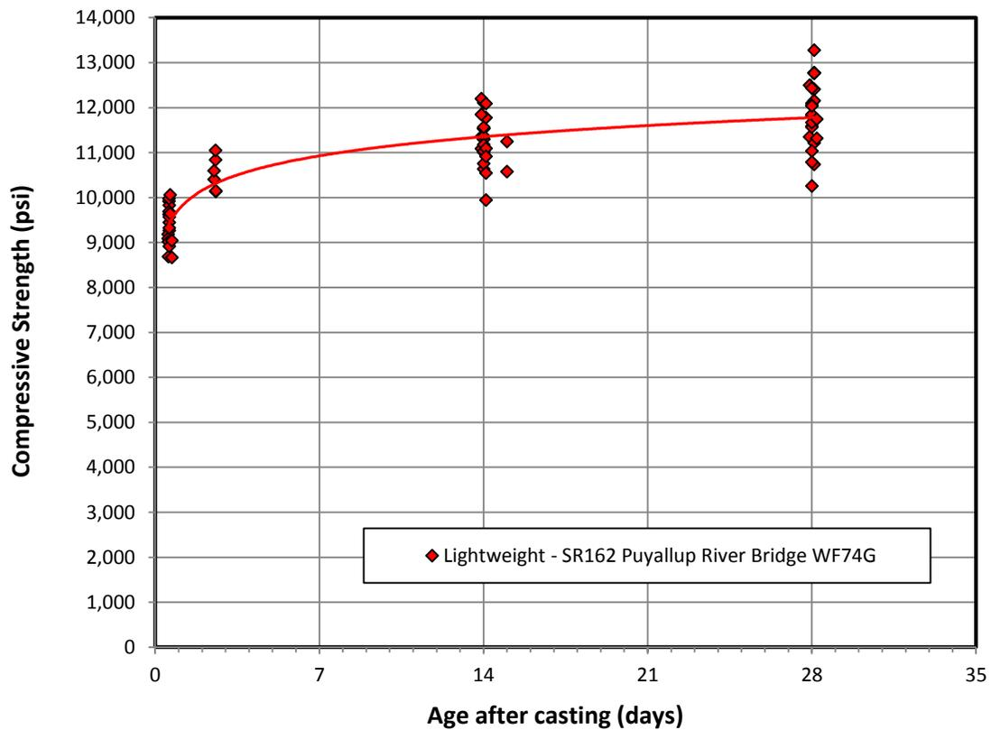
Fig. 8 Compressive strength versus age of concrete (SR162 Puyallup River Bridge)
