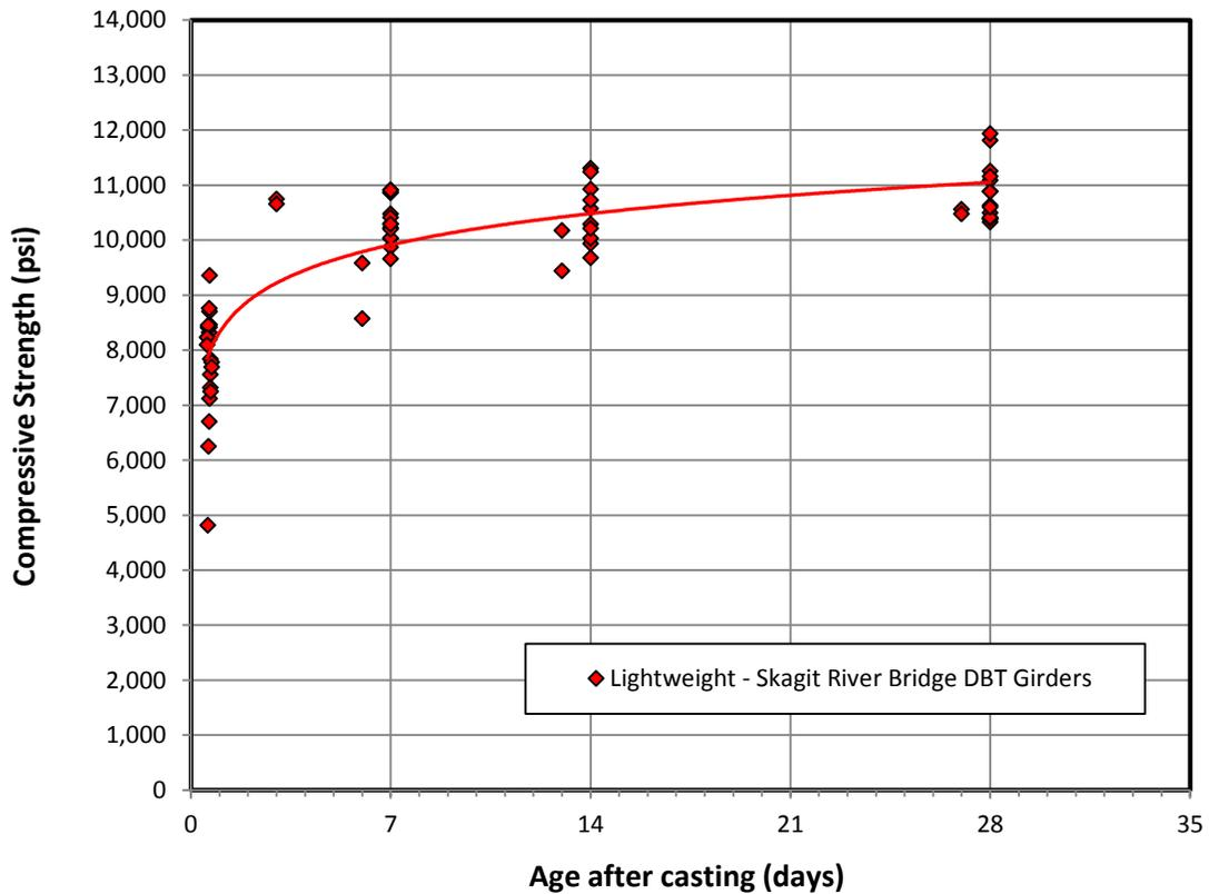
Fig. 7 Compressive strength versus age of concrete (Skagit River Bridge)
