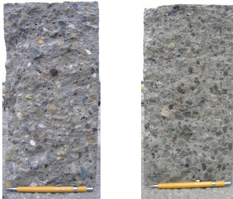
Fig. 15 Splitting tensile strength specimens after testing (NWC - left, LWC - right)
