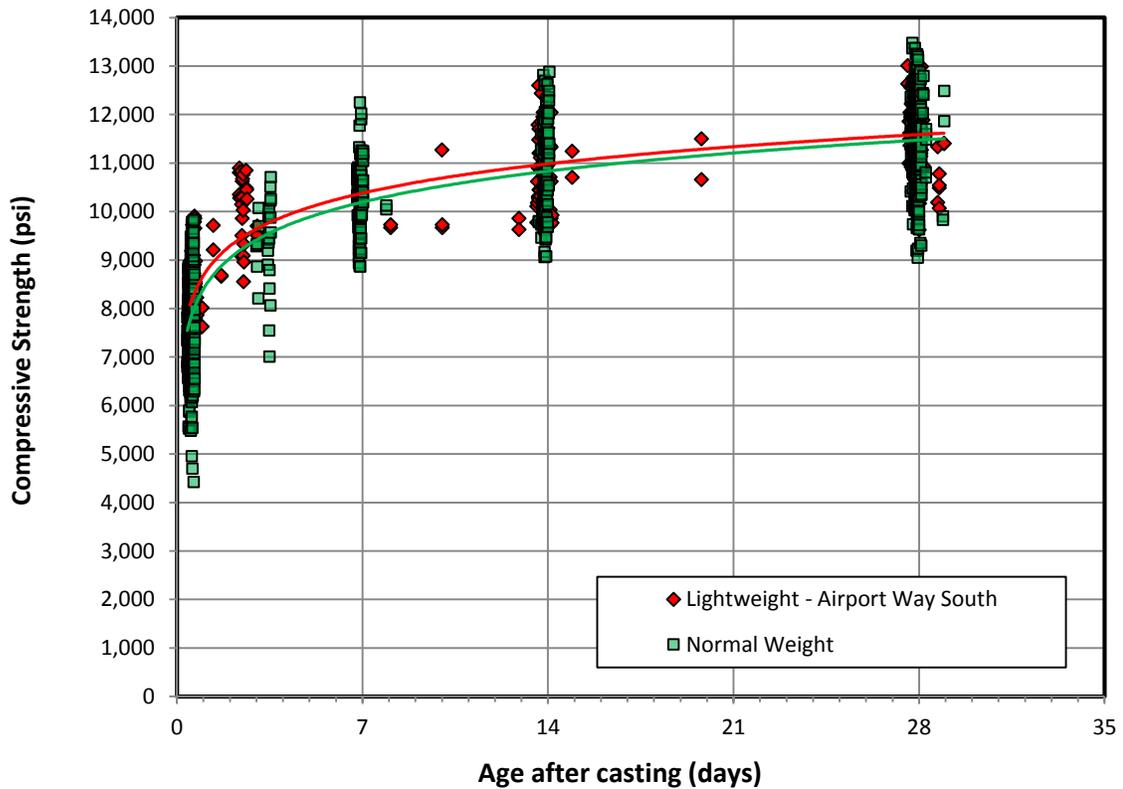
Fig. 6 Compressive strength versus age of concrete (Airport Way South)
