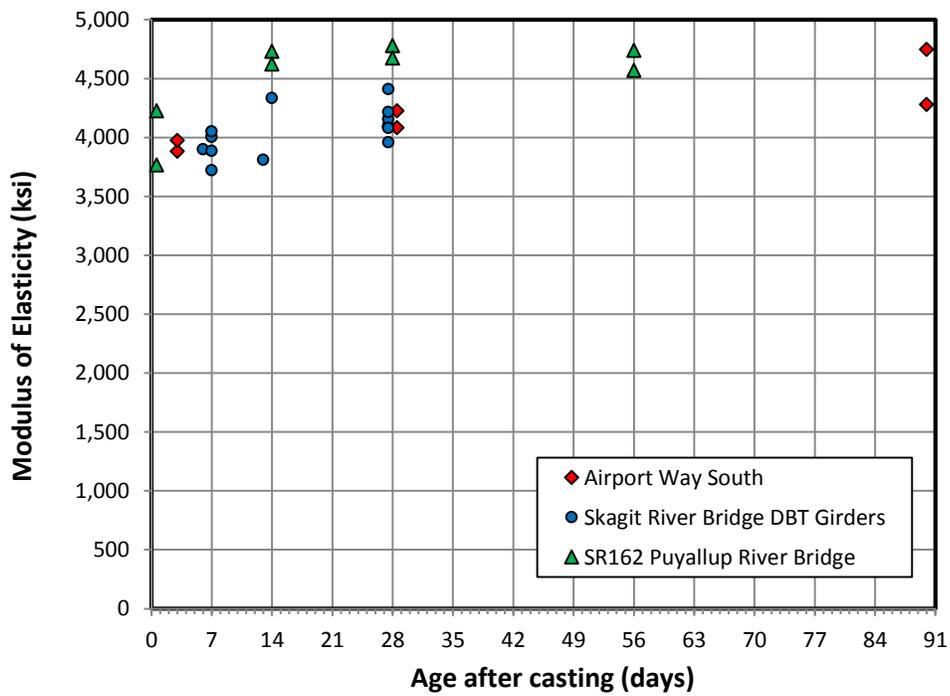
Fig. 10 Measured modulus of elasticity for sand lightweight concrete (all three projects)
