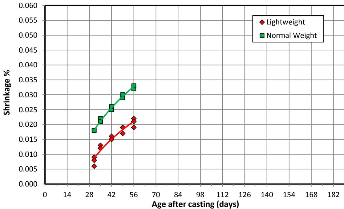
Fig. 13 Measured shrinkage (spring 2015, Puyallup River Bridge & Normal Weight)
