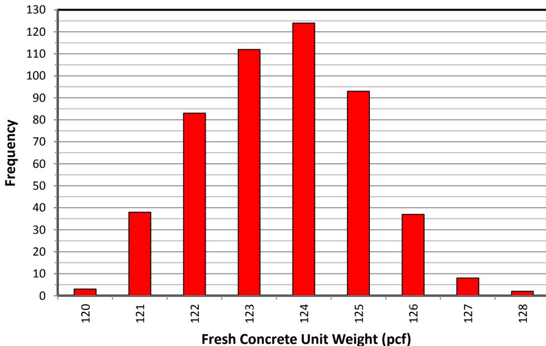
Fig. 5 Fresh Concrete Unit Weight Histogram (Airport Way South)
