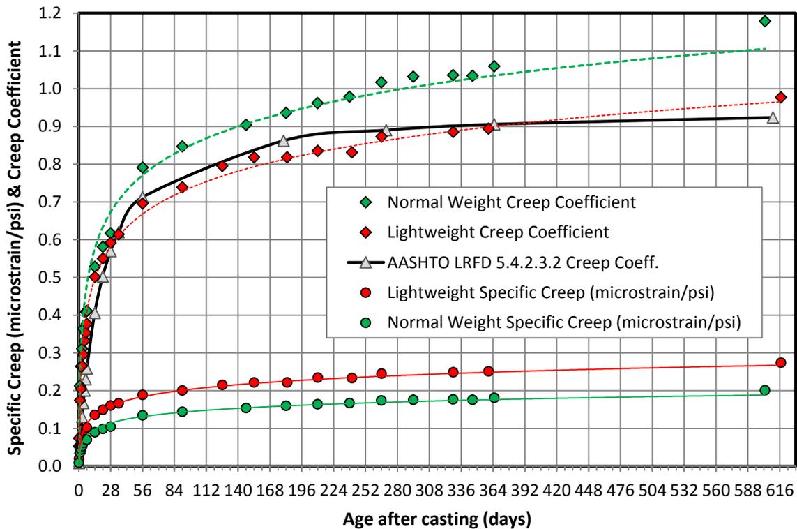
Fig. 11 Measured and predicted creep (Airport Way South)
