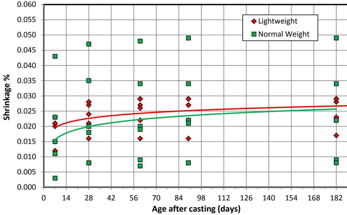
Fig. 12 Measured shrinkage (summer 2012, Airport Way South & Normal Weight)
