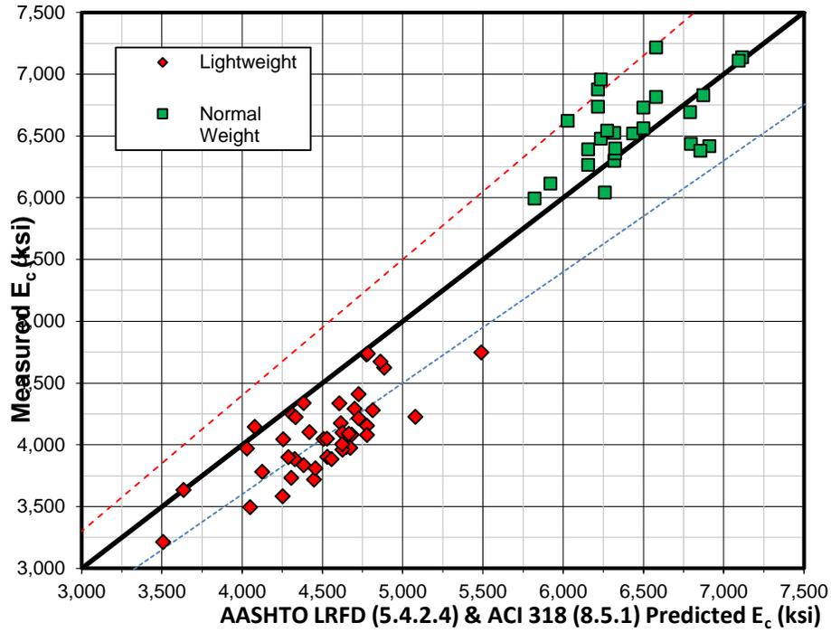
Fig. 9 Measured versus predicted modulus of elasticity for lightweight concrete and normal weight concrete (all three projects,  $K_1 = 1.0$  for all predictions)
