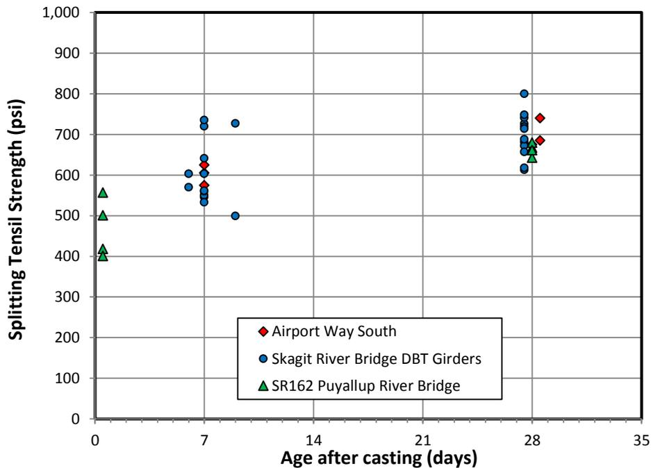
Fig. 14 Measured Splitting Tensile Strength versus Time (All Projects)
