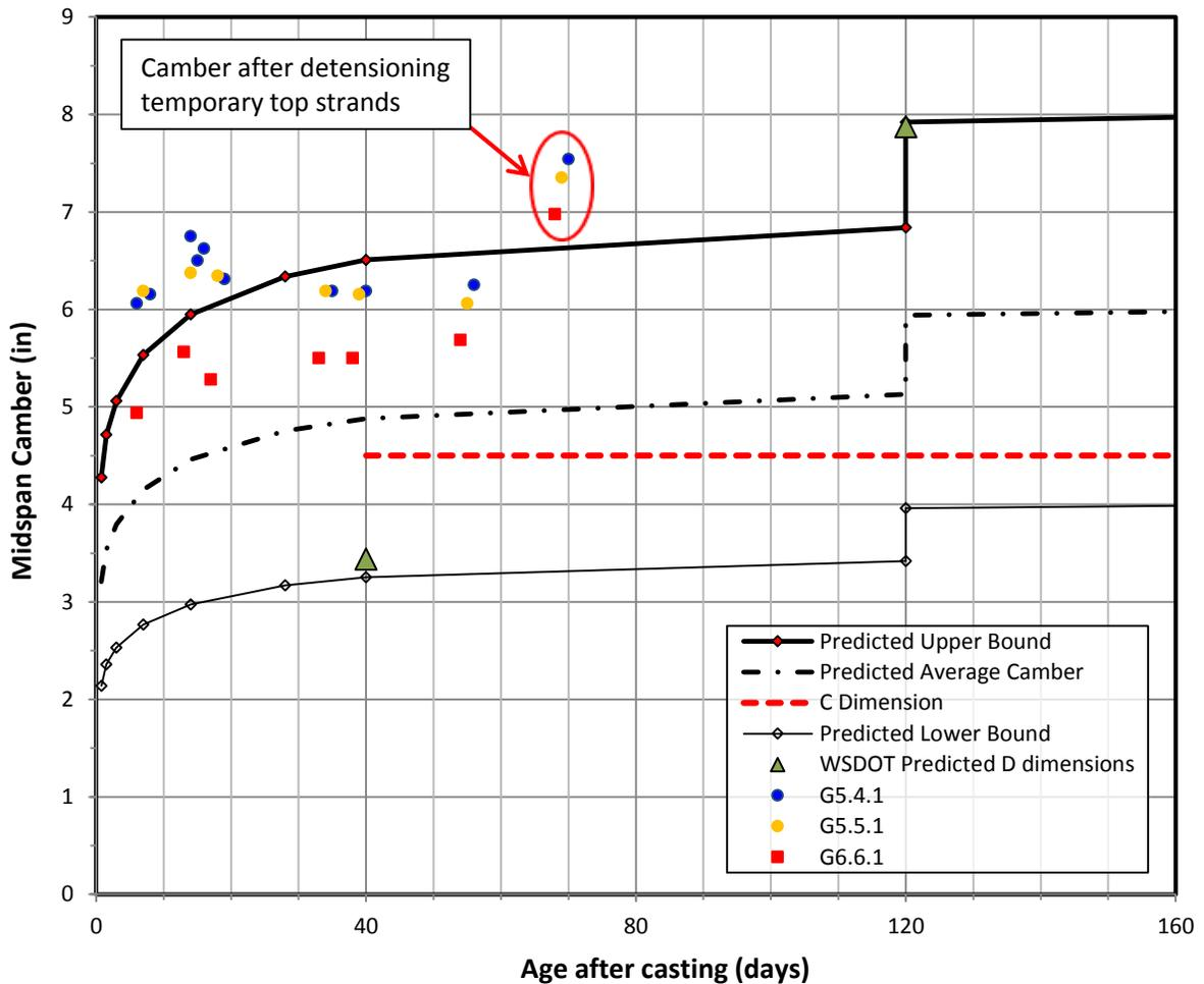
Fig. 17 Measured camber versus age after casting, SR162 Puyallup River Bridge WF74Gs
