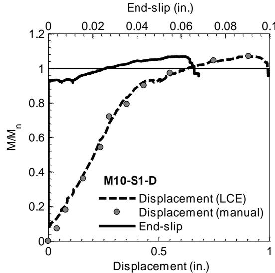
Fig. 7 Bending test results of the M10-S1-D specimen when tested at an embedment length of 3.25 ft (990 mm). In this figure, the dashed-line represents the relationship of  $M/M_n$  and the specimen deflection measured using the LCE. The gray dots are similar to the dashed-line, but the deflection was measured using a steel ruler. The solid-line represents the relationship of  $M/M_n$  and strand slippage. (Note:  $M$  = measured moment;  $M_n$  = nominal flexural capacity; 1 in. = 25.4 mm)
