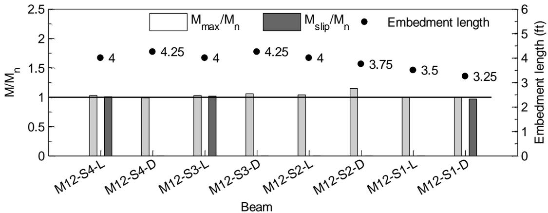
Fig. 12 Bending test results of the M12-S beams. (Note:  $M_{max}$  = maximum measured moment;  $M_{slip}$  = measured moment at which the prestressing strands began slipping;  $M_n$  = nominal flexural capacity; 1 ft = 305 mm.).
