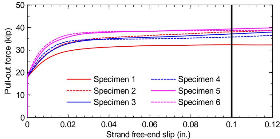
Fig. 2 Pull-out forces of the 6 strand specimens. (Note: 1 in. = 25.4 mm; 1 kip = 4.448 kN)
