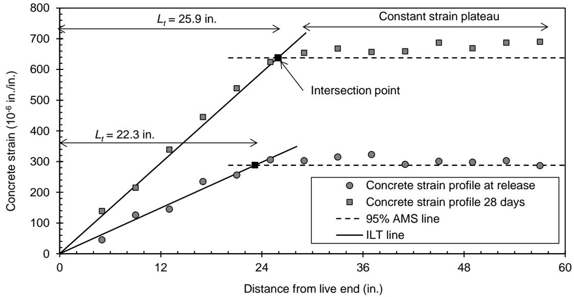
Fig. 5 Determination of transfer lengths at release and at 28 days of the M12-S1 beam. (Note:  $L_t$  = transfer length; AMS = Average Maximum Strain; ILT = initial linear trend; 1 in. = 25.4 mm)
