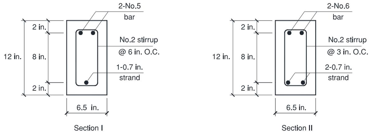
Fig. 3 Beam sections. Section I was used to cast 8 beams using the two concrete mixtures (M10-S1 to M10-S4 and M12-S1 to M12-S4), and section II was used to cast 4 beams using the M12 mixture (M12-D1 to M12-D4) as presented in Table 1. (Note: 1 in. = 25.4 mm; No.2 = 6.4 mm; No.5 = 16 mm; No.6 = 19 mm; 0.7 in. strand = 17.8 mm strand)
