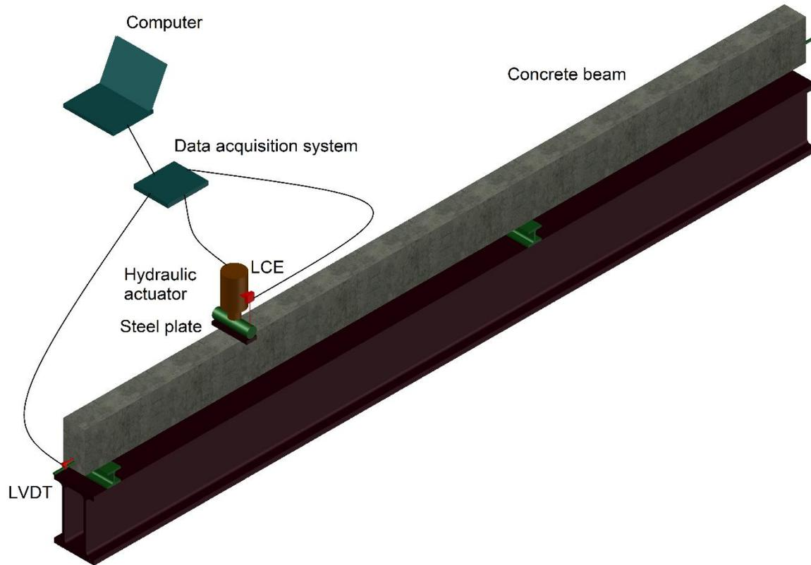
Fig. 6 Bending test frame. In this figure, the strand slippage is quantified using a LVDT.
