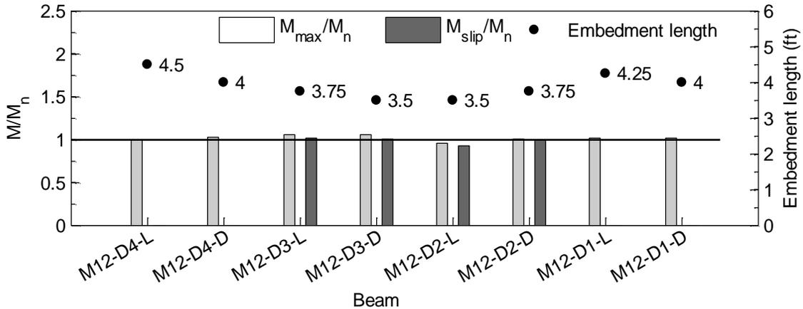
Fig. 14 Bending test results of M12-D beams. (Note:  $M_{max}$  = maximum measured moment;  $M_{slip}$  = measured moment at which the prestressing strands began slipping;  $M_n$  = nominal flexural capacity; 1 ft = 305 mm).
