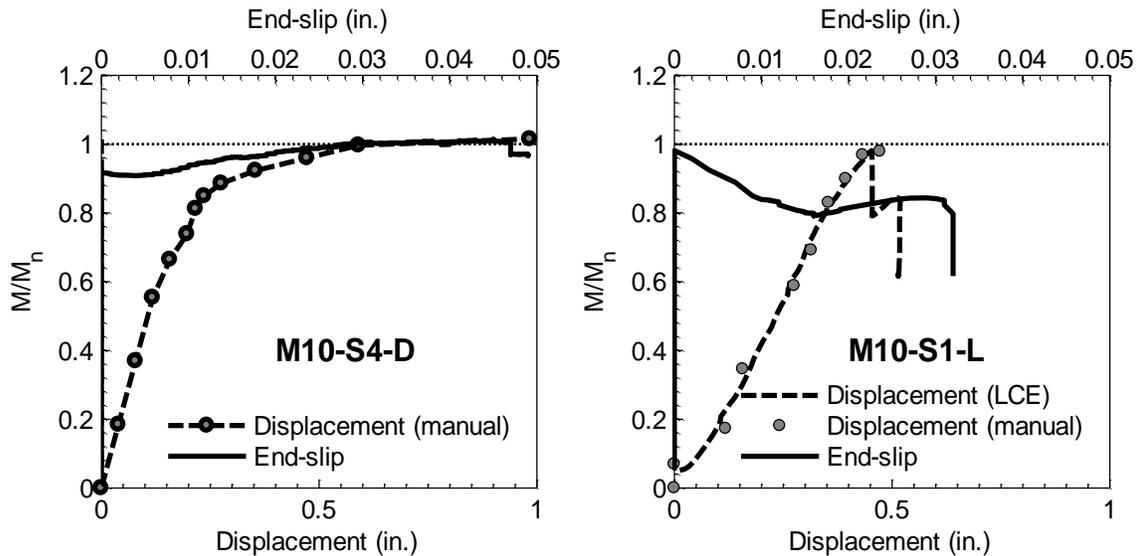
Fig. 11 Bending test results of the M10-S4-D and M10-S1-L specimens when tested at embedment lengths of 3.5 ft (1070 mm) and 3 ft (915 mm), respectively. (Note: 1 in. = 25.4 mm).
