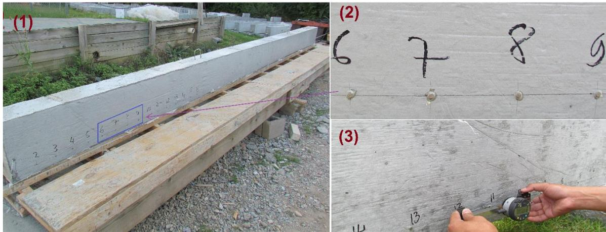
Fig. 4 (1) The attachment of a set of target points on the surface of a pretensioned concrete beam after removing the form; (2) A set of target points at a spacing of 4 in. (100 mm); (3) The use of mechanical strain gauge to measure concrete strains.
