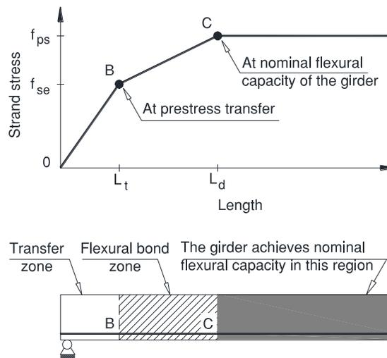
Fig. 1 Diagrams of transfer and development lengths. (Note:  $L_t$  = transfer length;  $L_d$  = development length;  $f_{se}$  = effective stress in the prestressing steel after losses;  $f_{ps}$  = is average stress in prestressing strand at the time for which the nominal flexural resistance of the member is required)
