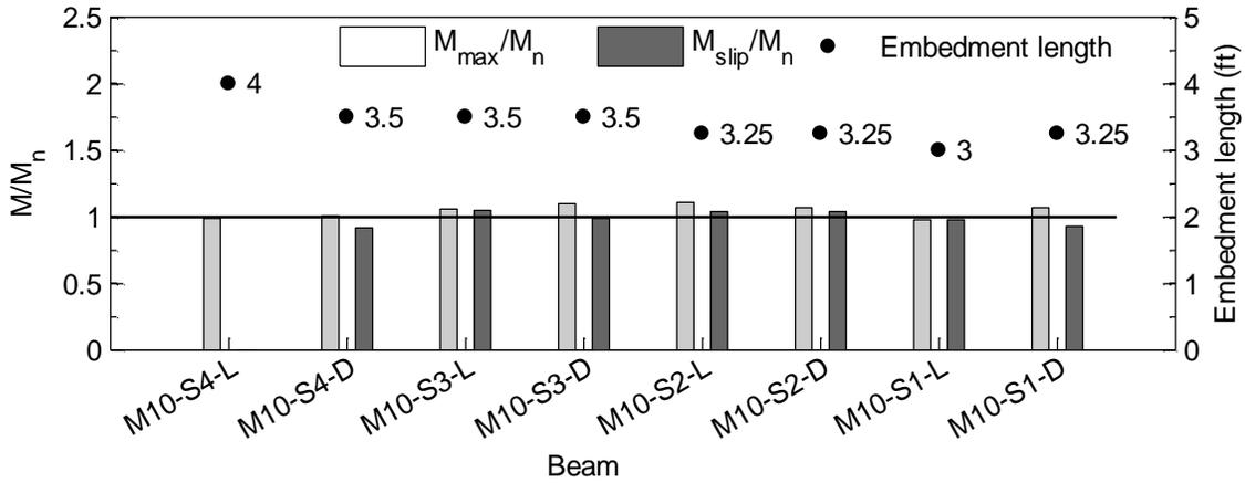
Fig. 10 Bending test results of the M10-S beams. (Note:  $M_{max}$  = maximum measured moment;  $M_{slip}$  = measured moment at which the prestressing strands began slipping;  $M_n$  = nominal flexural capacity; 1 ft = 305 mm).
