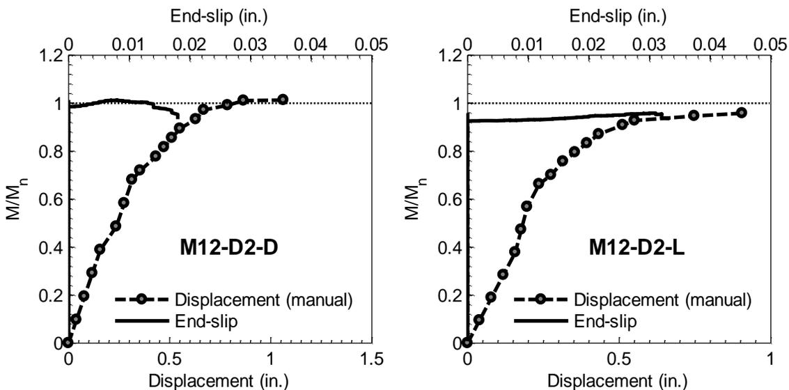
Fig. 15 Bending test results of the M12-D2-D and M12-D2-L specimens when tested at embedment lengths of 3.75 ft (1145 mm) and 3.5 ft (1070 mm), respectively. (Note: 1 in. = 25.4 mm).
