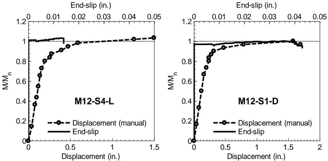
Fig. 13. Bending test results of the M12-S4-L and M12-S1-D specimens when tested at embedment lengths of 4 ft (1220 mm) and 3.25 ft (990 mm), respectively. (Note: 1 in. = 25.4 mm).
