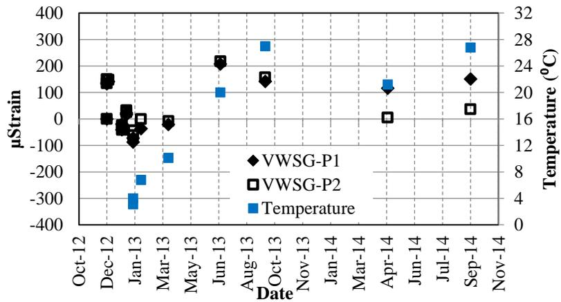
Fig. 12 Vibrating wire strain gage measurements – approach slab B
