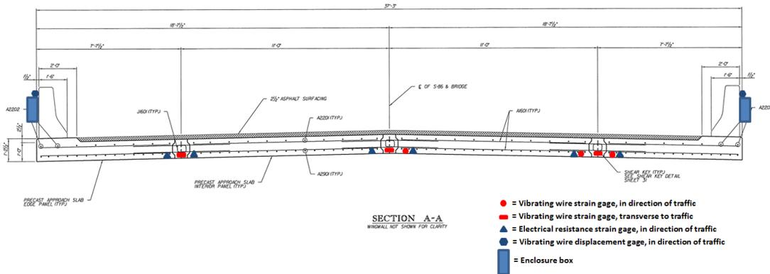
Fig. 6 Bent One approach slab schematic - cross-section
