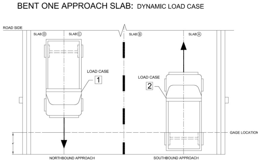
Fig. 9 Dynamic load case schematic
