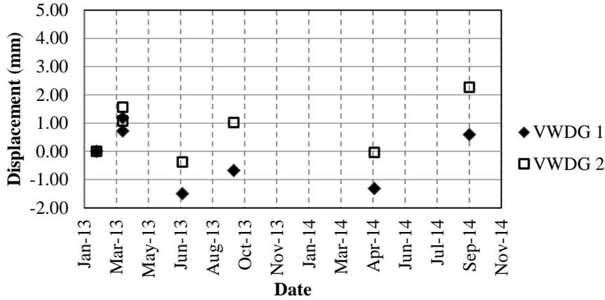
Fig. 14 Vibrating wire displacement gage measurements – Bent One
