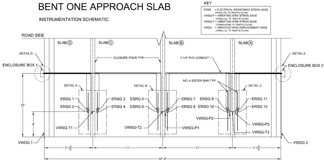
Fig. 5 Bent One approach slab schematic - plan view
