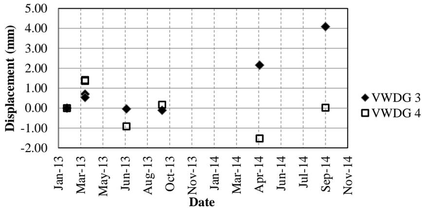
Fig. 15 Vibrating wire displacement gage measurements – Bent Four
