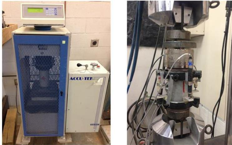
Fig. 7 Compressive strength testing (left); modulus of elasticity testing (right)
