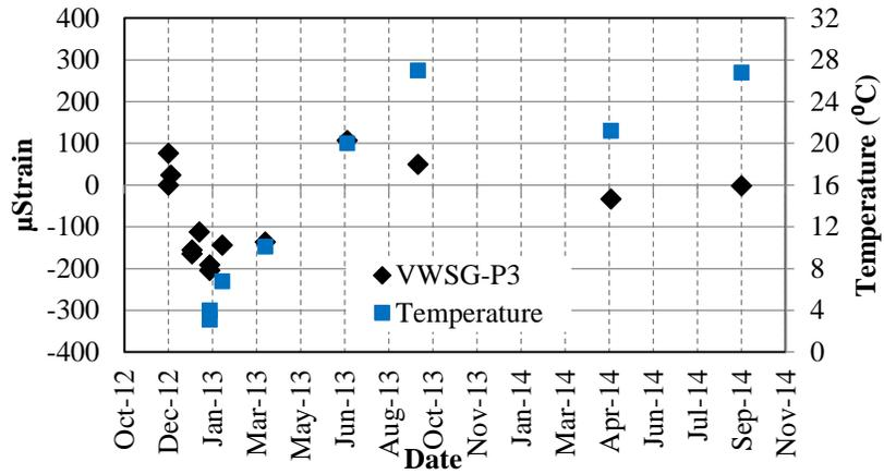
Fig. 11 Vibrating wire strain gage measurements - approach slab 'A'
