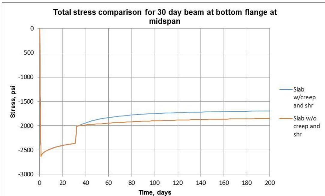
Figure 9 – Stress in the bottom flange at midspan for the case of placing the deck at 30 days.
