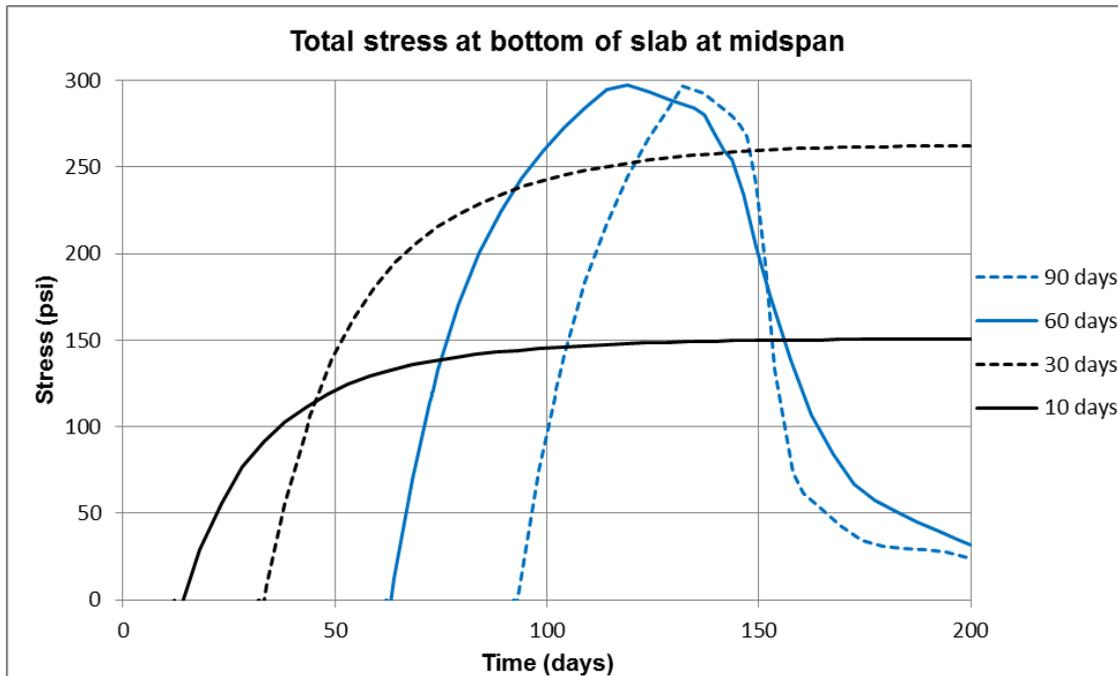
Figure 4 – Stress at the bottom of the slab vs. time for decks placed at different girder ages.
