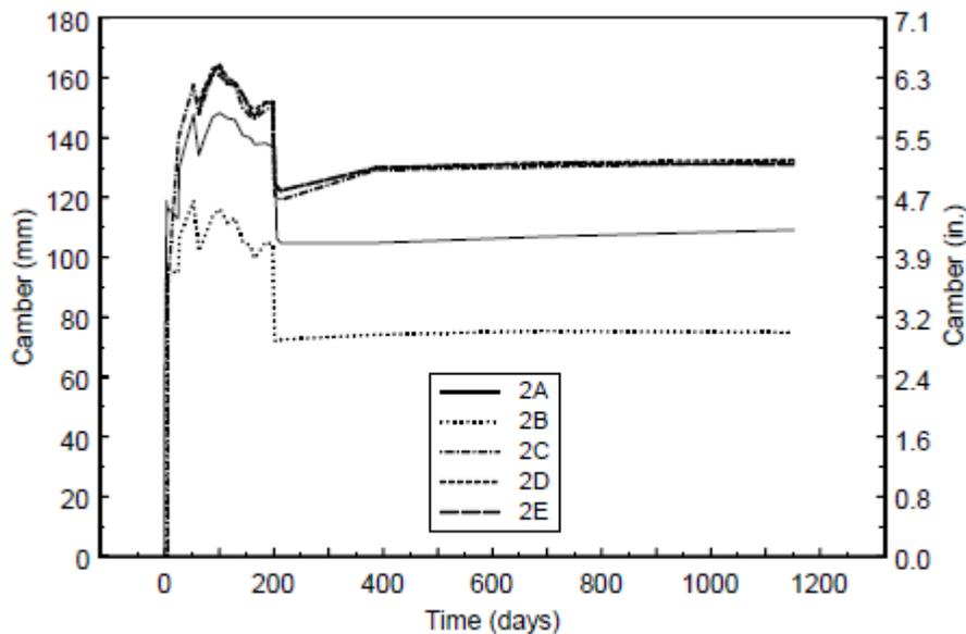
Figure 2 – Camber of girders with time (from Barr et al.<sup>6</sup>)
