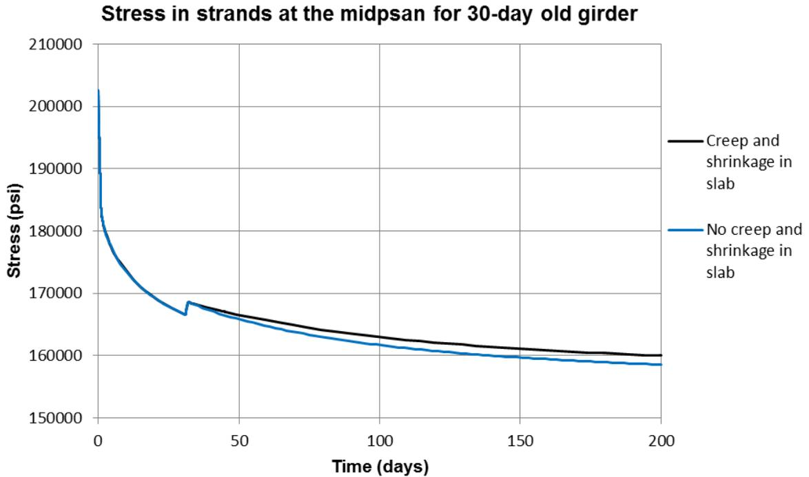
Figure 7 – Prestressing stress vs time for the case of deck slab placement at a girder age of 30 days; considering and ignoring creep and shrinkage of the slab.
