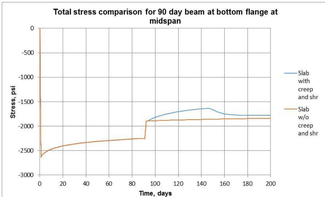
Figure 10 - Stress in the bottom flange at midspan for the case of placing the deck at 90 days
