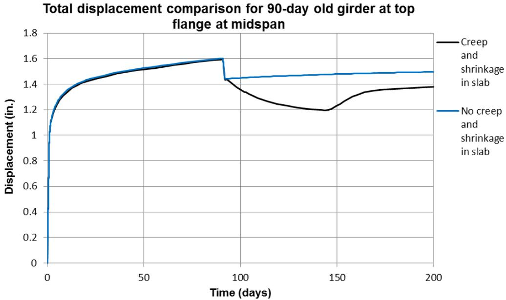
Figure 5 – Camber of the girder considering and ignoring creep, shrinkage and cracking of the deck.
