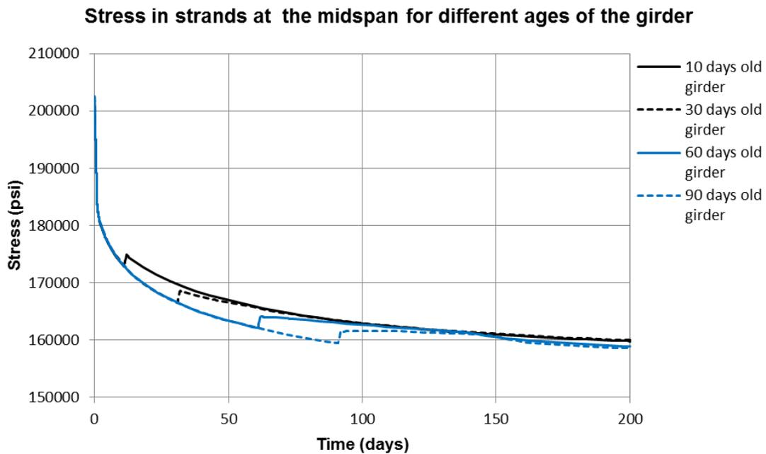
Figure 6 – Variation of prestressing stress with time for decks placed at different ages of the girder.
