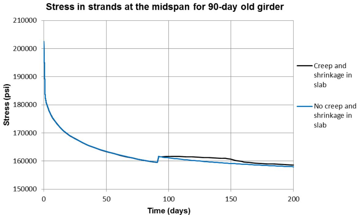
Figure 8 – Prestressing stress vs time for the case of deck slab placement at a girder age of 90 days; considering and ignoring creep and shrinkage of the slab.
