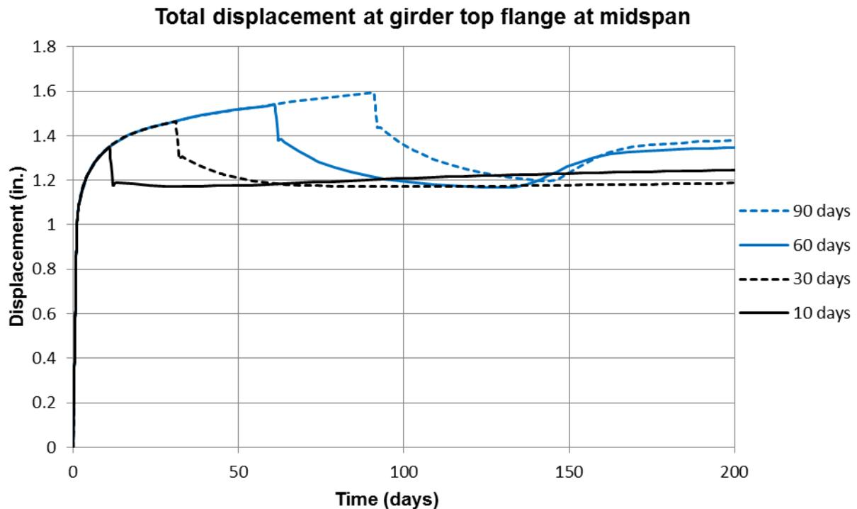
Figure 3 – Displacement of the top flange with time for decks cast at various ages.
