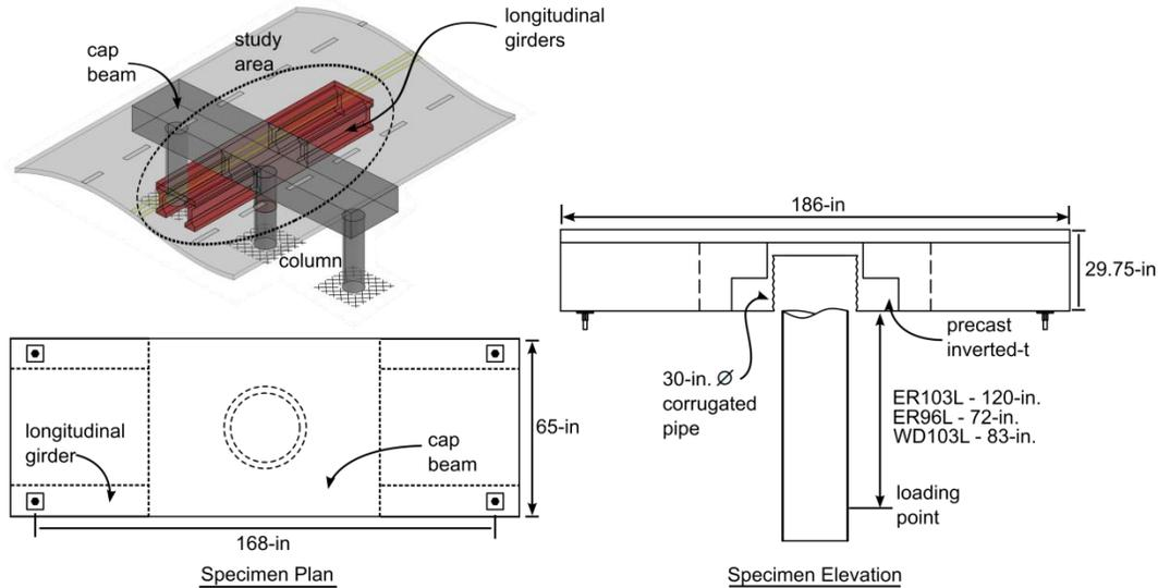
Fig. 7 Longitudinal study region and scaled specimen geometry
