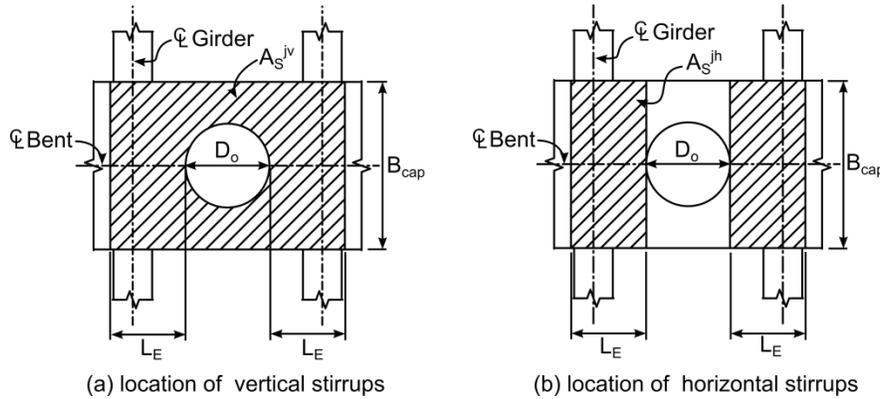
Fig. 14. Required location of (a) vertical and (b) horizontal stirrups for the embedded ring connection
