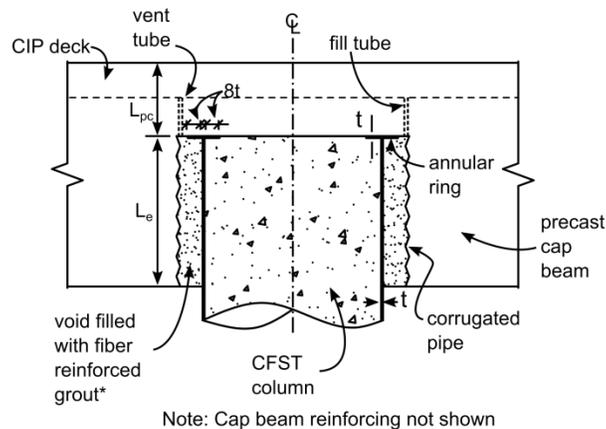
Fig. 12. Embedded Ring Connection
