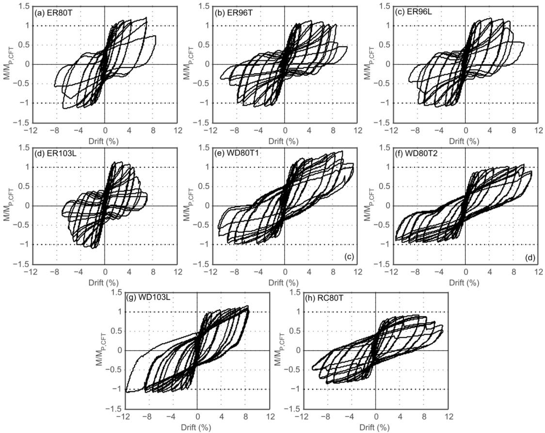
Fig. 10 Experimental moment-drift behaviors
