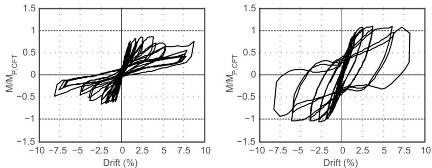
(a) Inadequately Embedded Specimen (b) Adequately Embedded Specimen
