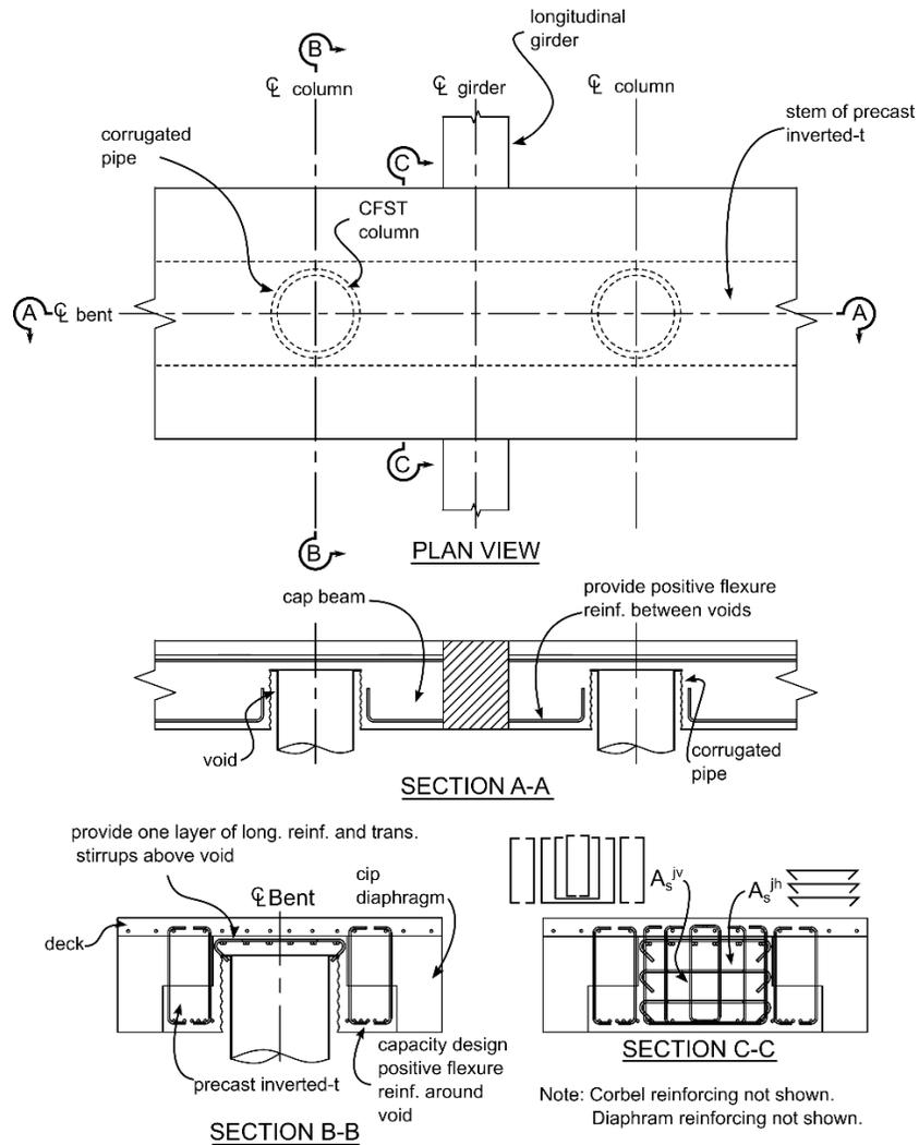
Fig. 13 Cap beam details for embedded connection
