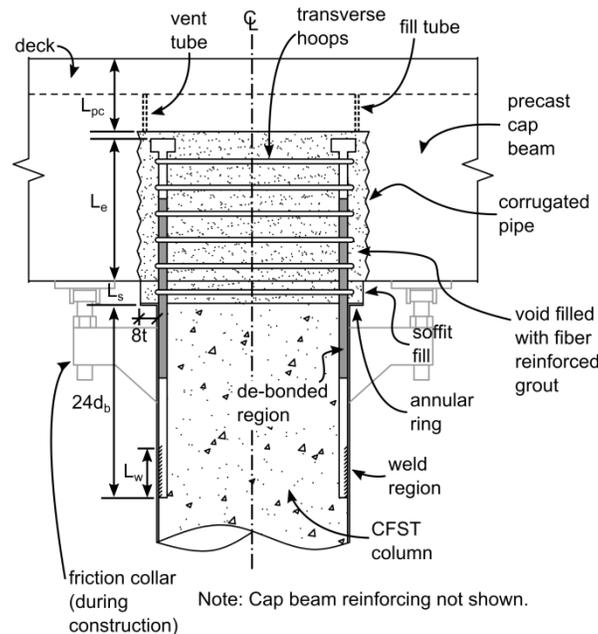
Fig. 15. Welded dowel connection
