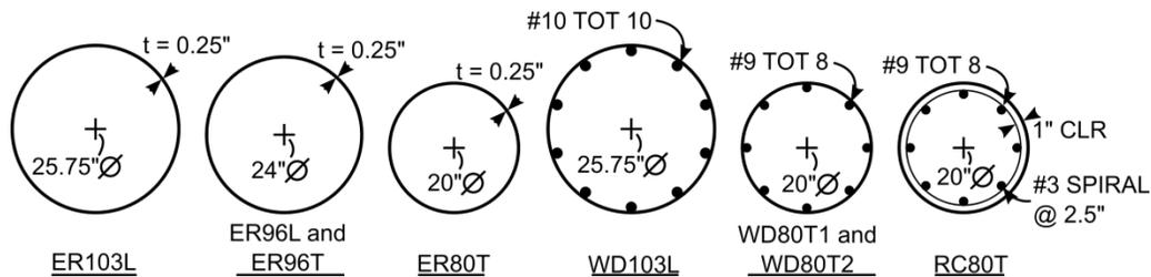
Fig. 8 Column cross sections in connection region
