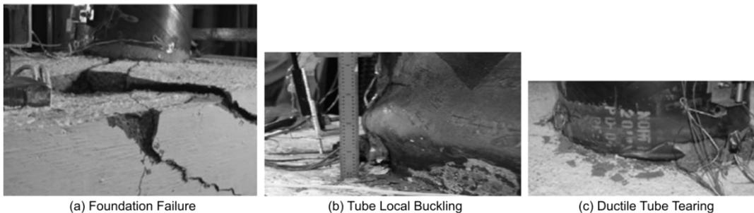
(a) Foundation Failure
