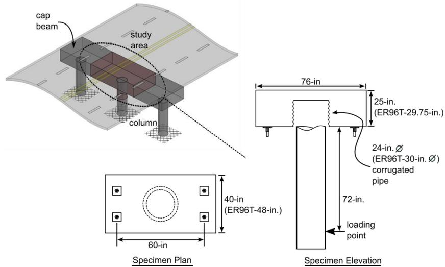
Fig. 6 Transverse study region and scaled specimen geometry.
