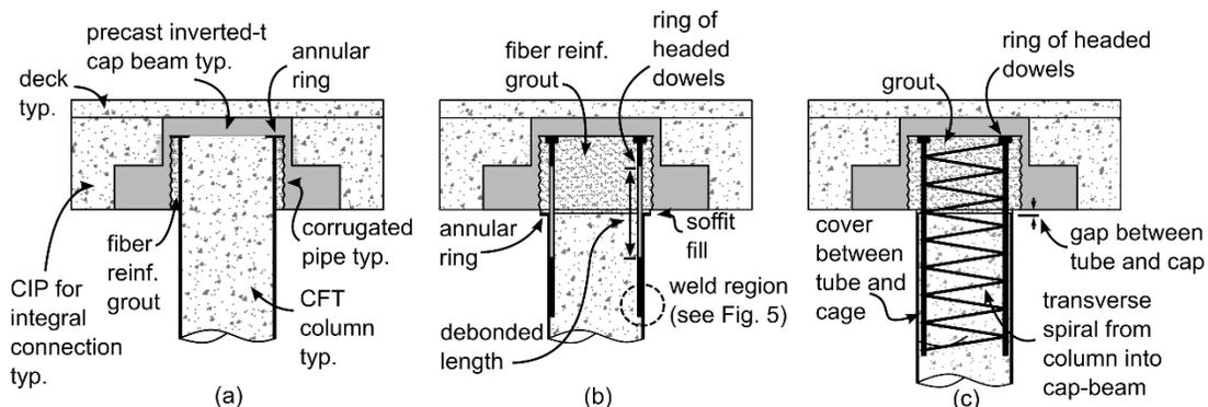
Fig. 4 Proposed CFST Column-to-Precast Cap Beam Connections. (a) Embedded Ring Connection (ER), (b) Welded Dowel Connection (WD), and (c) Reinforced Concrete Connection (RC)
