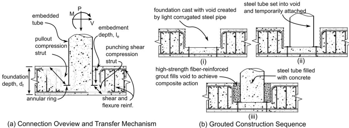
Fig. 1 CFST column-to-foundation connection
