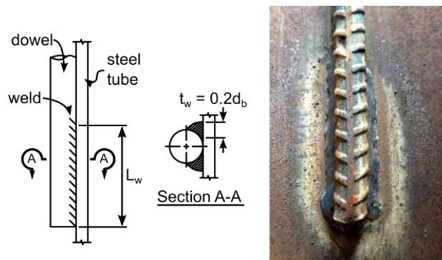
Fig. 5 Flare Bevel Groove Weld Between Longitudinal Dowel and Steel Tube
