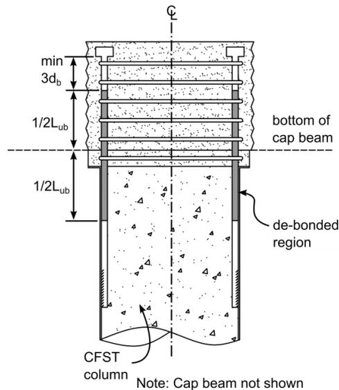
Fig. 16. Welded dowel connection de-bonding dimensions
