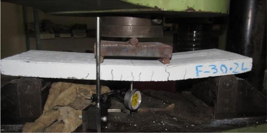
Figure 5.7 Front view of panel crack pattern for a sample of F4 group
