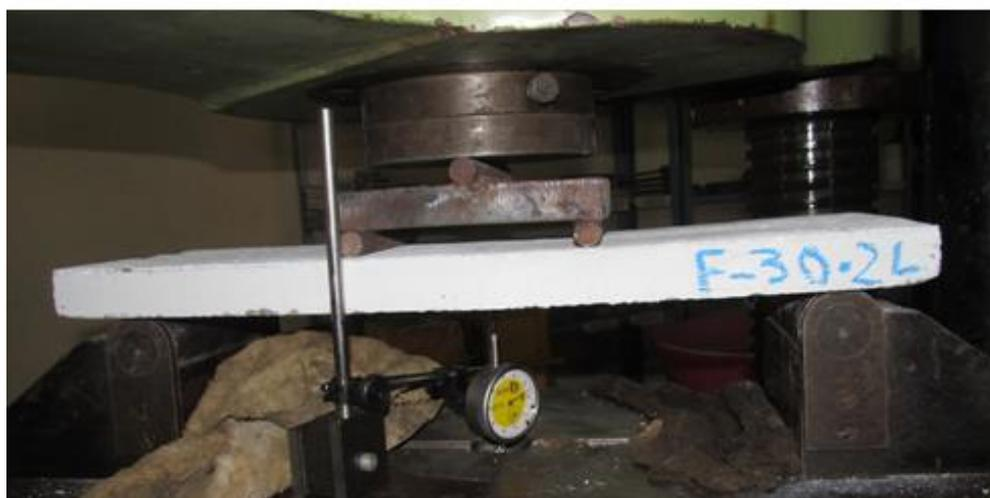
Figure 4.2 Specimen set up under two point loads
