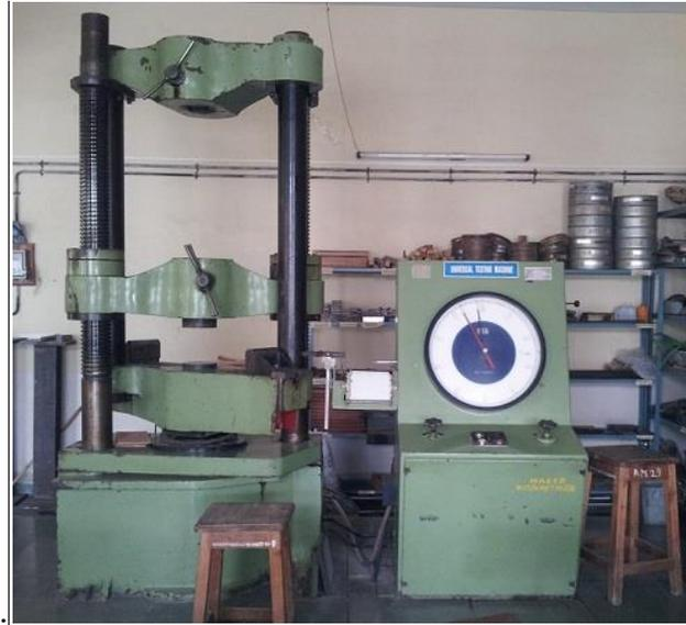
Figure 4.1 Universal Testing Machine
