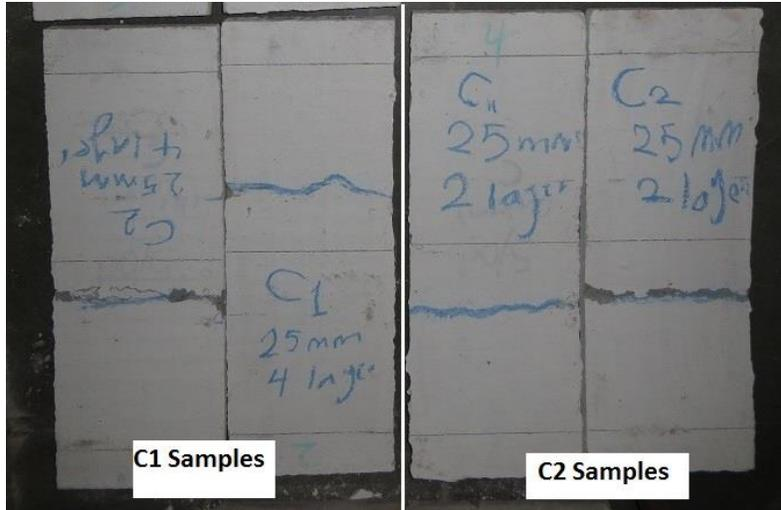
Figure 5.4 Top view of panel crack patterns for C1 and C2 Samples
