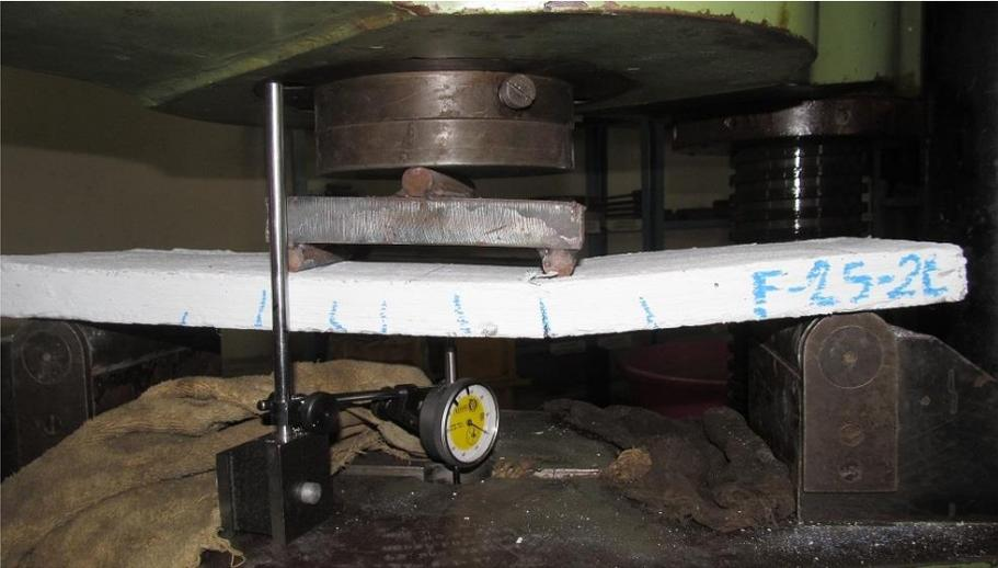
Figure 5.8 Front view of panel crack pattern for a sample of F2 group
