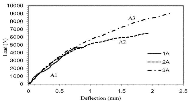
Figure 2.3 Load deflection curves for the folded panels
