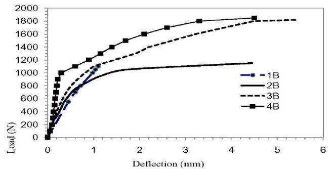
Figure 1.4 Load deflection curves for flat panels
