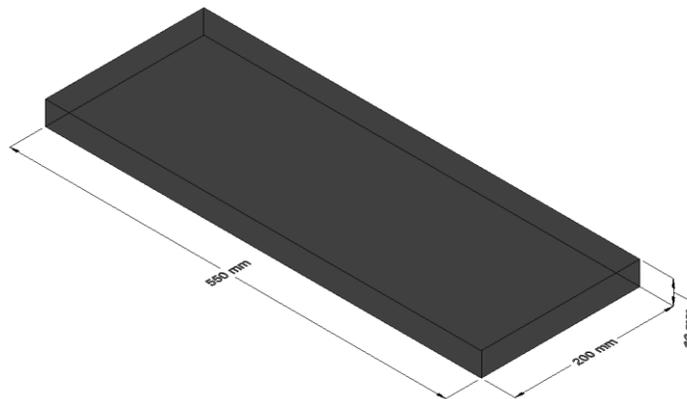
Figure 3- 2 Dimensions of the specimen with 30 mm thickness
