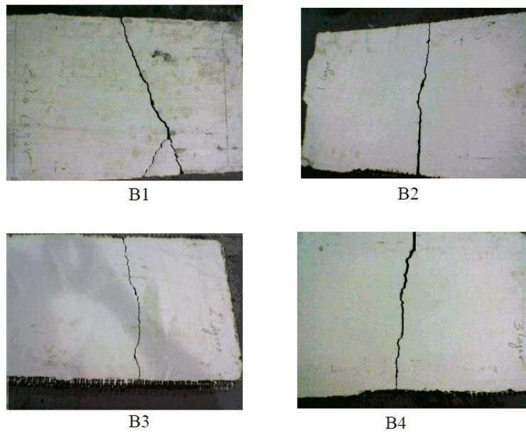
Figure 2.6 Crack pattern at the top face of the flat panels
