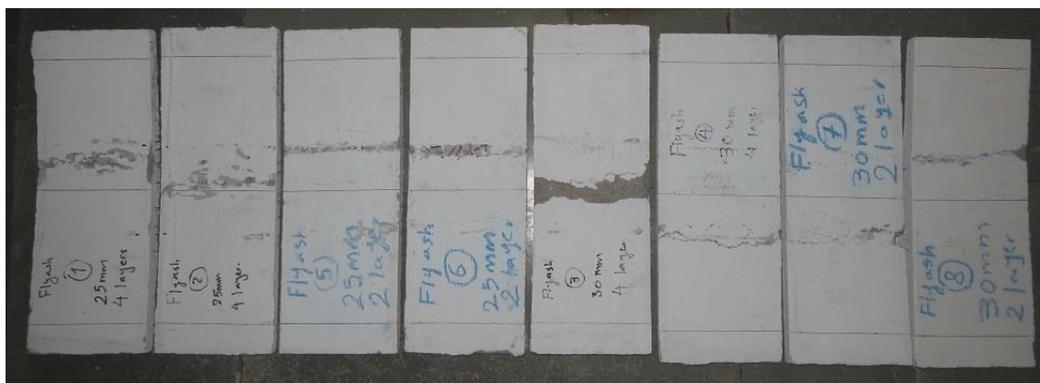
Figure 5.6 Top view of panel crack patterns of samples
