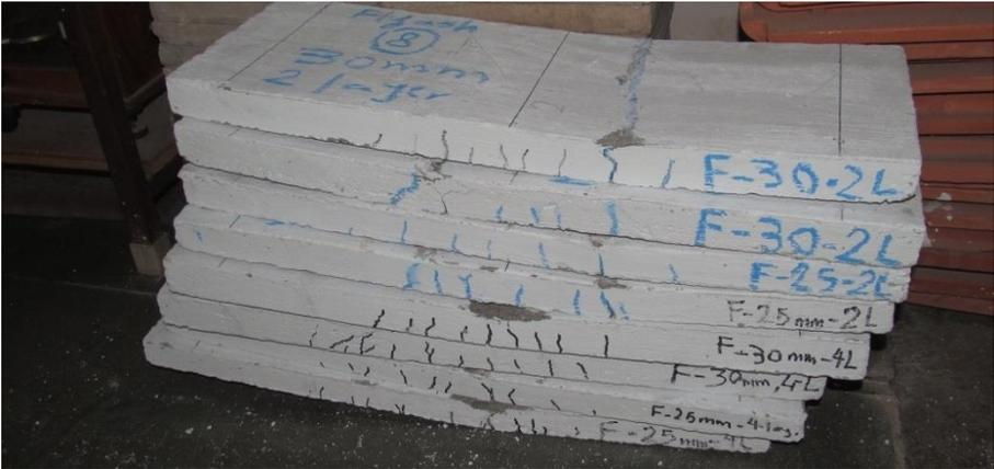
Figure 5.9 Front crack patterns of Samples
