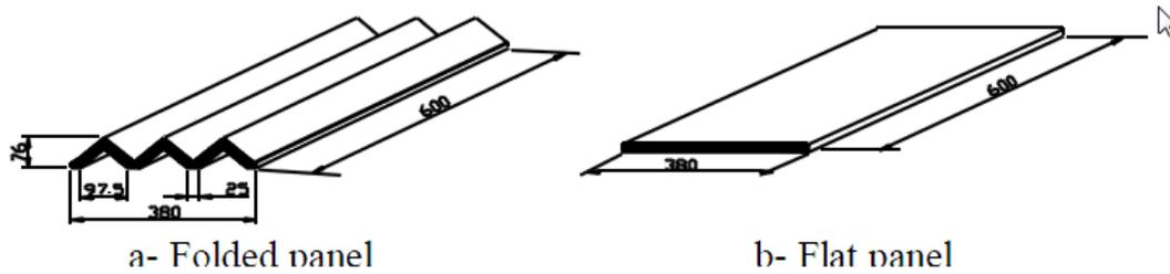
Figure 2- 1 Dimensions of the folded and flat panels (dimensions are in mm).
