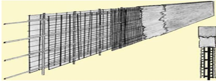
Figure1- 1 Typical cross section of ferrocement structure
