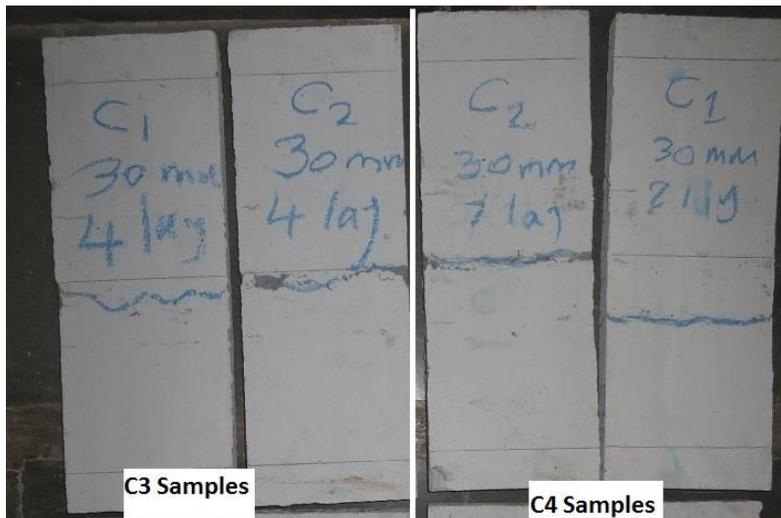
Figure 5.5 Top views of panel crack patterns for C3 and C4 samples
