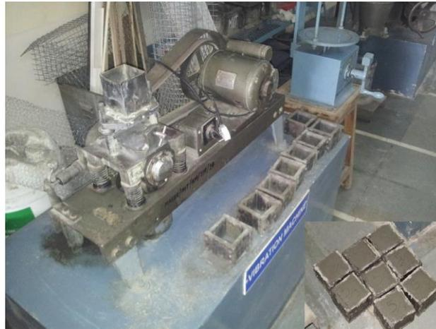
Figure 3.4 compressive test cubes
