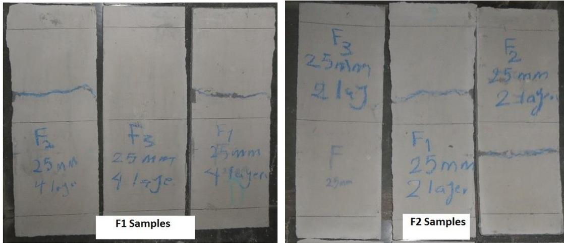
Figure 5.2 Top view of panel crack pattern for F1 & F2 Samples
