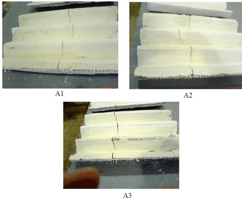
Figure 2.5 Crack pattern at the top face of the folded panels
