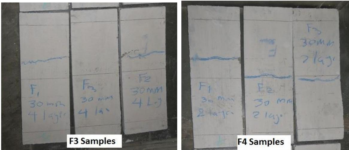
Figure 5.3 Top view of panel crack pattern for F3 & F4 Samples
