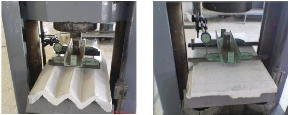
Figure 2- 2 set up of the tested folded and flat panels.
