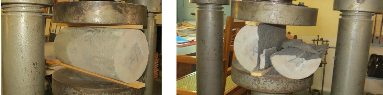
Figure 3.5 Tensile splitting tests
