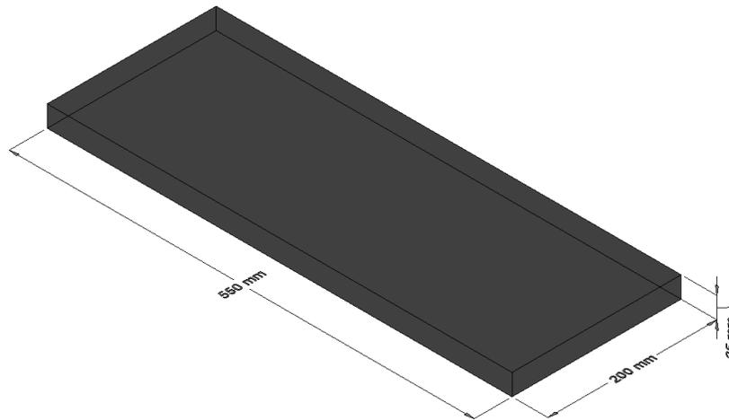
Figure 3- 1 Dimensions of the specimen with 25 mm thickness
