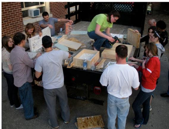
Fig. 7 “Stripping Party” at University working from precast company's flat bed truck which is strategically parked close to the dumpster
