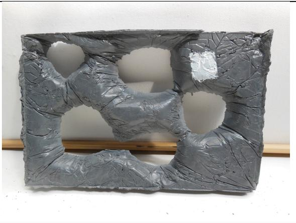
Fig. 28 Wrinkled Panel with Voids
