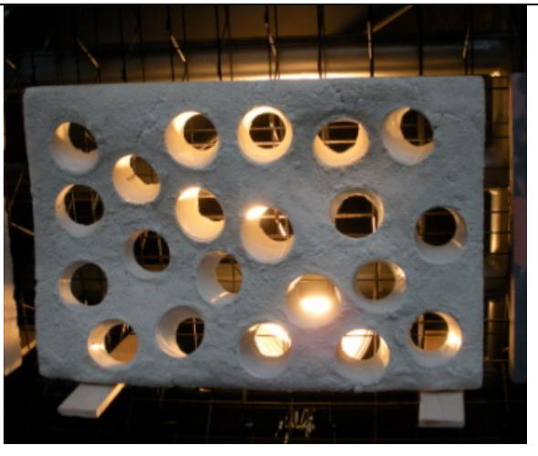
Fig. 30 Warped Grid Screen
