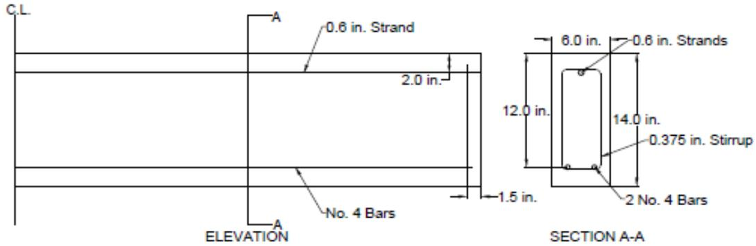
Figure 1: Cross-section details for a top strand beam, Note: 1 in. = 25.4 mm
