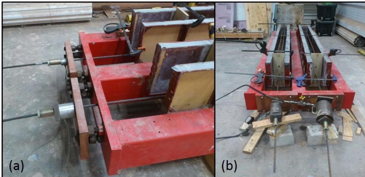
Figure 2: Prestressing setup showing (a) anchorage (dead) end and prestress release mechanism and (b) strand tensioning mechanism at the live end
