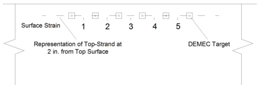
Figure 4: Representation of DEMEC Points and Surface Strain on a Typical Top-Strand Beam
