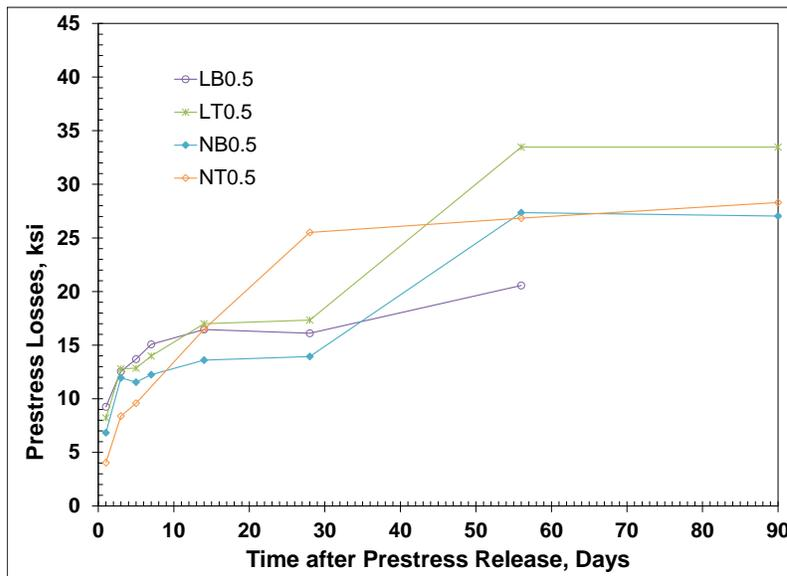
Figure 7 Total prestress losses of 0.5 in. special strand beam specimens, Note: 1 MPa = 145 psi
