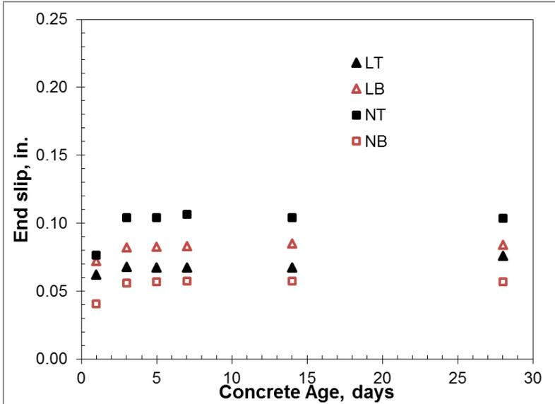
Figure 5: Comparison between all the 0.5 in. special specimens with averaged end slip values, Note: 1 in. = 25.4 mm
