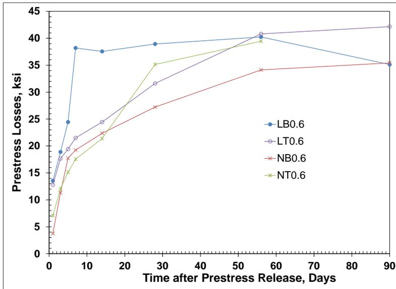
Figure 8. Total prestress losses of 0.6 in. strand beam specimens, Note: 1 MPa = 145 psi
