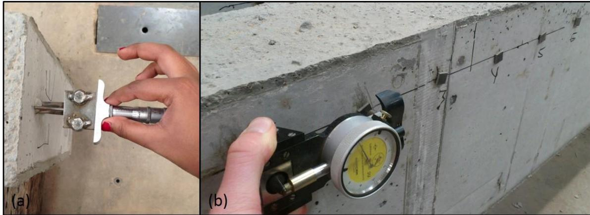
Figure 3: (a) End-slip measured using a depth micrometer and (b) DEMEC gauge used to measure surface strain for prestress losses
