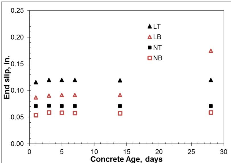
Figure 6: Comparison between all the 0.6 in. specimens with averaged end slip values, Note: 1 in. =25.4 mm
