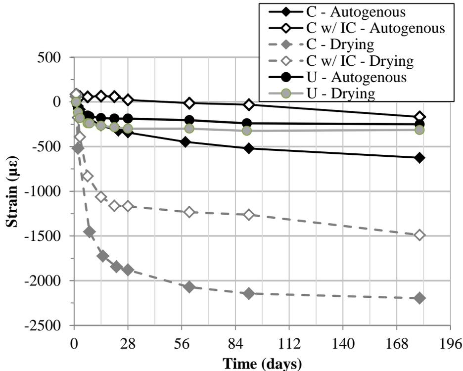
Fig. 7. Autogenous and drying shrinkage as a function of time
