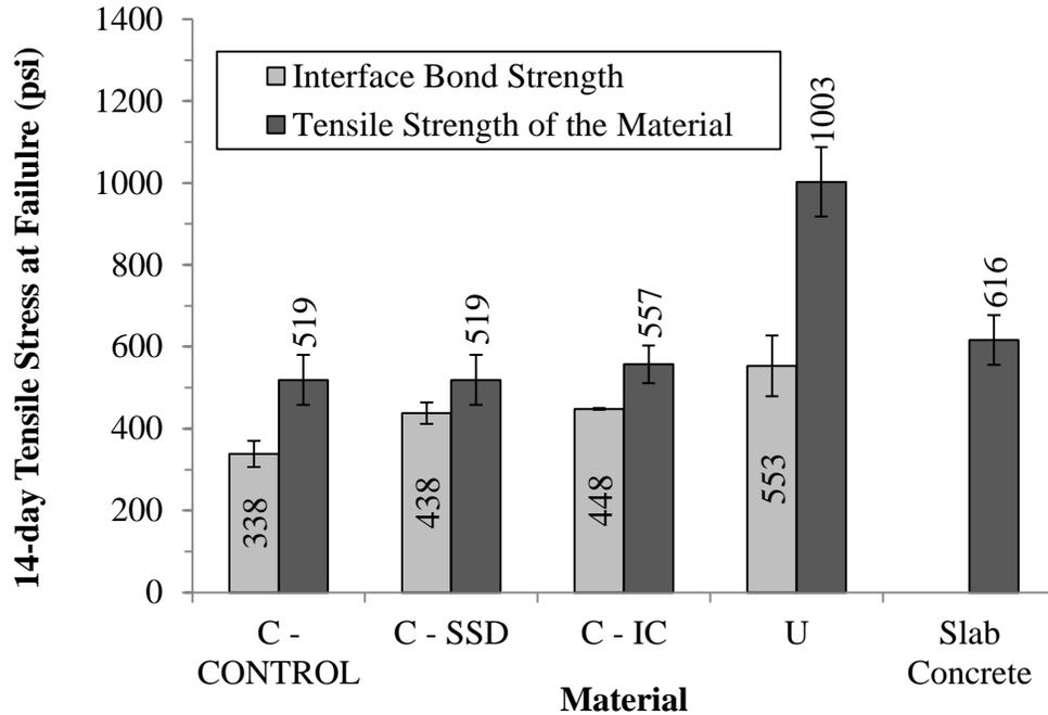
Fig. 6. 14-day pull-off bond strength: Effect of moisture at interface (SSD, IC), and use of UHPC material (U) (Error bars indicate one standard deviation from the average of four specimens)
