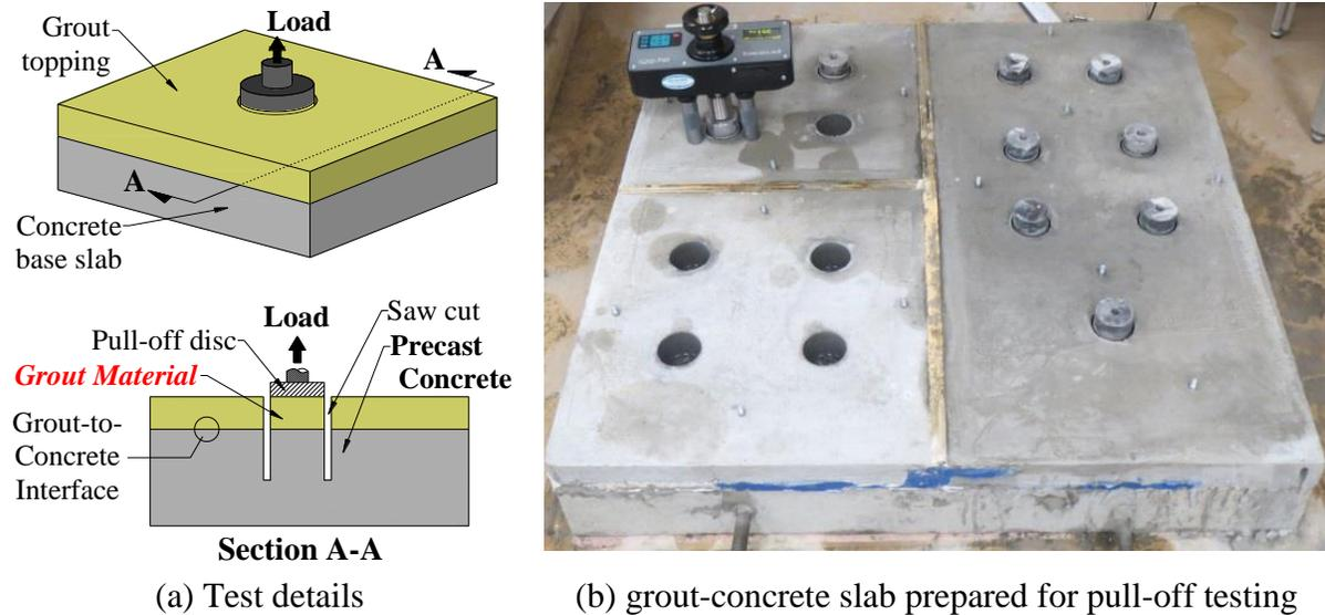
Fig. 3. ASTM C1583 Direct tension bond pull-off test
