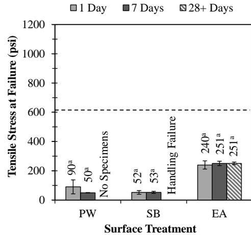
(b) Magnesium Phosphate Grout "M"
