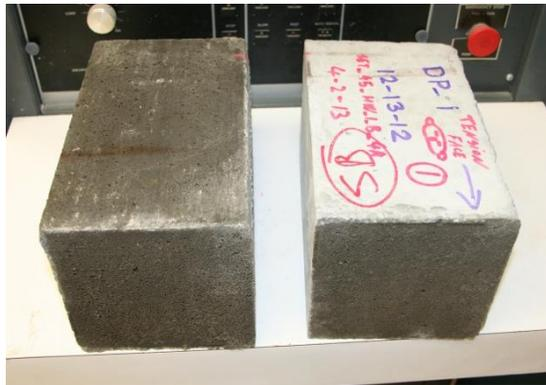
(a) Example of interface bond failure
