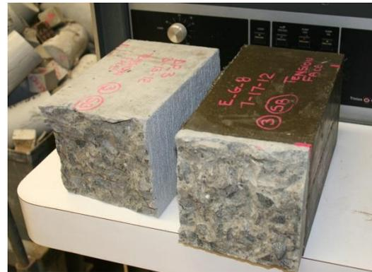
(b) Example of failure by tensile rupture of concrete
