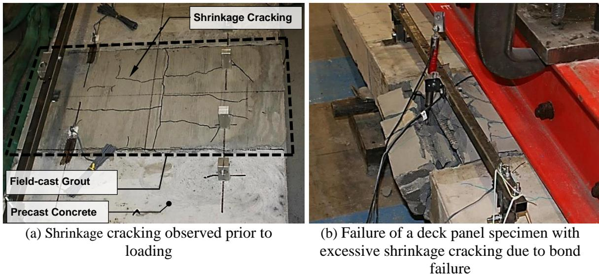
Fig. 1. Observations from deck panel connection tests using a non-shrink cementitious grout<sup>4</sup>
