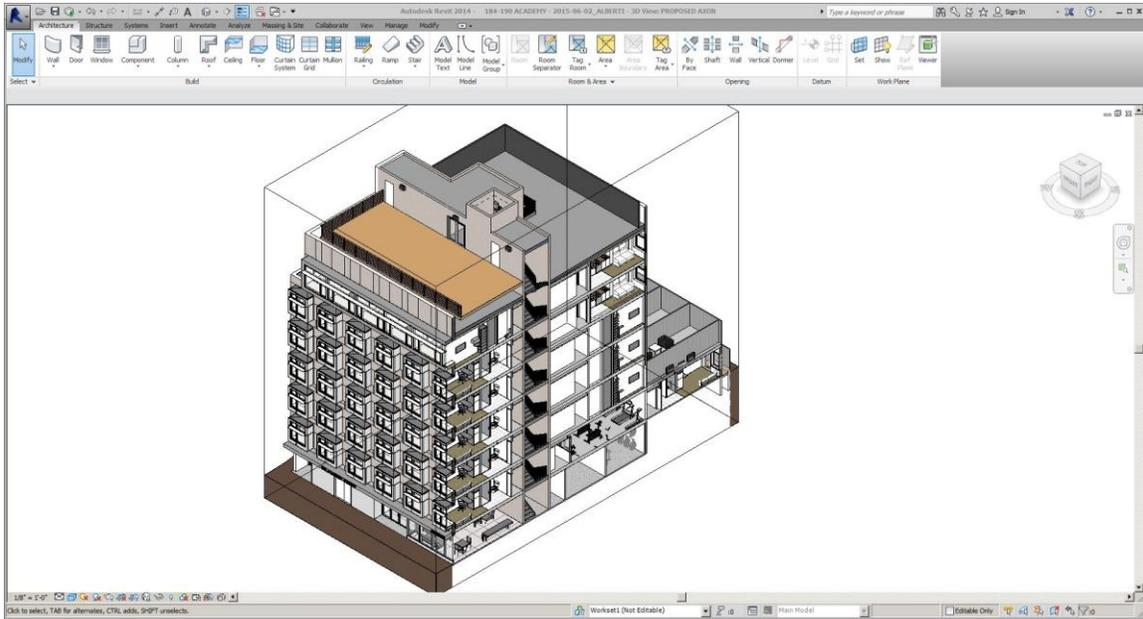
Figure 13: The architects used BIM package Autodesk Revit® to complete schematic design and move into the construction documentation phase of the project.
