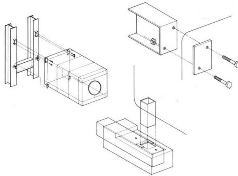
Figure 04: Units that make up the exterior of the Nakagin Capsule Tower were bolted to a steel frame with only four (4) tension bolts making it feasible to remove units for servicing.
