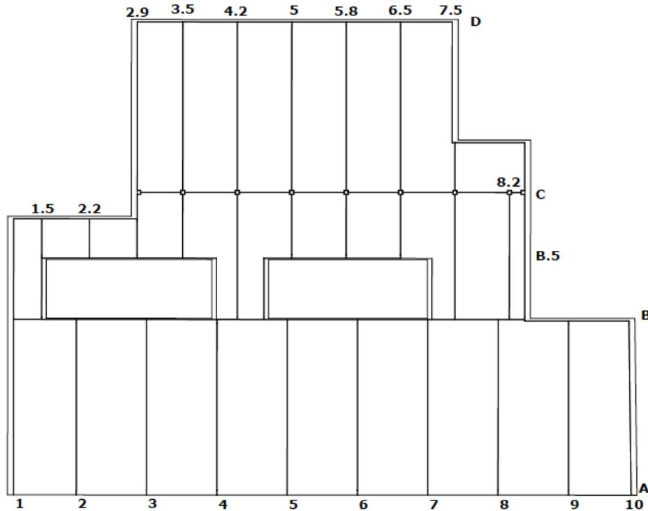
Figure 18: At the time of writing, a preliminary floor and wall plank layout had been arrived at and input into the architect’s Building Information Model. The three-dimensional data would ultimately be extracted to produce the two-dimensional fabrication drawings to ultimately form the panels.
