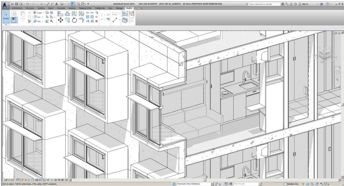
Figure 21: A cutaway section through the building's south façade reveals the monolithically poured front panels that contain the window boxes.
