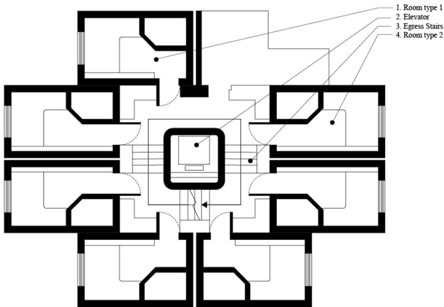
Figure 03: The Nakagin Capsule Tower, typically upper-floor unit cluster.
