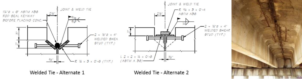
Figure 4: Connection of Deck Beam Elements
