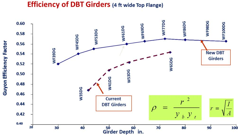
Figure 3: Efficiency of wide flange deck girder
