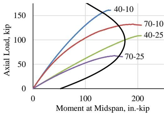
**Figure 5: Interaction Diagram (2 – PS Wires)**
