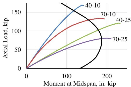
**Figure 7: Interaction Diagram (6 – PS Wires)**
