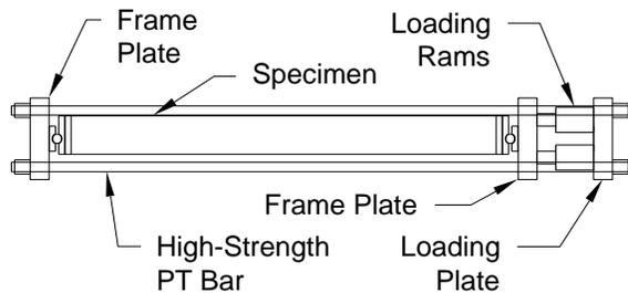
**Figure 3: Column Loading Frame**
