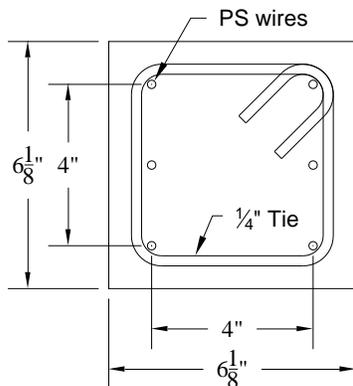
**Figure 1: Column Cross-Section**
