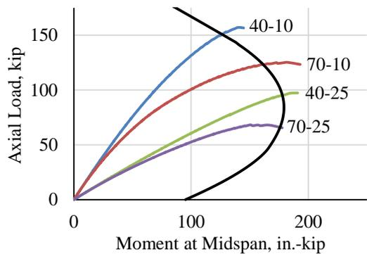
**Figure 6: Interaction Diagram (4 – PS Wires)**
