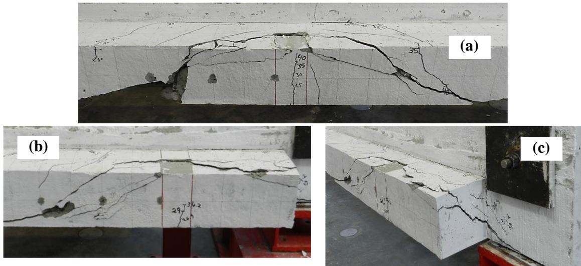
Figure 4: (a) Front View for Inner Ledge Failure (b) Front View for End Ledge Failure (c) Side View for End Ledge Failure
