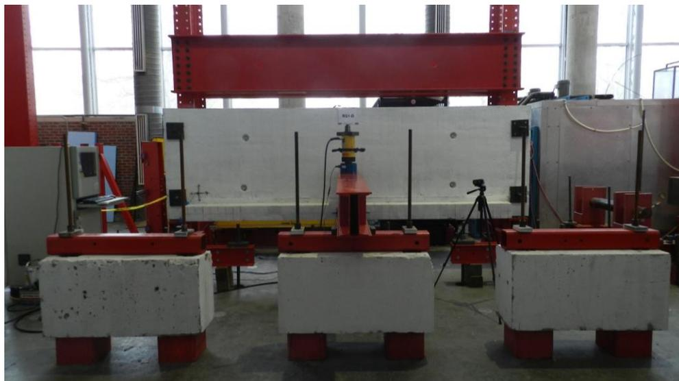
Figure 3: Test at Mid-span (Inner Failure)
