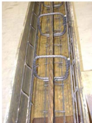
Fig. 6 Specimen Strand Confinement
