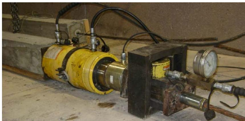
Fig. 7 Pull-out Testing Setup
