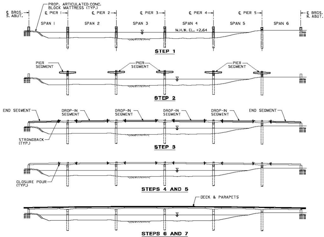
Figure 7 – Girder Erection Scheme
