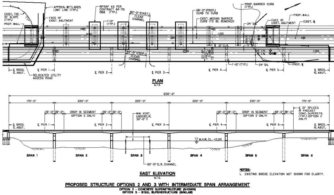
Figure 4 – Recommended Span Arrangement (Alternative 2)
