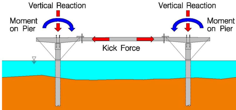
Figure 10 – Unbalanced Moment on Piers and Kick Force on Girders
