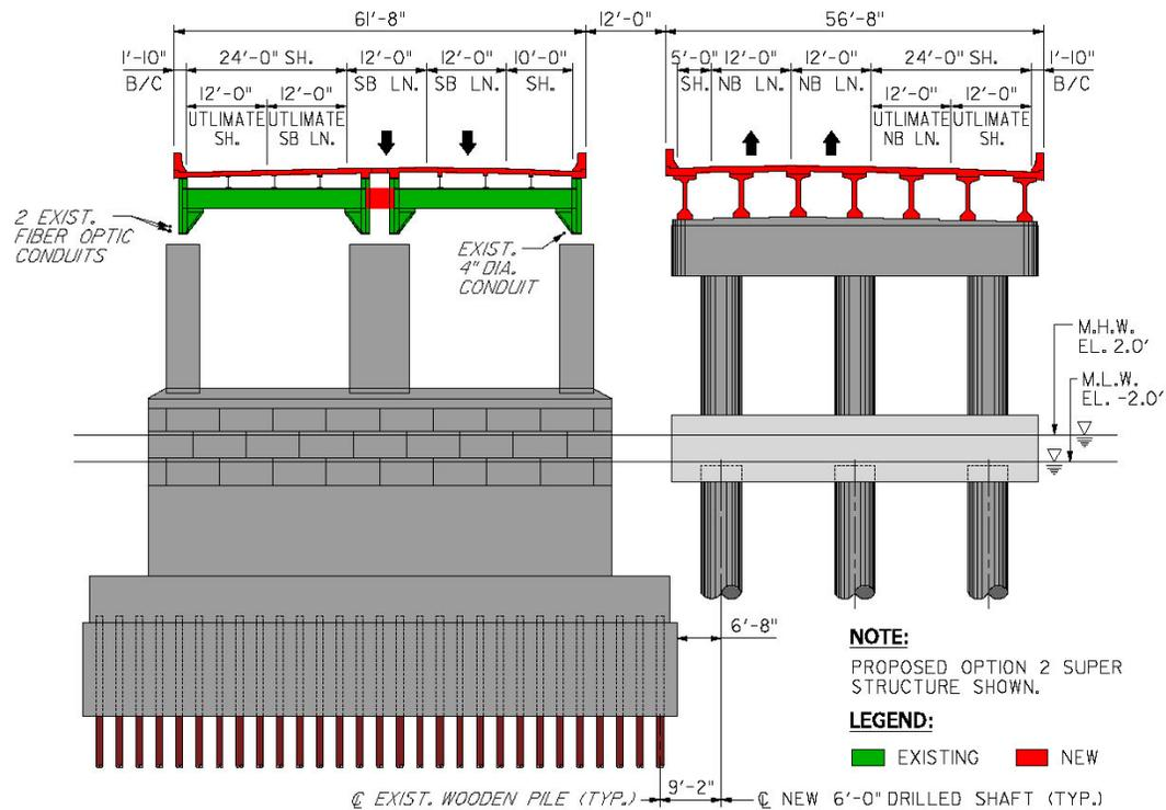
Figure 5 – Typical Bridge Section, Existing and Proposed Bridges
