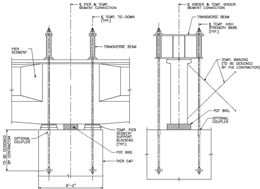
Figure 8 – Temporary Tie-down Details
