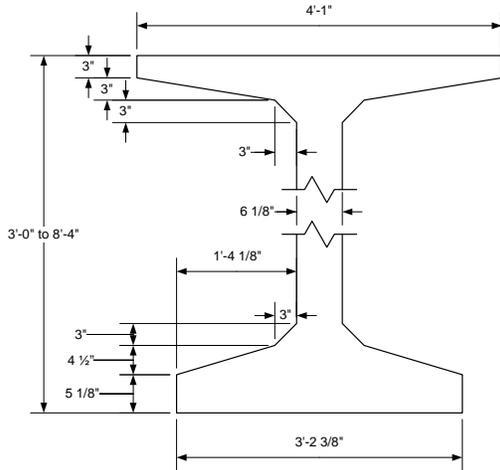
Figure 3 Typical Section for the WF-Series Girder
