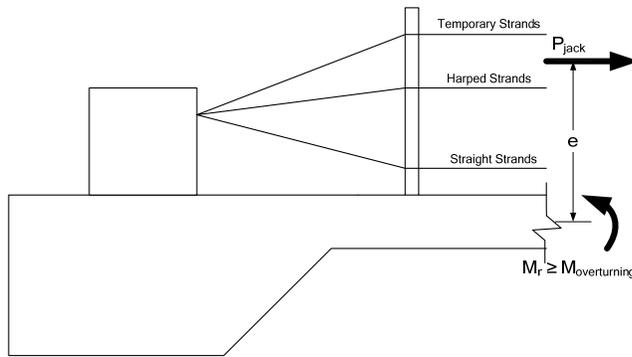
**Figure 1 Free Body Diagram of Critical Section of Prestressing Line**
