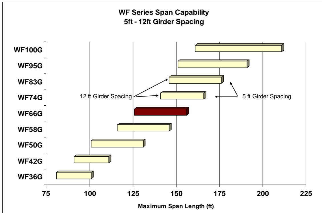
Figure 5 Span Capabilities of the WF-series Girders
