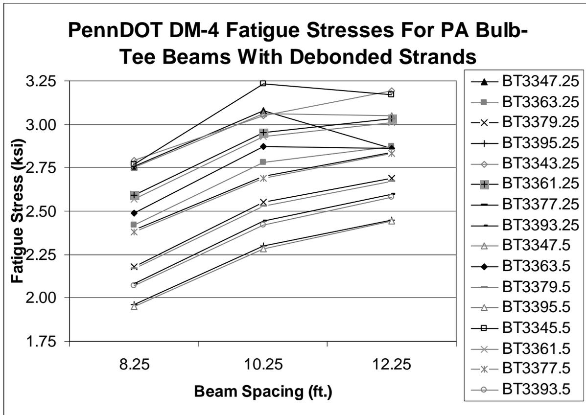
Figure 8 PennDOT DM-4 Fatigue Stresses for PA Bulb-tee Beams with Debonded Strands
