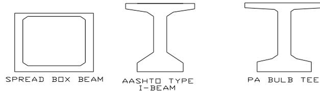
Figure 1. Typical Prestressed Girder Cross Sections
