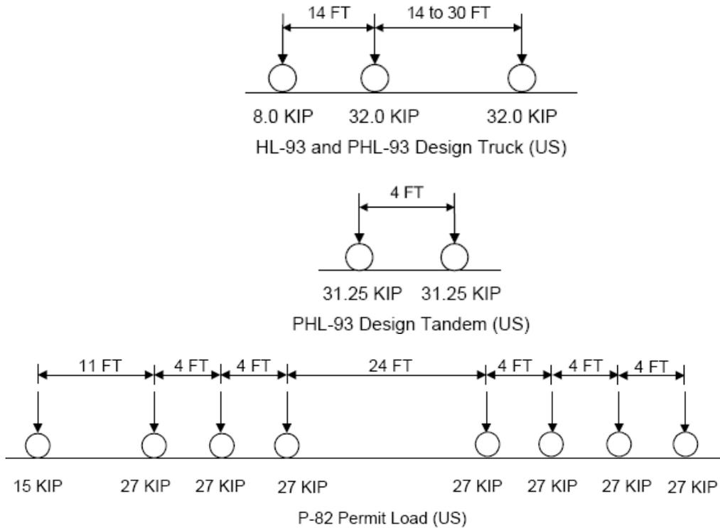
Figure 4. PennDOT Design Vehicles (Note: Superimposed uniform lane load of 0.64 kips/ft for the PHL-93 Design Truck and Tandem not shown)
