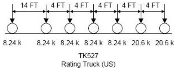
Figure 3. PennDOT TK527 Rating Vehicle
