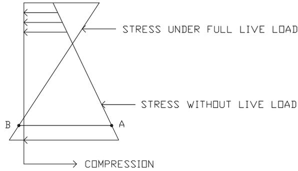
Figure 5. Stress Distribution along the Depth of a Prestressed Concrete Section (Level AB = CG of prestressing tendons; Trapezoidal distribution under dead loads; Triangular distribution under live loading plus dead loads; A to B represents a stress range)
