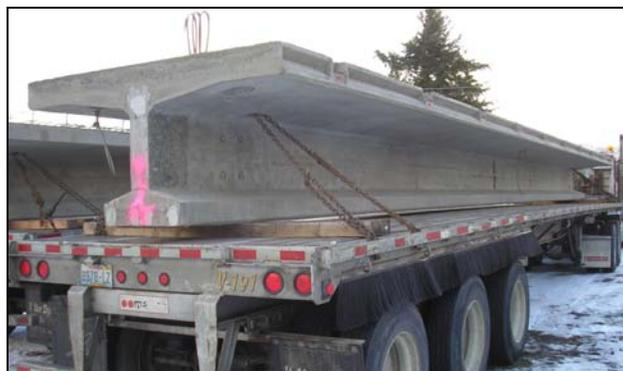
Fig. 8 Deck Bulb Tee Girder
