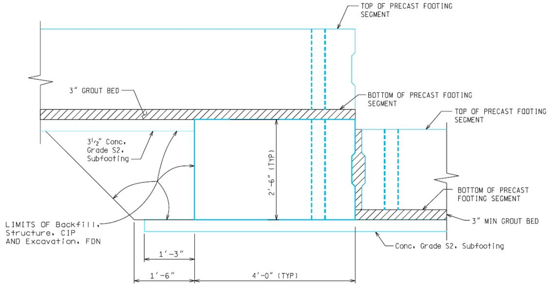
**Figure 5.** Precast Footing Block Elevation
