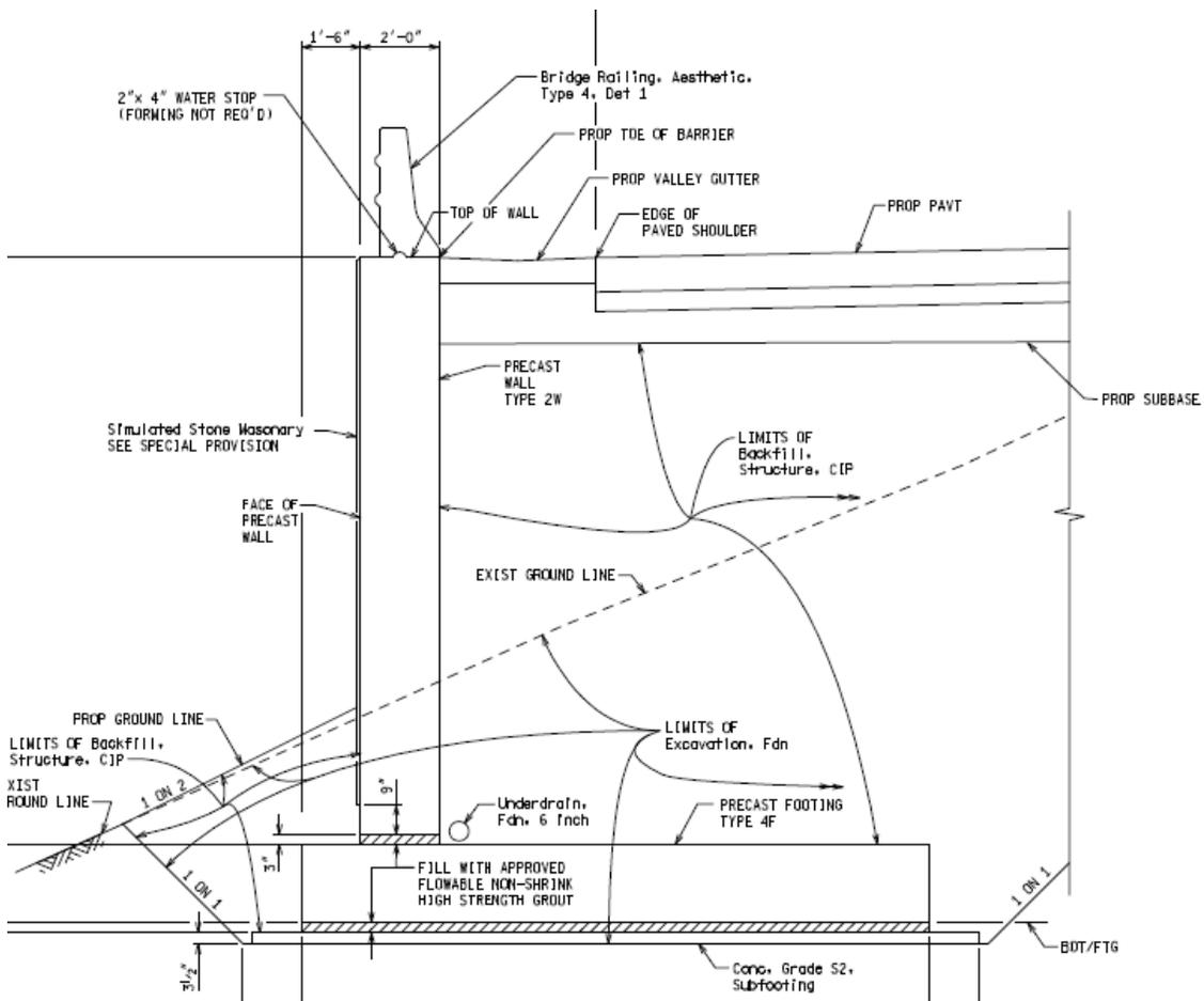
**Figure 2.** Precast Cantilever Retaining Wall System
