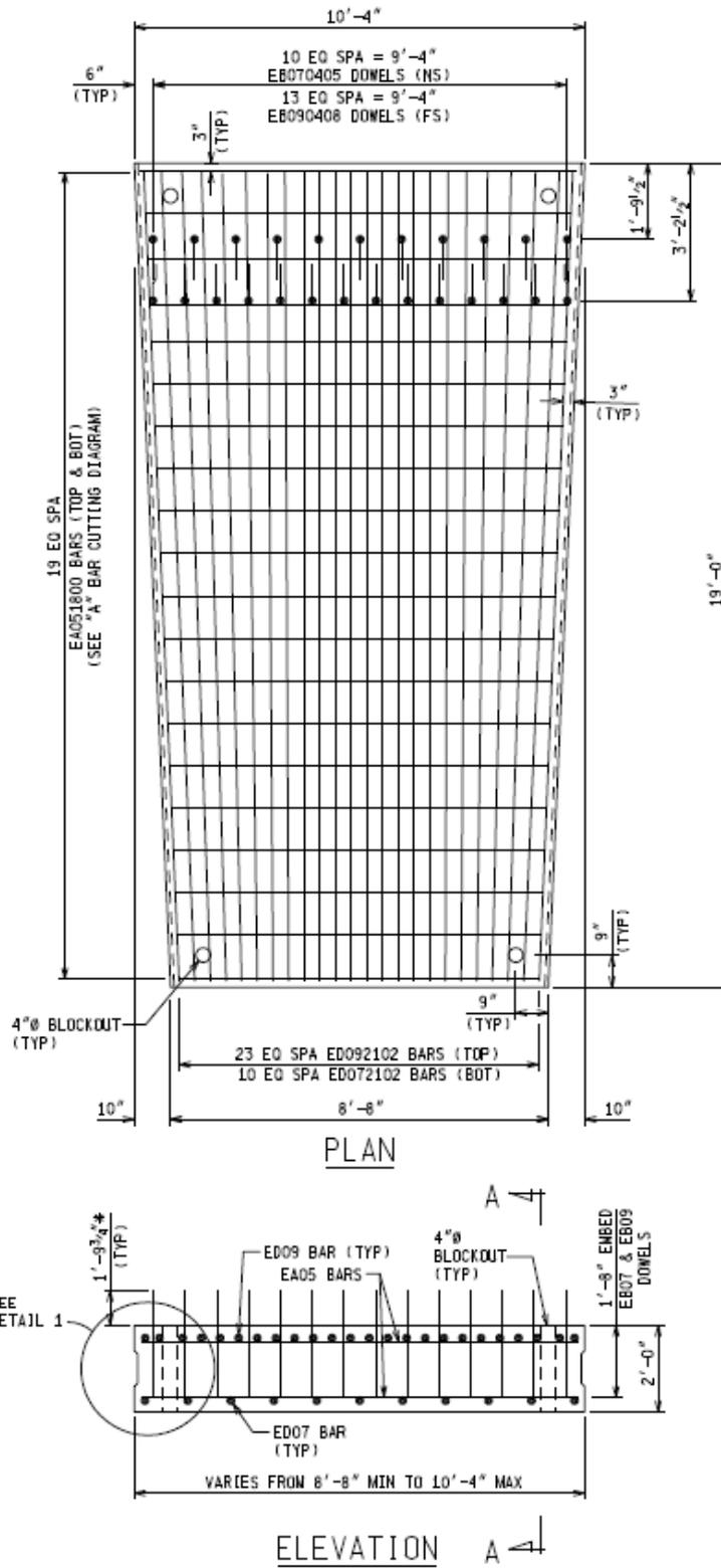
Figure 4. Trapezoidal Precast Footing Segment, Type 16 F
