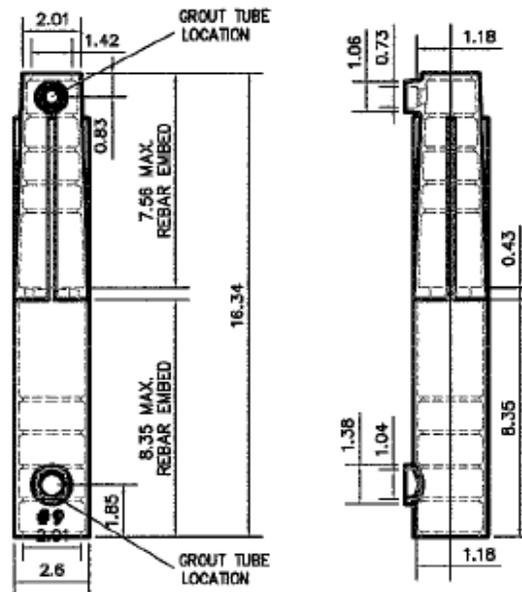
**Figure 7.** Grout Filled Mechanical Splicer for # 9 bars
