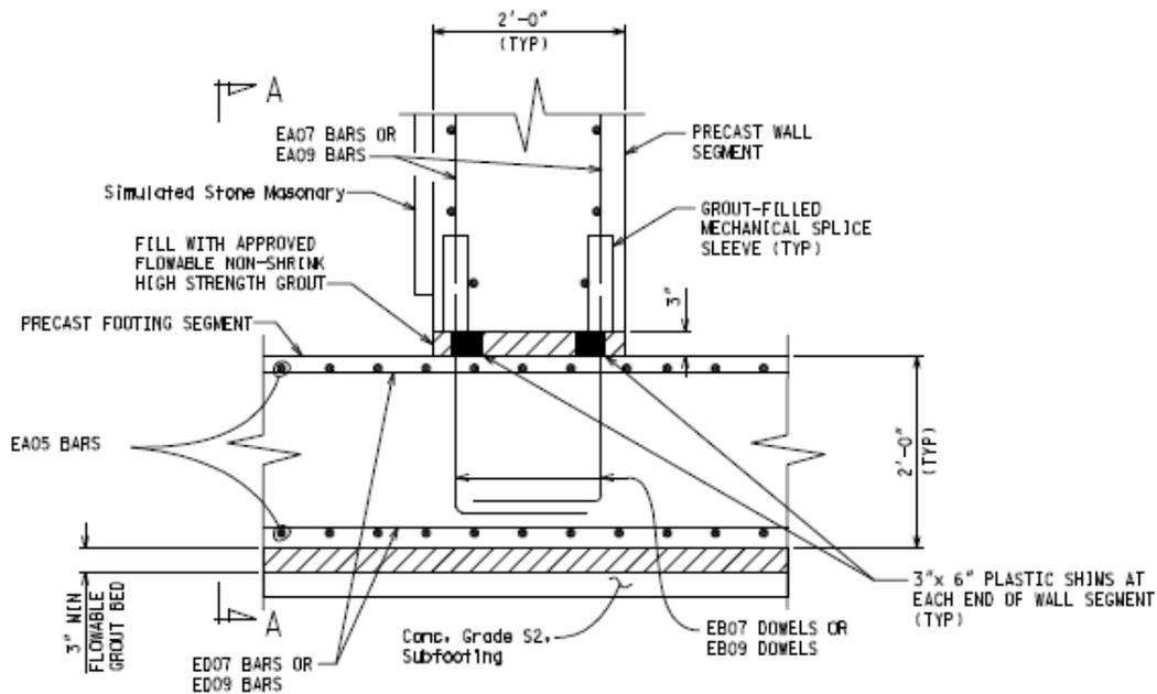
**Figure 3.** Typical Wall Segment-to-Footing Segment Connection
