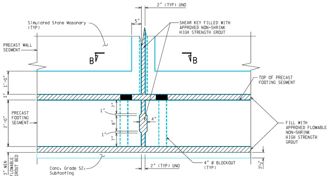
**Figure 8.** Vertical Shear Keys Detail
