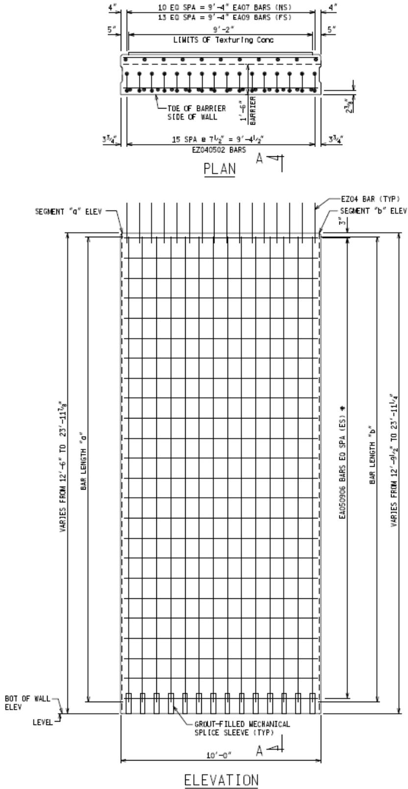
Figure 6. Precast Wall Stem Segment, Type 3 W
