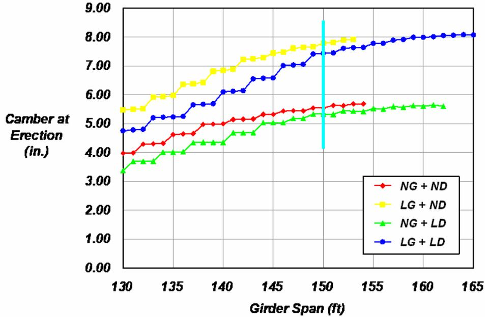
Fig. 10 Camber at erection with increasing span – 10 ft girder spacing
