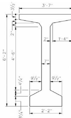
Fig. 1 Dimensions of 74-in. Deep Modified Bulb-Tee Girder Section
