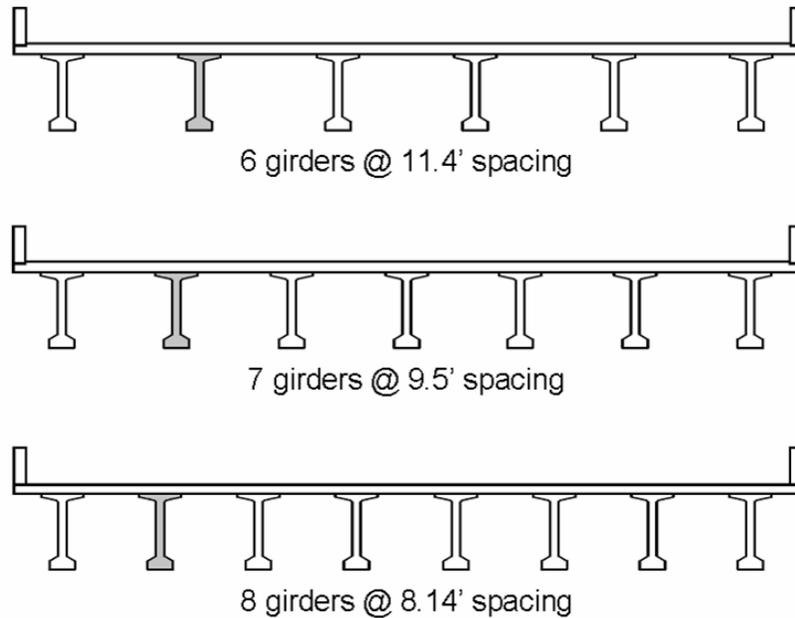
Fig. 3 Three typical sections considered for maximum span designs
