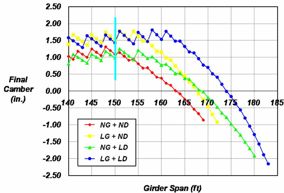
Fig. 12 Final camber with increasing span – 8 ft girder spacing
