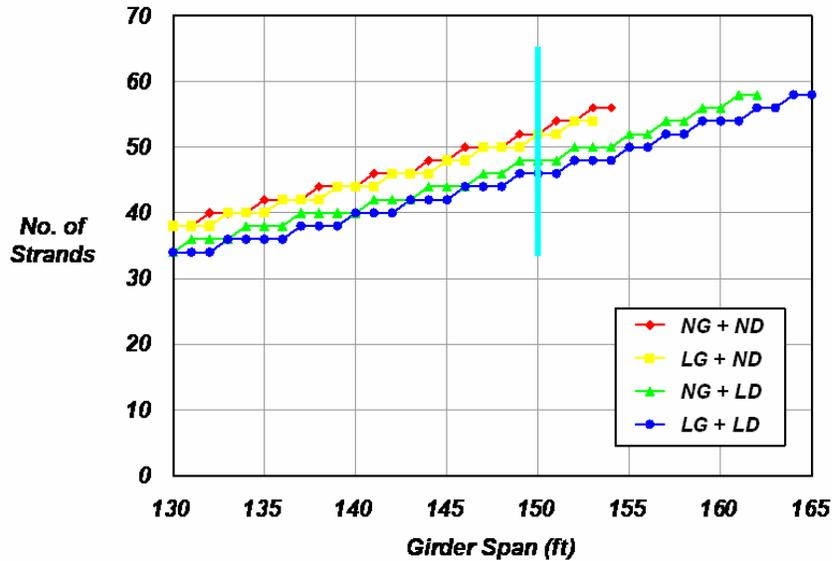
Fig. 8 Required number of strands with increasing span – 10 ft girder spacing
