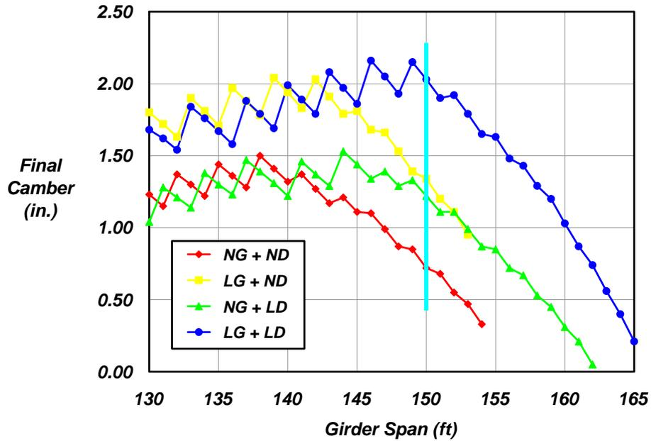
Fig. 11 Final camber with increasing span – 10 ft girder spacing
