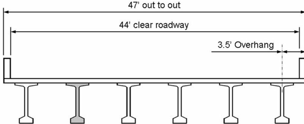
Fig. 6 Typical section for fixed span designs
