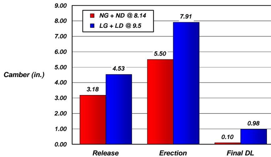
Fig. 5 Comparison of cambers for girder designs with 162 ft maximum spans
