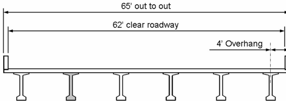
Fig. 2 Typical section for maximum span designs
