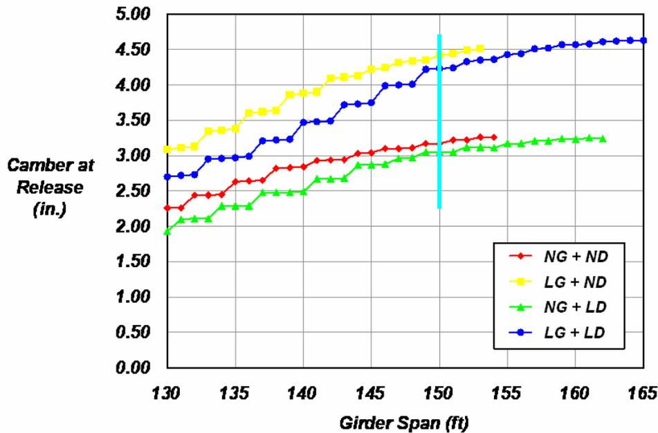
Fig. 9 Camber at release with increasing span – 10 ft girder spacing
