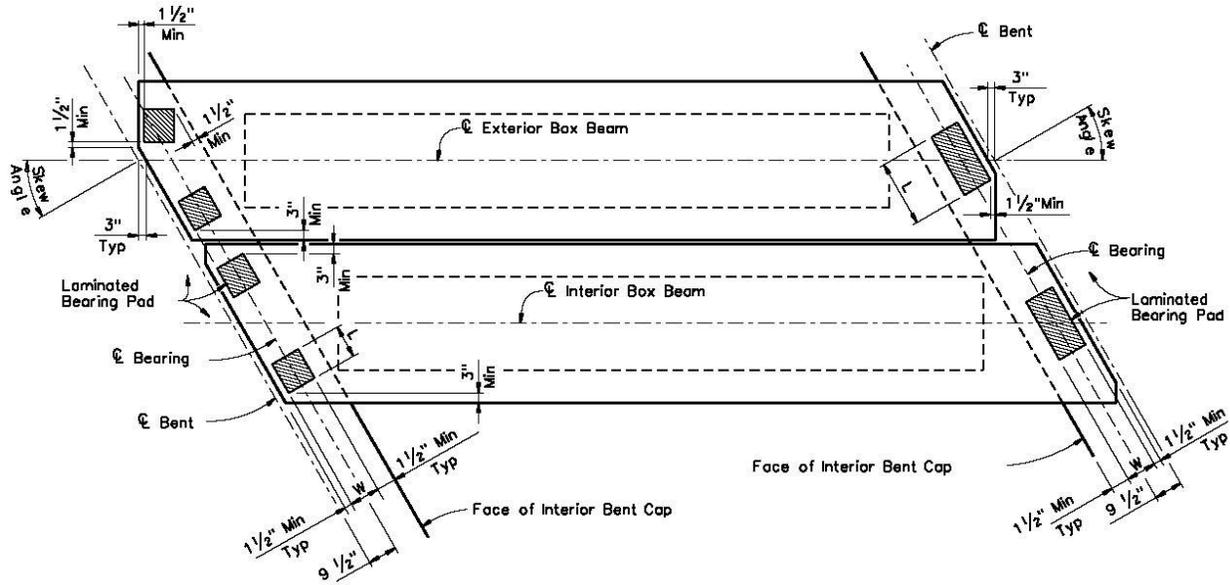
Figure 2: Plan of two adjacent boxes of the NASA Road 1 bridge in Texas (PCI 2007)
