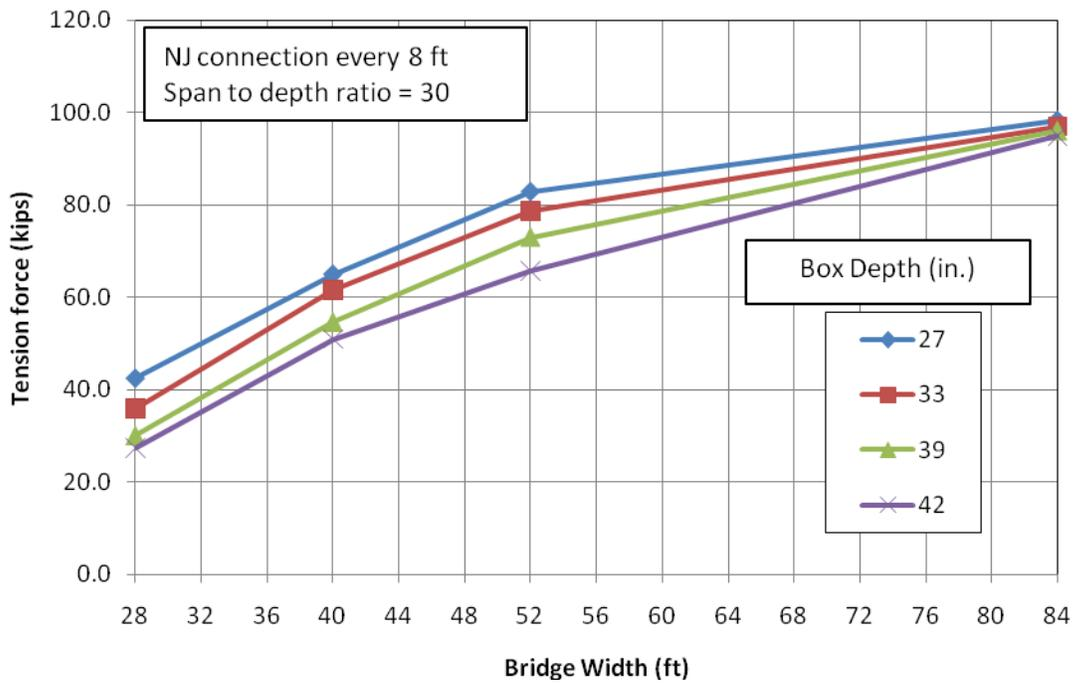
**Figure 11 Effect of box depth and bridge width on the required transverse tension force (kips) for the NJ system**
