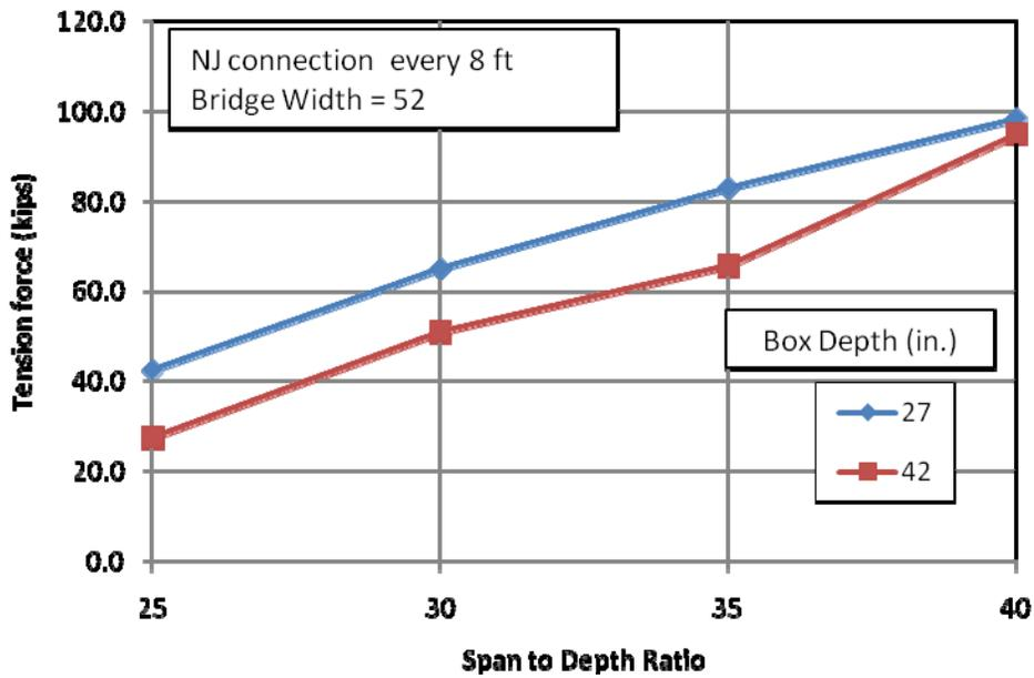
**Figure 14 Effect of span-to-depth ratio on the required factored transverse tension force (kips) for NJ system**
