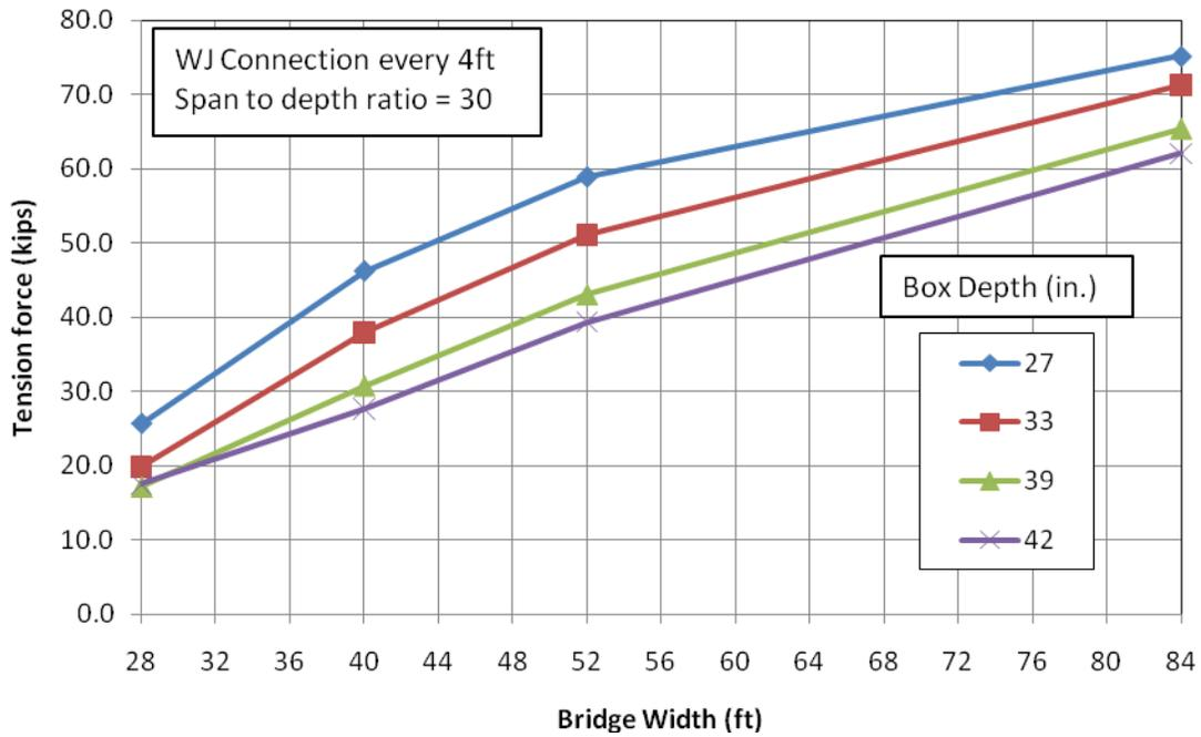
**Figure 10 Effect of box depth and bridge width on the required transverse tension force (kips) for the WJ system**
