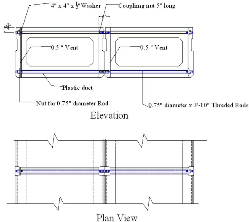
Figure 8 NJ Connection detail
