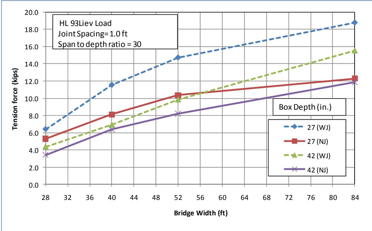
**Figure 12 Comparing the tension force (kip/ft) required for the WJ and NJ systems**
