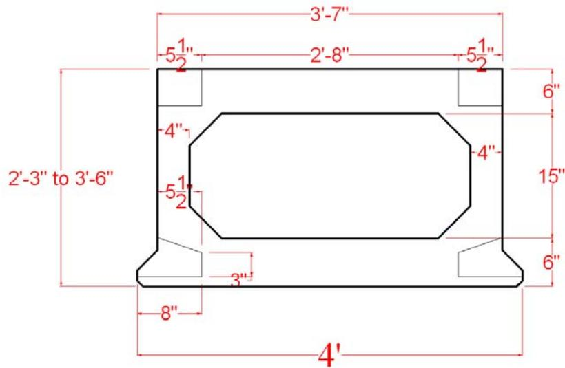
Figure 5 WJ System Box Dimensions
