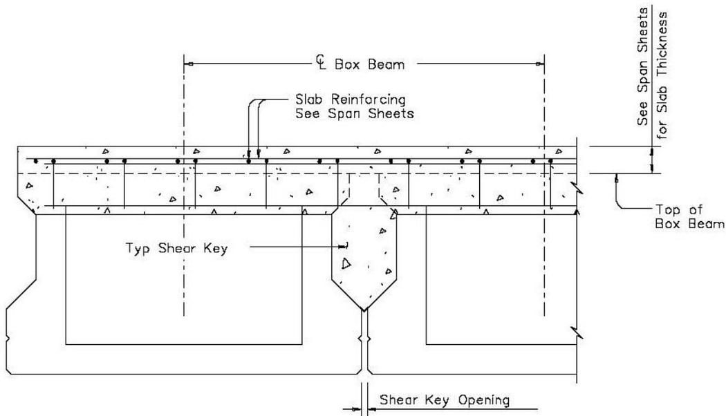
Figure 3: Cross section of transverse connection of the NASA Road 1 bridge in Texas (PCI 2007)
