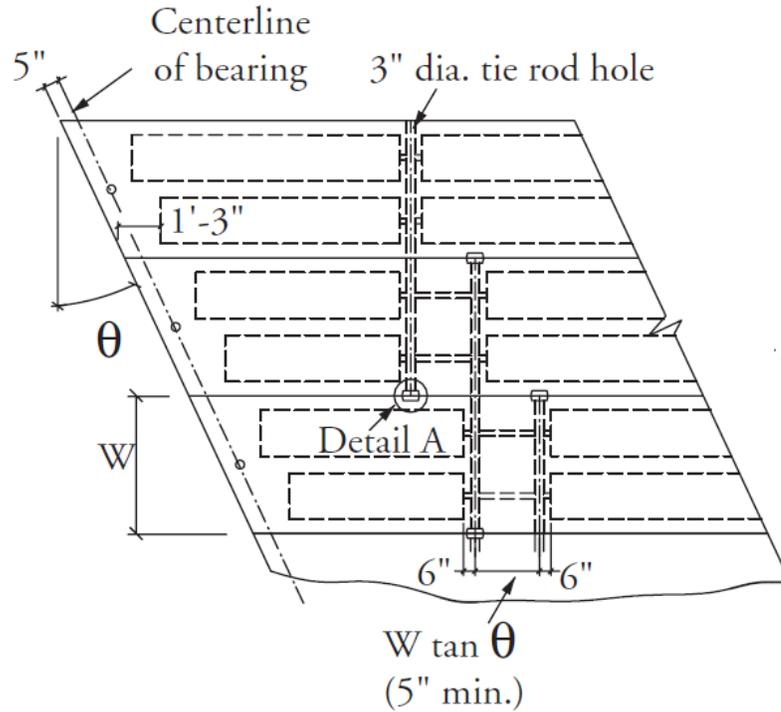
Figure 1: Post-tensioning of a skewed bridge (PCI 2003)
