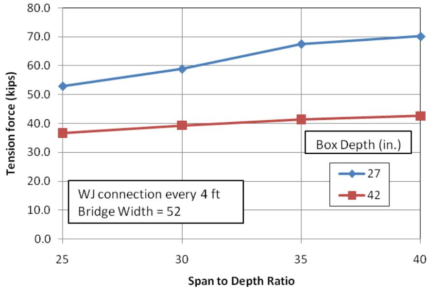
**Figure 13 Effect of span-to-depth ratio on the required transverse tension force (kips) for the WJ System**
