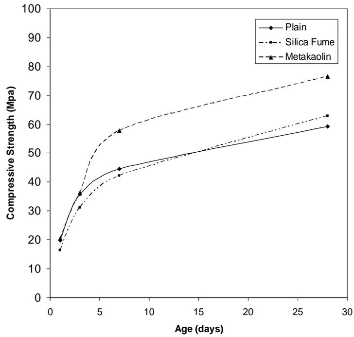
Fig. 4 Variation of Compressive Strength with Age for Concrete
