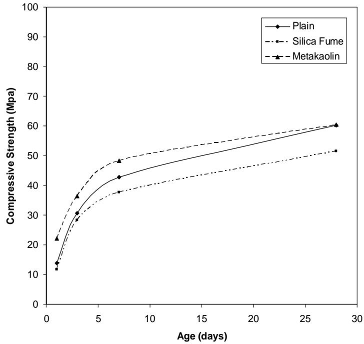
Fig. 2 Variation of Compressive Strength with Age for Paste
