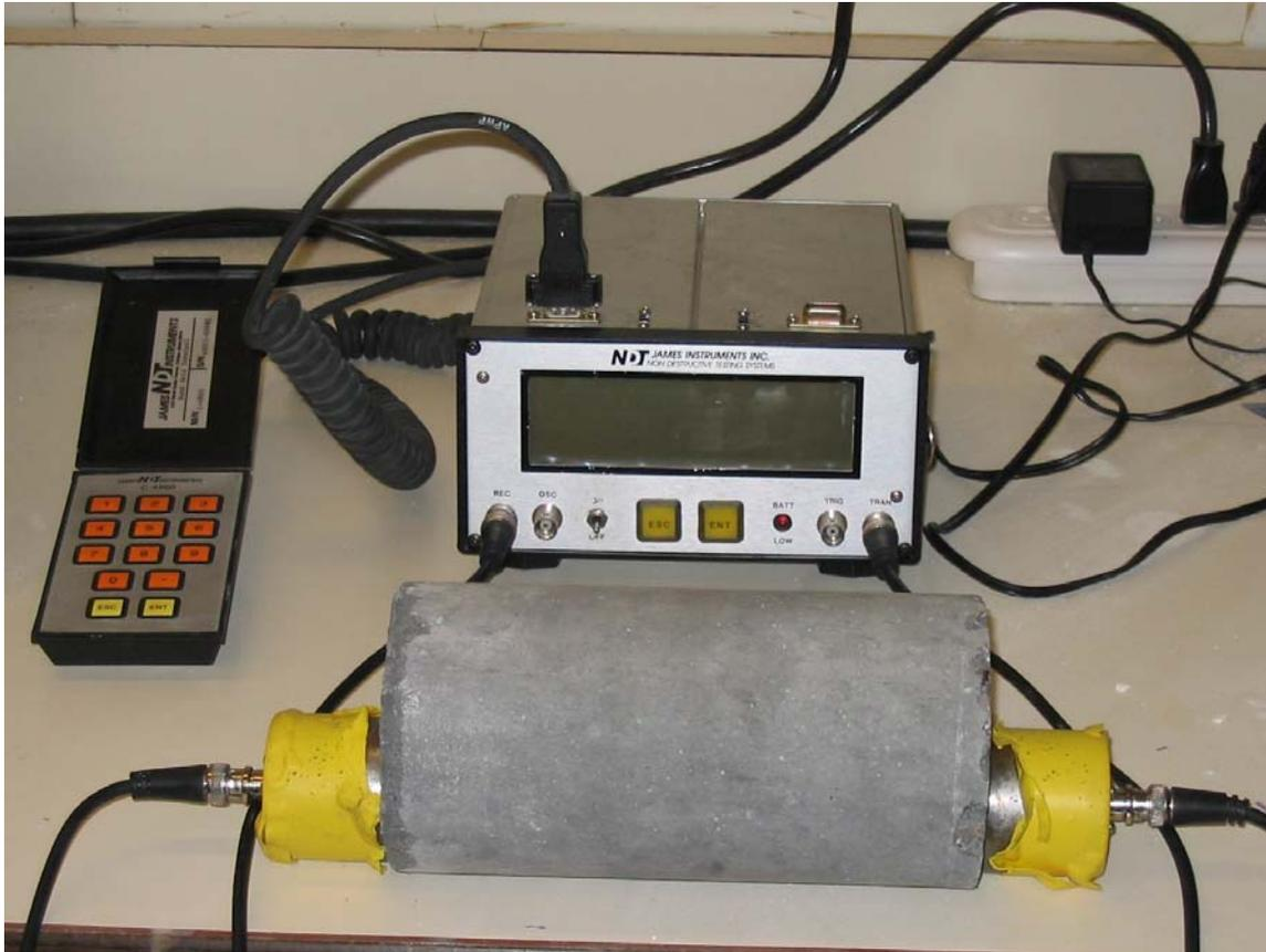
Fig. 1 Experimental Set-up for Ultrasonic Pulse Velocity Testing
