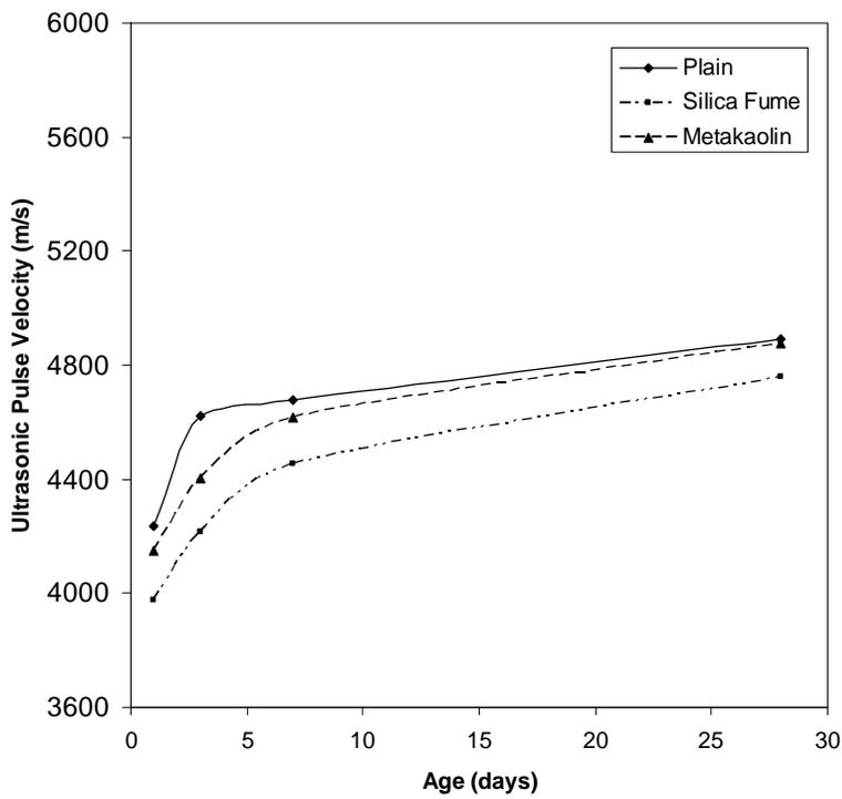
Fig. 7 Variation of Ultrasonic Pulse Velocity with Age for Concrete
