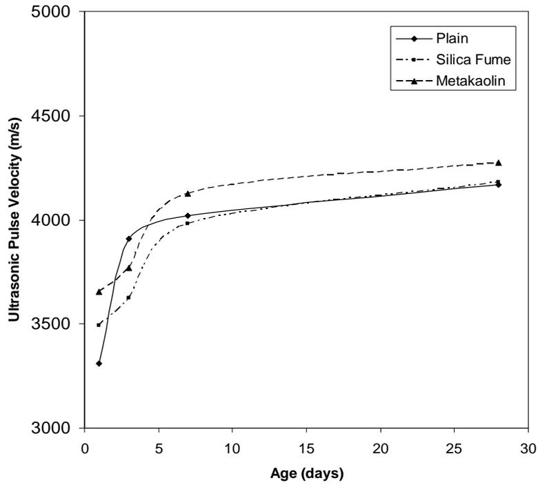
Fig. 6 Variation of Ultrasonic Pulse Velocity with Age for Mortar
