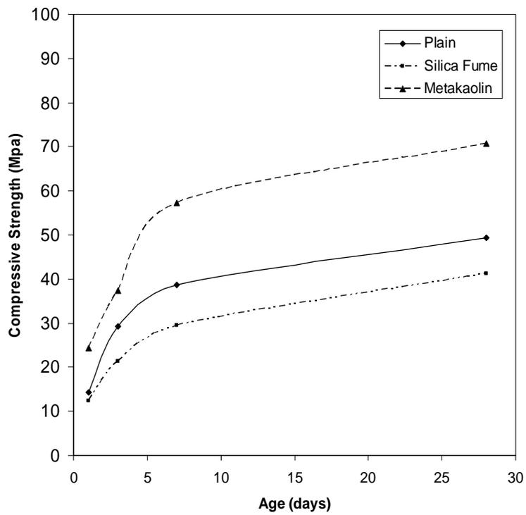
Fig. 3 Variation of Compressive Strength with Age for Mortar
