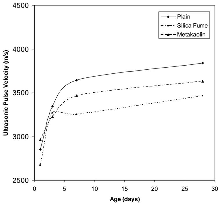
Fig. 5 Variation of Ultrasonic Pulse Velocity with Age for Paste
