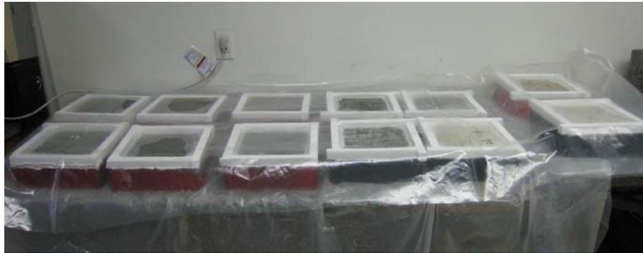
Figure 3 Ponding of Specimens
