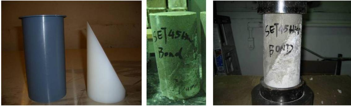
(a) Test Mold and Dummy Section (b) Completed Slant Shear Cylinders (c) Test Setup
