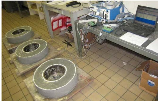
Figure 10 AASHTO PP34 Test Setup
