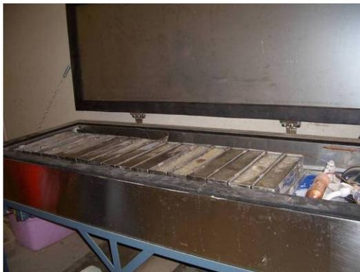
(a) Freezing-and-Thawing Apparatus
