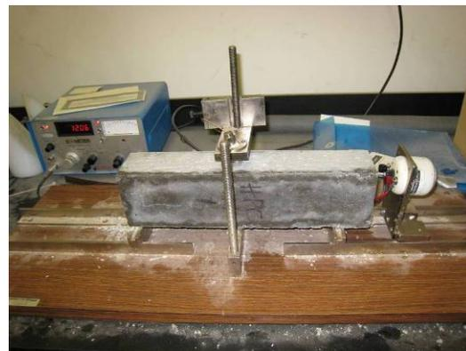
(b) Fundamental Transverse Frequency Test
