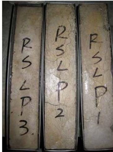
Figure 9 Failure of RSLP Mix 2 Specimens
