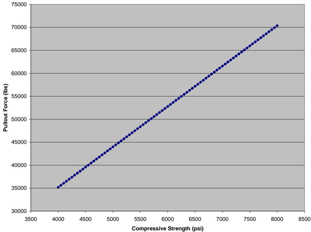
**Fig. 2 Design Pullout Load for Varying Compressive Strengths**
