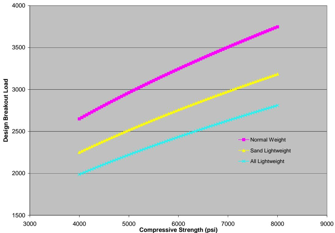
**Fig. 1 Design Breakout Load (lbs) for Varying Compressive Strengths**
