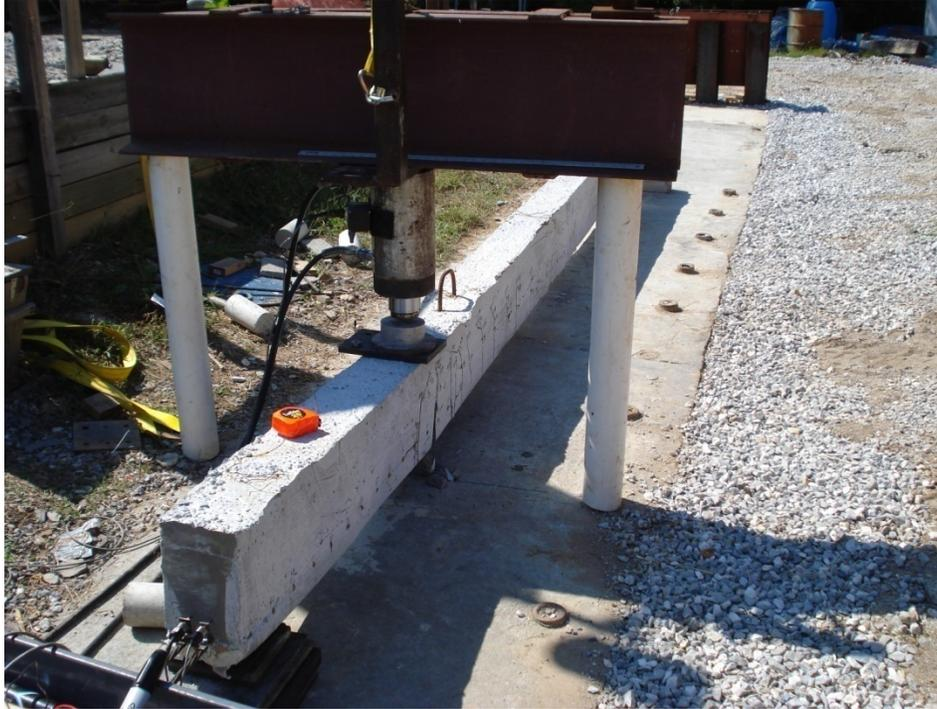
Fig. 4 Instrumented beam after failure
