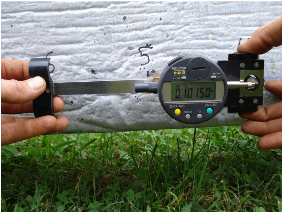
Fig. 2 DEMEC Target Strain Gauge
