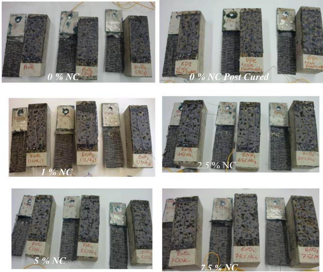
Fig. 10: Failure mode of testing single-lap shear samples at elevated temperature
