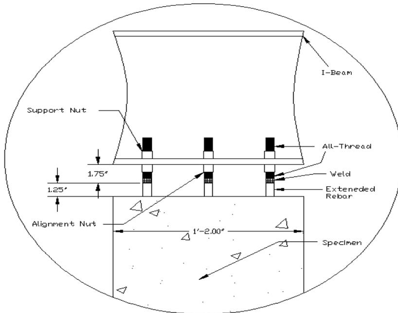
Figure 7: Testing Setup for Transverse Joint
