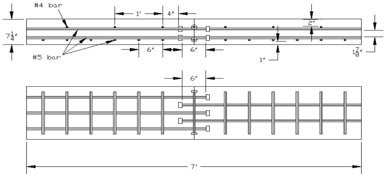
Figure 5: Headed bar Transverse Joint Specimen
