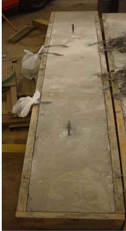
Figure 14: Completed Flexural Specimen
