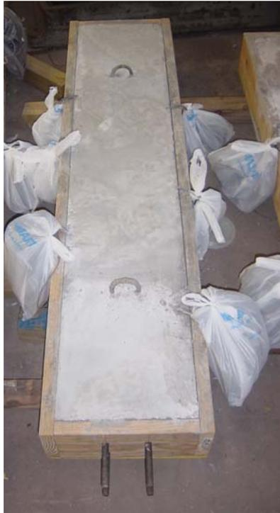
Figure 13: Completed Tension Specimen
