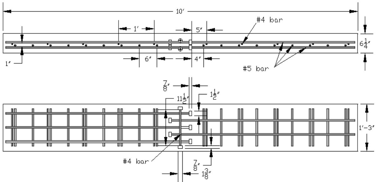
Figure 3: Headed bar Longitudinal Joint Specimen
