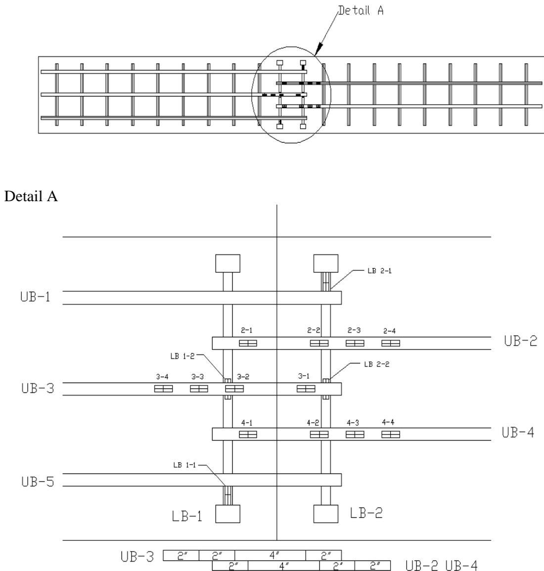
**Figure 8: Strain Gage Configuration in u-bar Detail**
