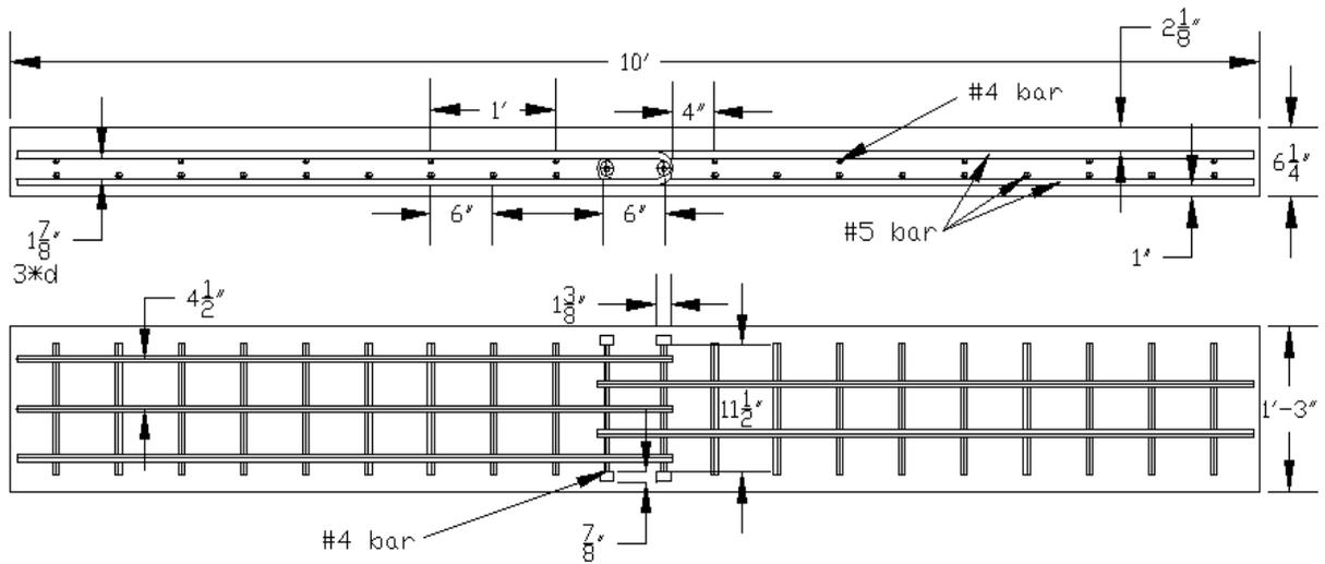
Figure 2: U-bar Longitudinal Joint Specimen
