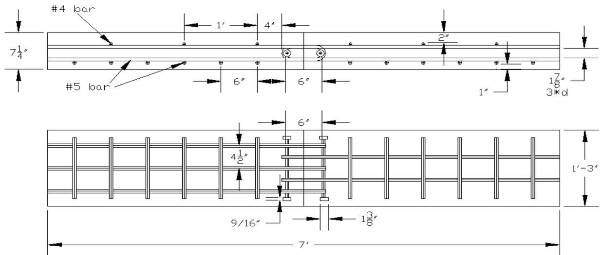
Figure 4: U-bar Transverse Joint Specimen
