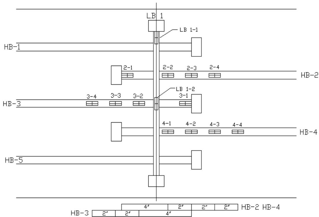
Figure 9: Strain Gage Configuration in Headed Bar Details
