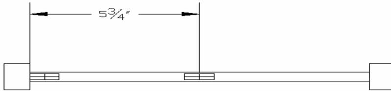
Figure 10: Strain Gage Placement on Lacer Bars
