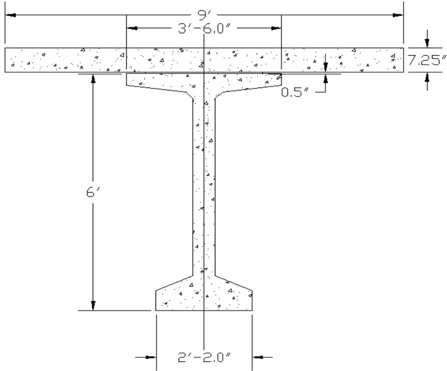
Figure 1: Section Used for Negative Moment Longitudinal Reinforcement Calculation
