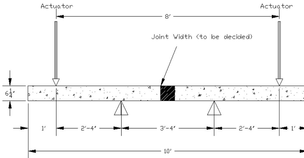
Figure 6: Testing Setup for Longitudinal Joint
