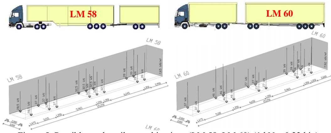
Figure 5: Possible truck-trailer combinations (LM 58, LM 60) ( $1 \text{ kN} \approx 0,22 \text{ kip}$ )
