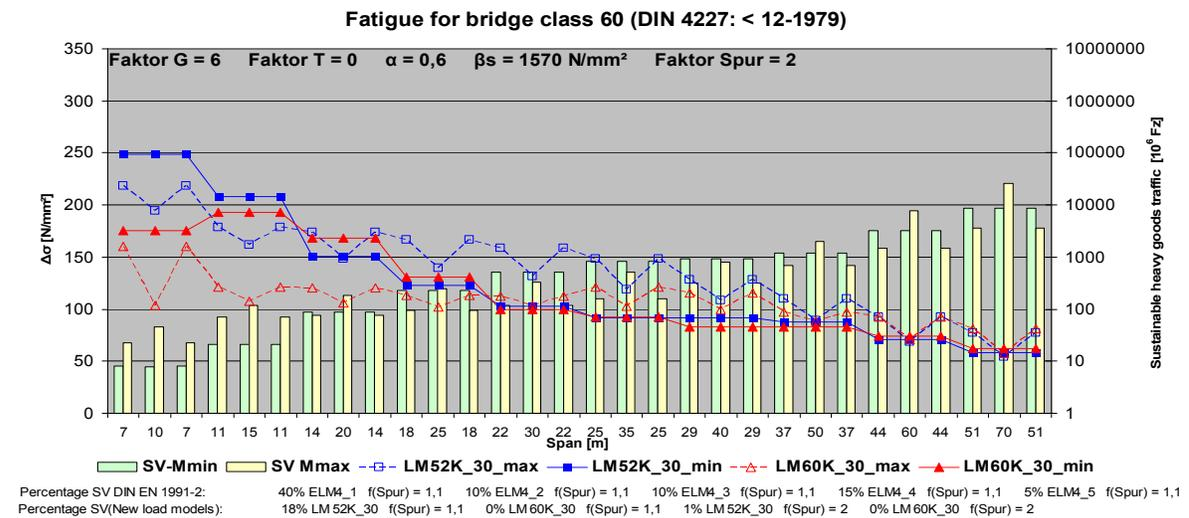
Figure 16:  $\Delta\sigma$  from comparisons of the “new” load models with bridge class 60 (DIN 4227: < 12-1979) (1 m  $\approx$  3,28 ft, 1N/mm<sup>2</sup>  $\approx$  0,145 ksi)
