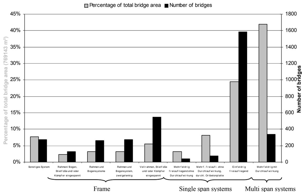
Figure 12: Static systems in longitudinal direction
