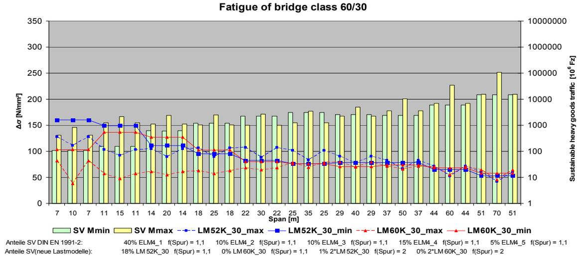
Figure 14:  $\Delta\sigma$  from the comparison of “new” load models with bridge class 60/30 (1 m  $\approx$  3,28 ft, 1N/mm<sup>2</sup>  $\approx$  0,145 ksi)
