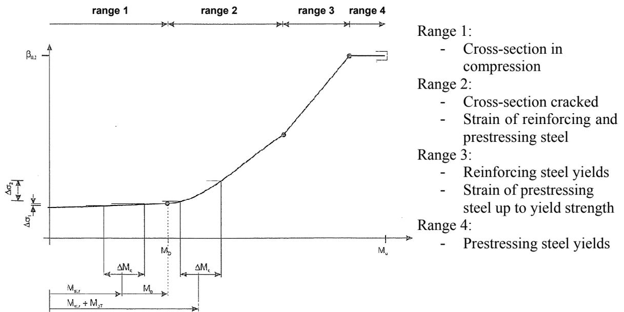
Figure 8:  $M - \sigma_z$  correlation of prestressing steel reinforcement from [27]
