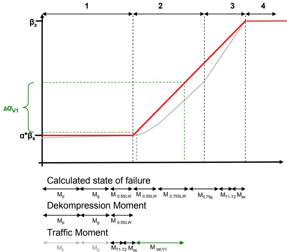
Figure 9: Modified  $M - \sigma_z$  correlation (limited prestressing)
