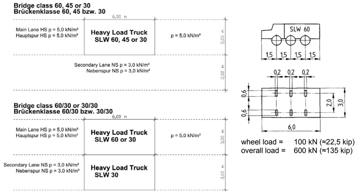
Figure 2: Schematic representation of German bridge classes, plan view
