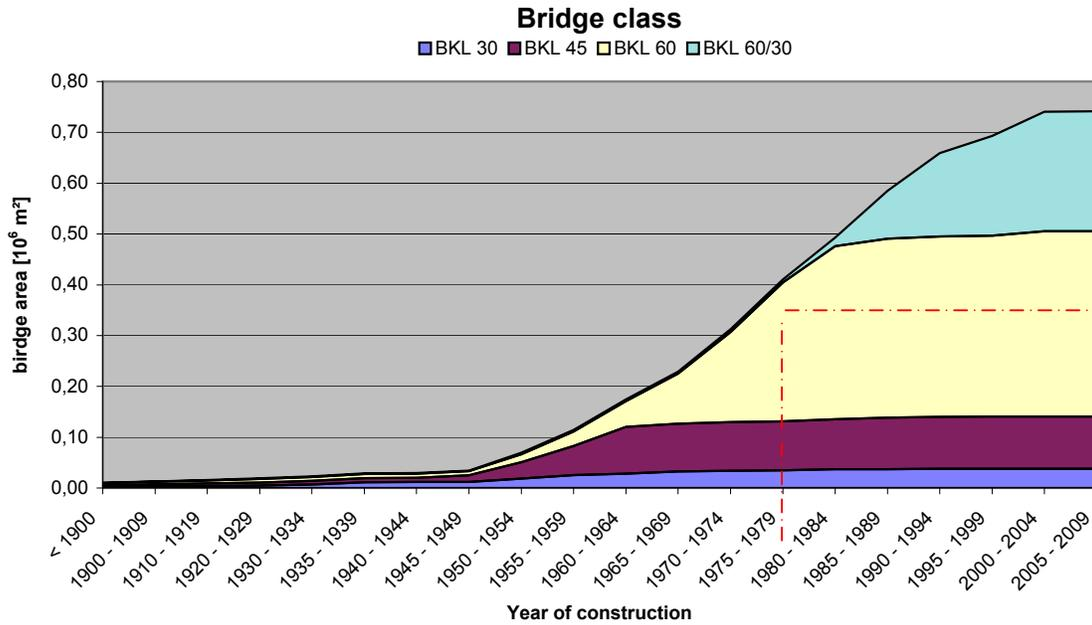
Figure 4: Trend in total bridge area ( $1 \text{ m}^2 \approx 10,76 \text{ ft}^2$ )
