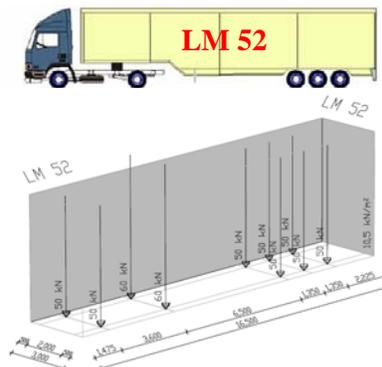
Figure 6: Possible truck-trailer combinations (LM 52) ( $1 \text{ kN} \approx 0,22 \text{ kip}$ )
