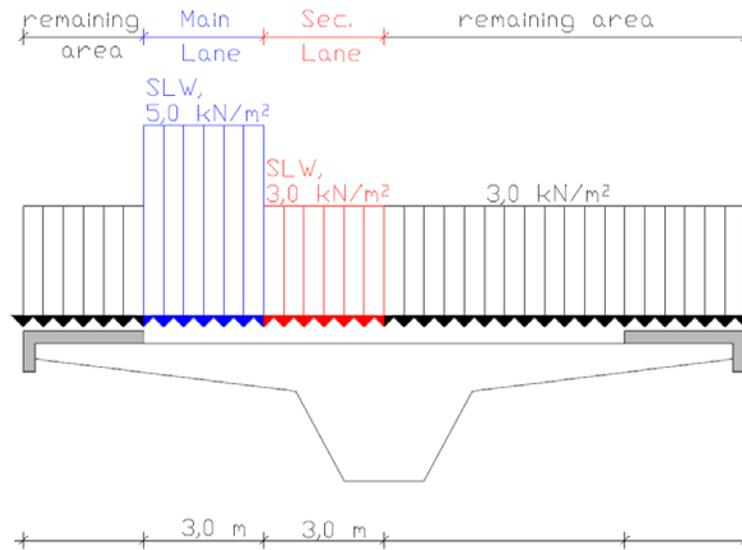
Figure 3: Schematic representation of German bridge classes, cross section
