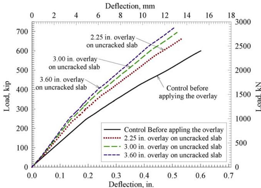
Fig. 3 Load-deflection curve for each model generated from the nonlinear FEA
