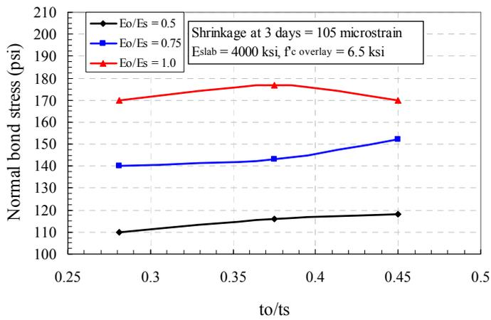
Fig. 9 Induced normal bond stress for shrinkage of 105 microstrain
