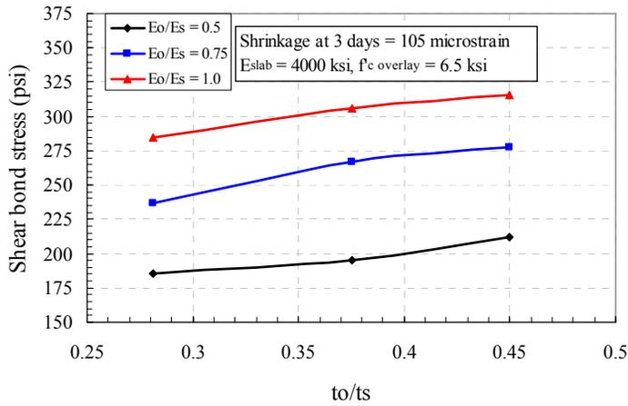
Fig. 8 Induced shear bond stress for shrinkage of 105 microstrain
