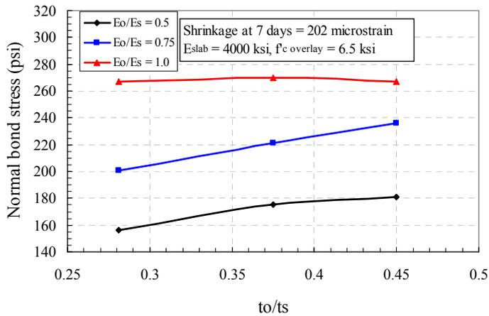
Fig. 11 Induced normal bond stress for shrinkage of 202 microstrain
