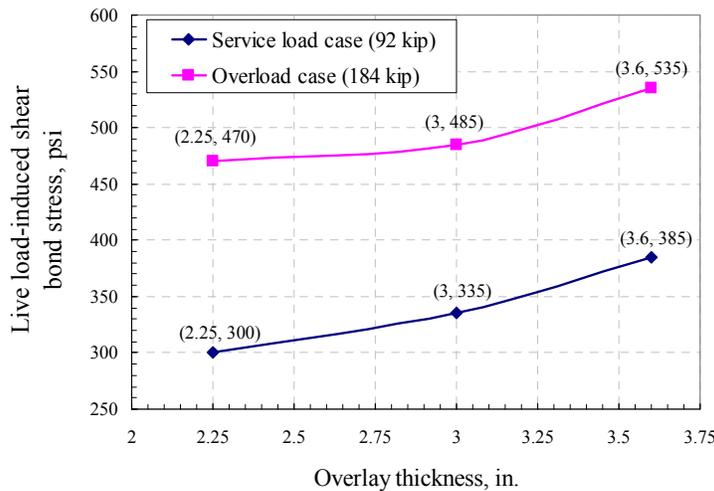
Fig. 5 Overlay thickness versus the maximum live load-induced shear bond stress
