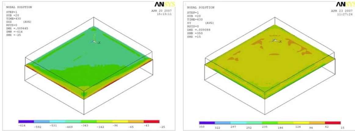
Fig. 7 Typical shear (left) and normal (right) bond stress contours ( $t_o/t_s=0.281$ ,  $E_o/E_s=1$ )
