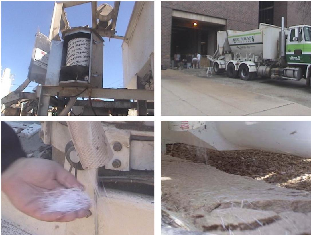
Fig. 2 The new fiber feeder system<sup>4</sup>
