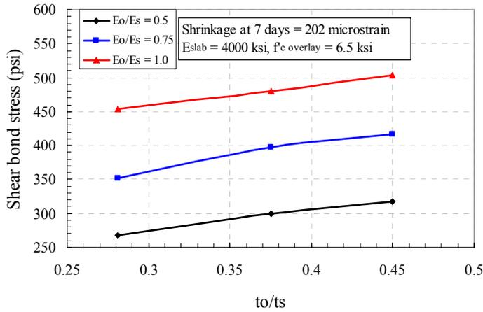
Fig. 10 Induced shear bond stress for shrinkage of 202 microstrain
