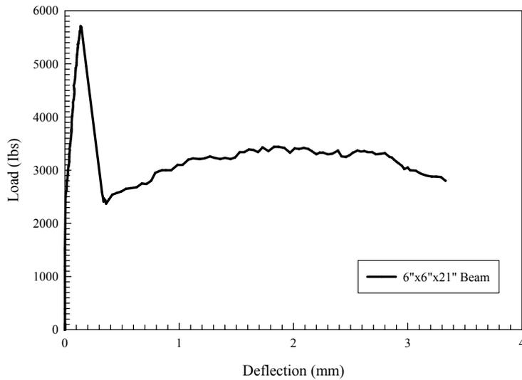
Fig. 1 Load-deflection curve for the fibrous LMC overlay<sup>1</sup>
