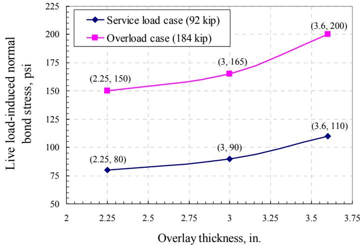
Fig. 4 Overlay thickness versus the live load-induced normal bond stress
