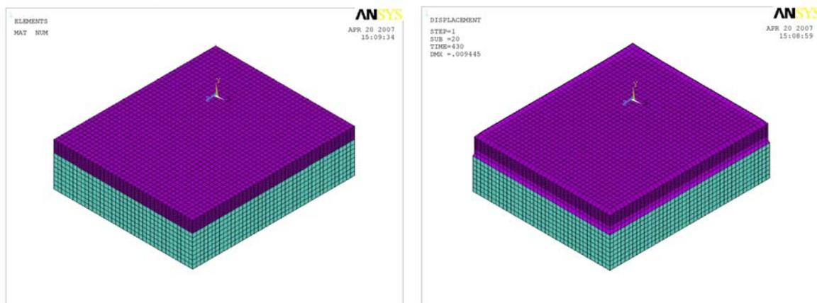
Fig. 6 Meshing of the overlay and slab in the FEA models and typical deformed shape
