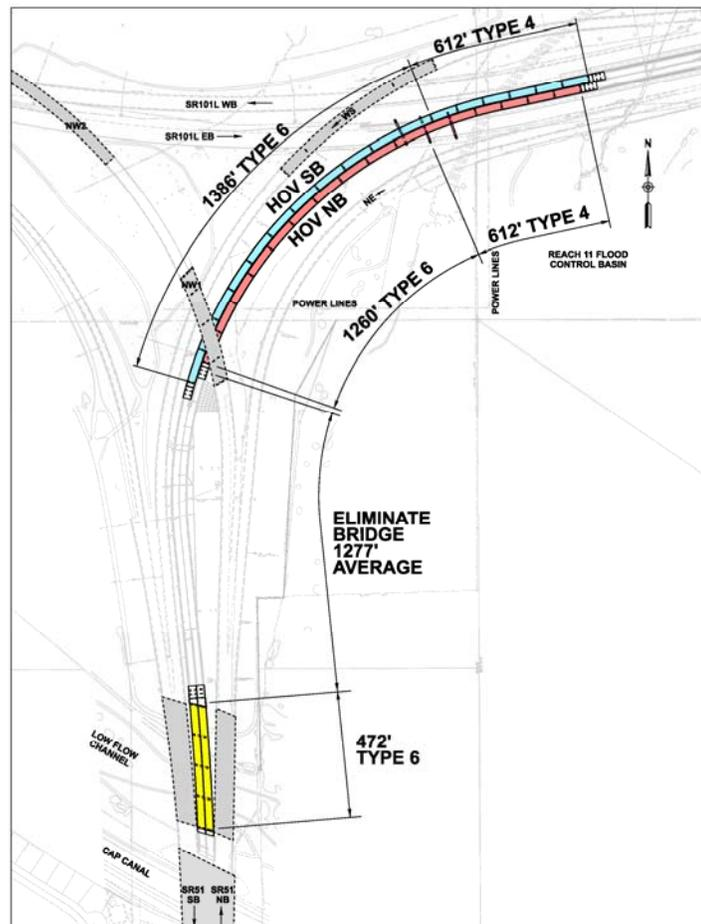
**Figure 04** – Cost savings estimated at \$5.5-million was achieved by eliminating over 80,000 square feet of bridge.
