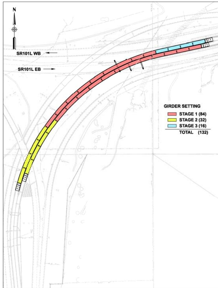
**Figure 13** – 132 Girders set in three mobilizations.
