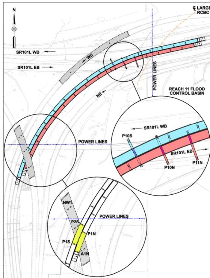
**Figure 09** – Of the many constraints, perhaps the top two are (1) passage under existing Ramp NW bridge with no substructure underneath; and (2) passage over SR101L EB with three cleverly designed straddle bents.
