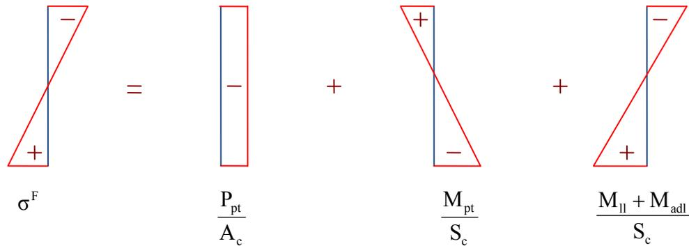
Fig. 4 Concrete Stress Distribution in Composite Section – Final
