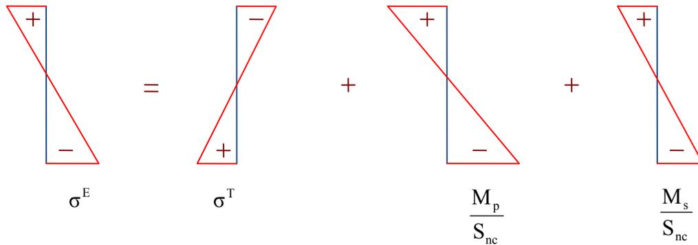
Fig. 2 Concrete Stress Distribution in Girder at Propping Location – During Erection
