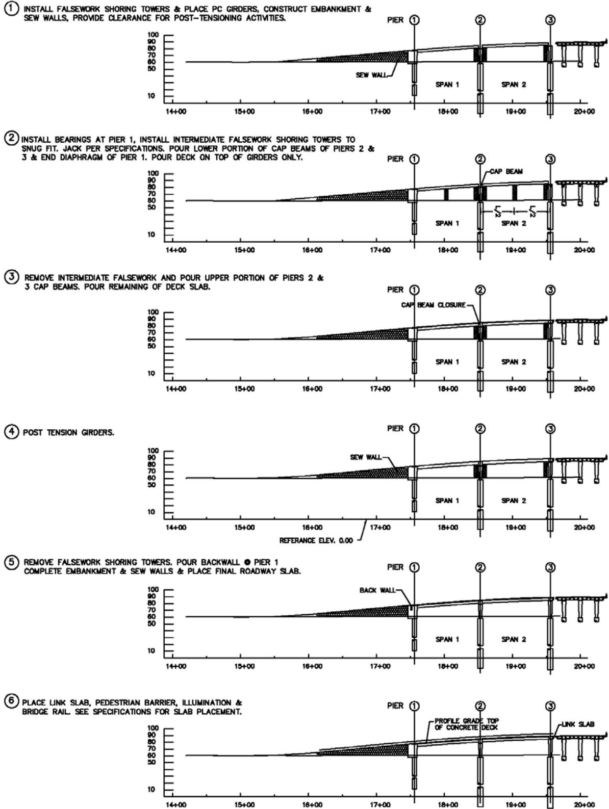
Fig. 6 Construction Sequence of the Pacific Avenue Overcrossing
