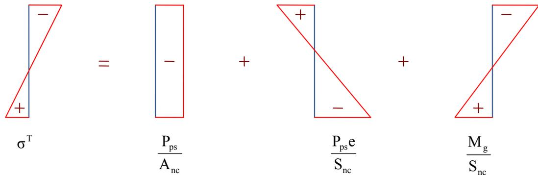
Fig. 1 Concrete Stress Distribution in Girder – During Transportation
