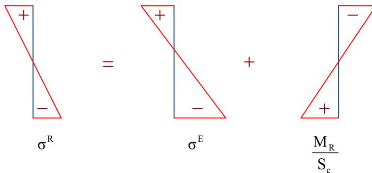
Fig. 3 Concrete Stress Distribution in Girder – Removal of Propping Stage
