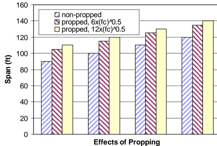
Fig. 15 Effects of Propping and Increasing Maximum Allowable Tensile Stress on Span Length
