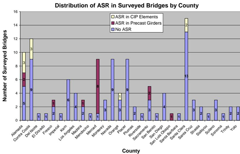
Figure 7. ASR occurrence in the surveyed bridges by county.
