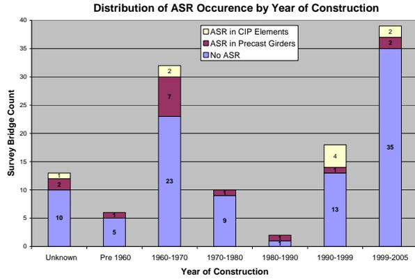
Figure 6. ASR occurrence in the surveyed bridges by year of construction.
