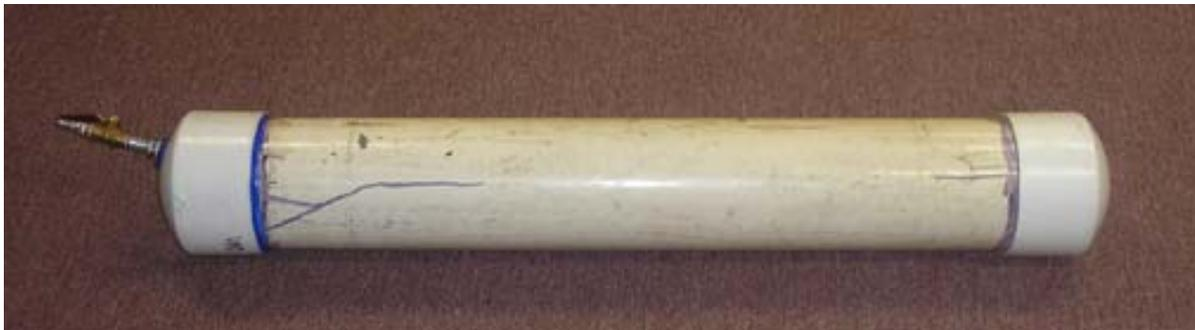
**Fig 7 21.7 Liter Calibration Cylinder for Void Measuring Equipment (VME)**
