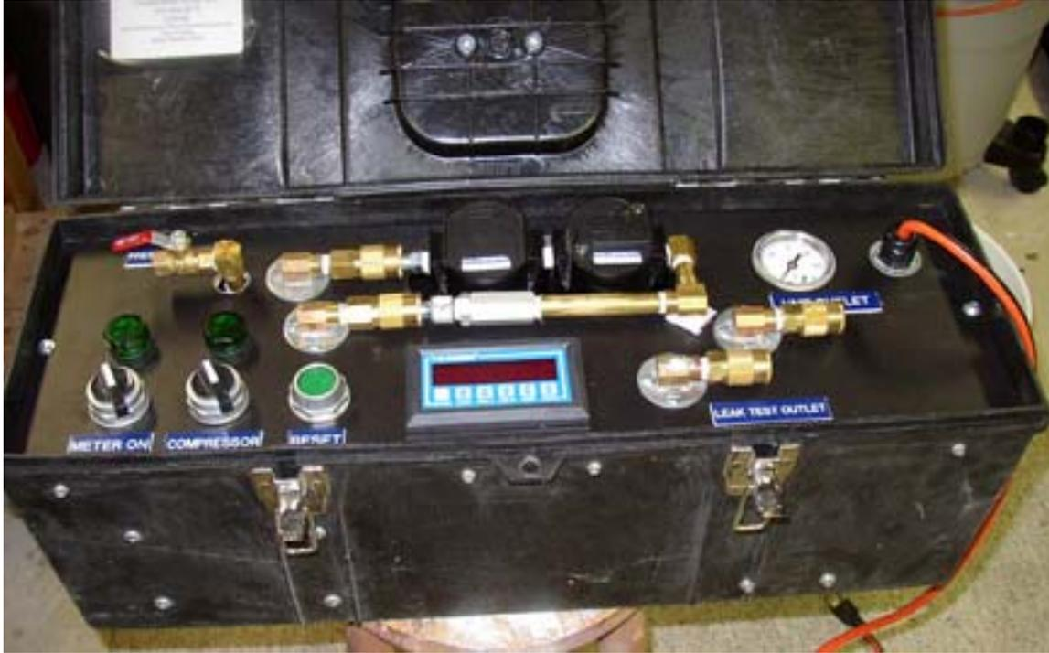
**Fig 8. Forensic Void Measuring Equipment- contains system for pressurizing and detecting leaks**
