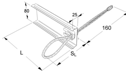
Picture 2: Connecting Loop (metal version)
