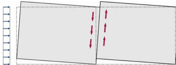
Picture 8: Shear forces parallel to the joint
