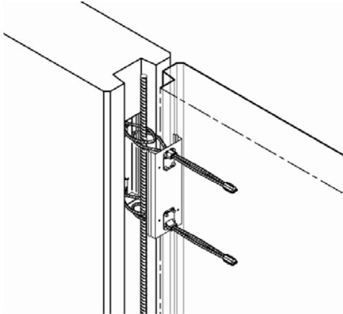
Picture 1: Cross Section of Philipp Power Box
