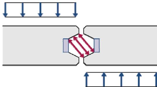
Picture 9: Shear forces at right angles to the joint
