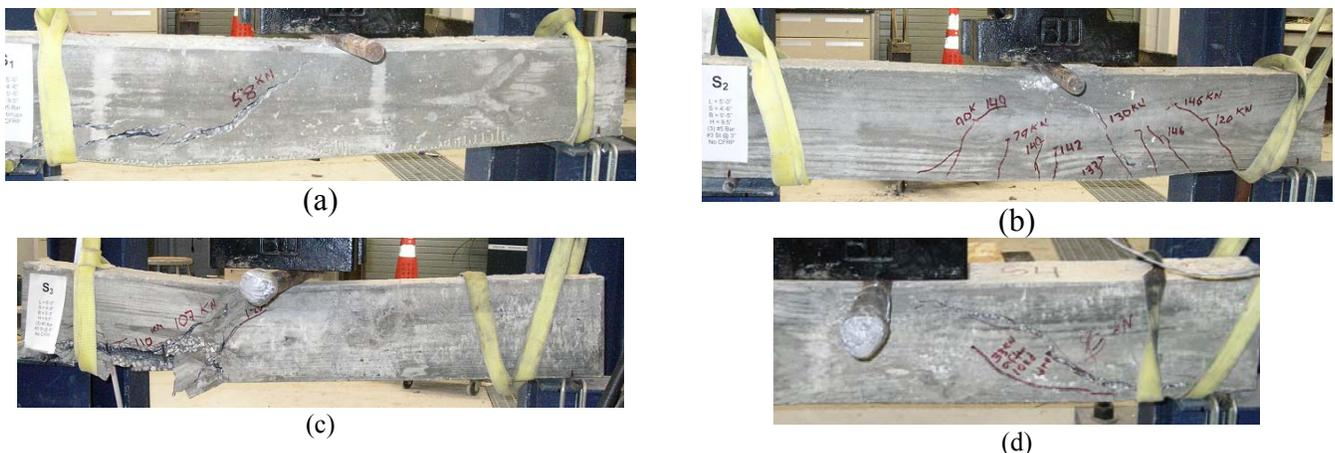
**Fig. 1 Testing of control beams (a) S1, (b) S2, (c) S3, and (d) S4**
