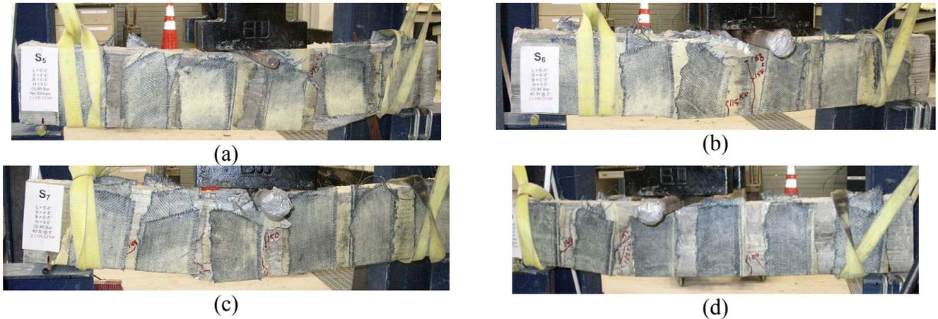
**Fig. 2 Testing of shear strengthened beams (a) S5, (b) S6, (c) S7, and (d) S8**
